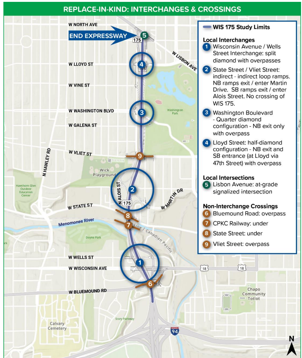
Figure 29 – WIS 175 Interchanges and Crossings – Replace-In-Kind
