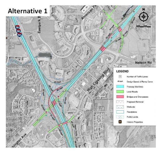
**Alternative 1** provides freeflow system ramps for the US 151/Interstate connection. The connection to East Washington Avenue is served with a more traditional diamond interchange with signalized ramp terminals (as opposed to the current cloverleaf interchange). It also relocates the American Center main entrance from American Parkway to American Family Drive.
