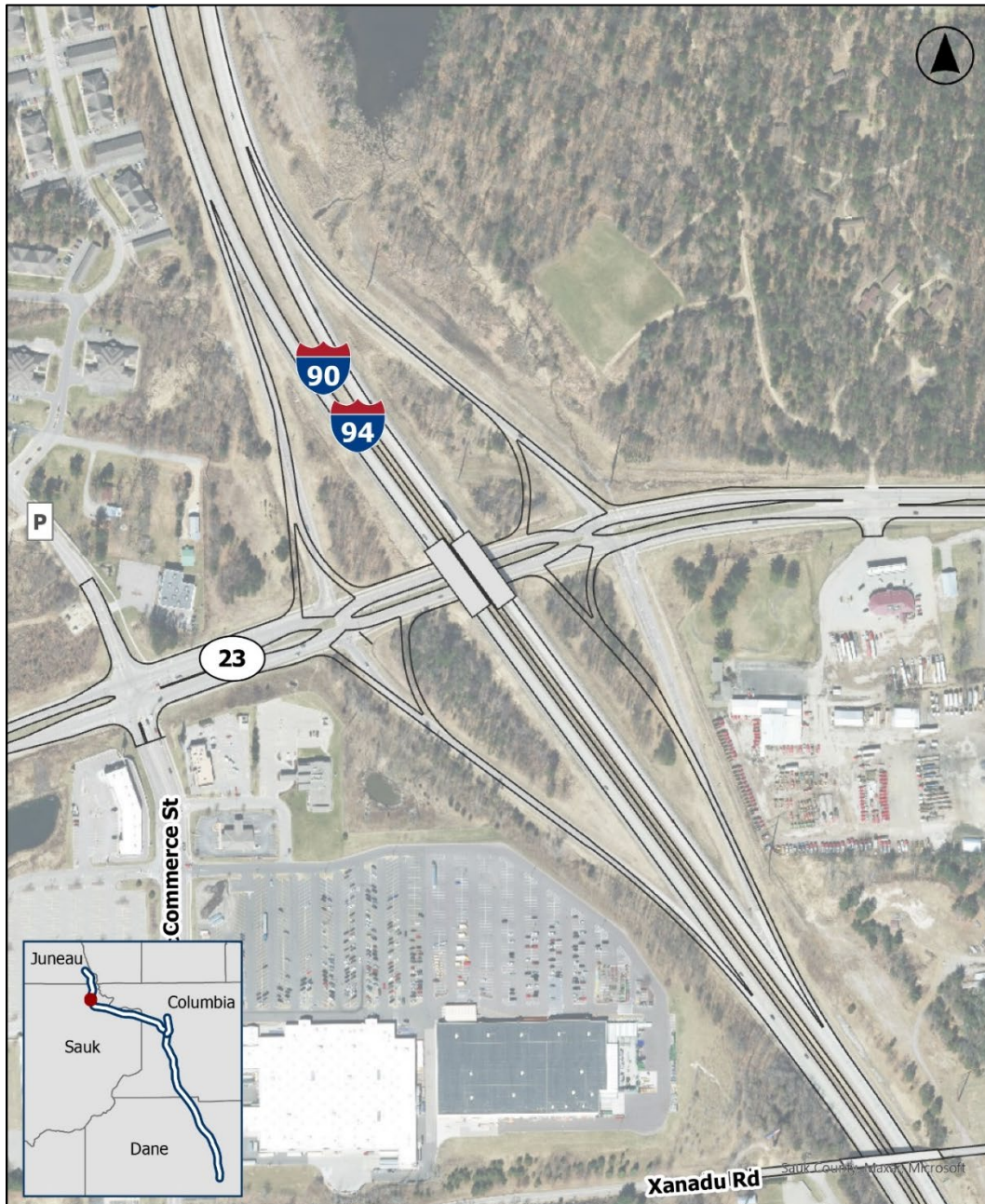
Figure 3-40: WIS 23 – Diverging Diamond Interchange
