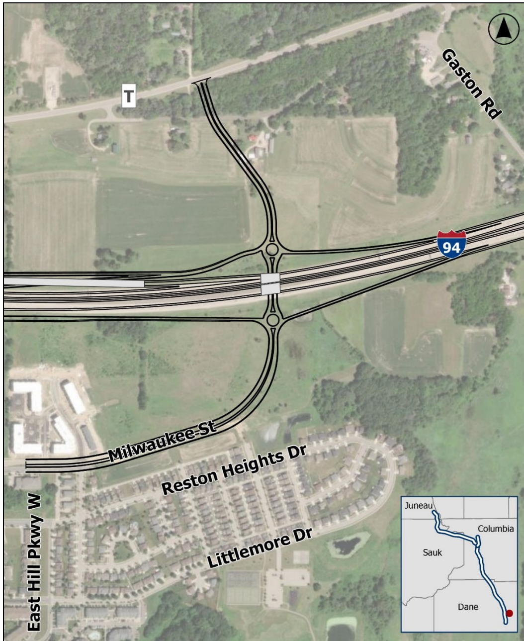
Figure 3-11: Milwaukee Street - Diamond Interchange
