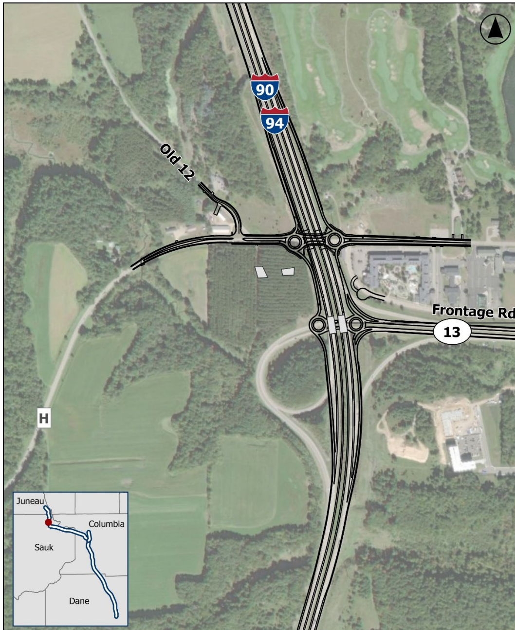
Figure 3-42: WIS 13 – Split Diamond Interchange
