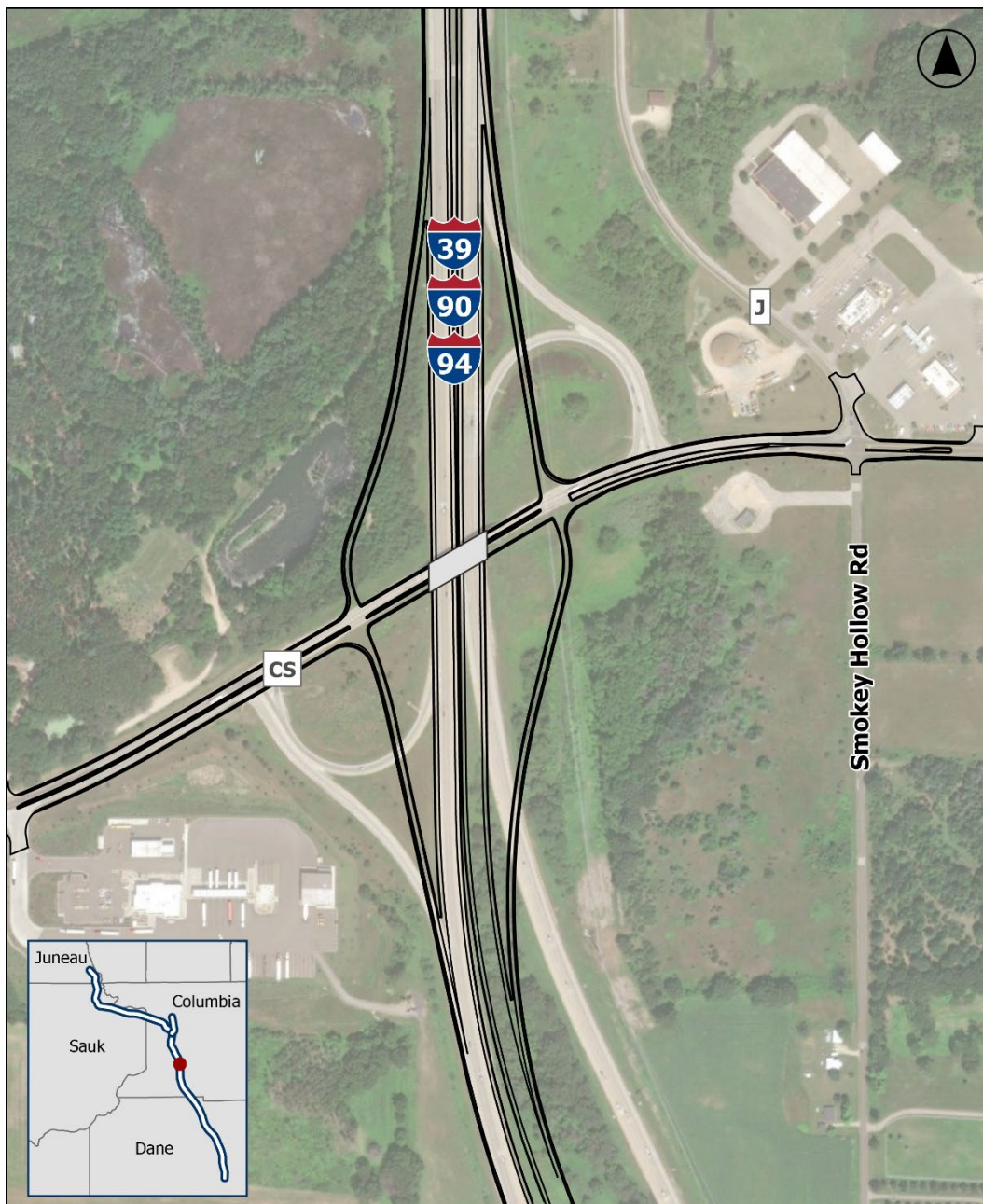
Figure 3-29: County CS – Diamond Interchange
