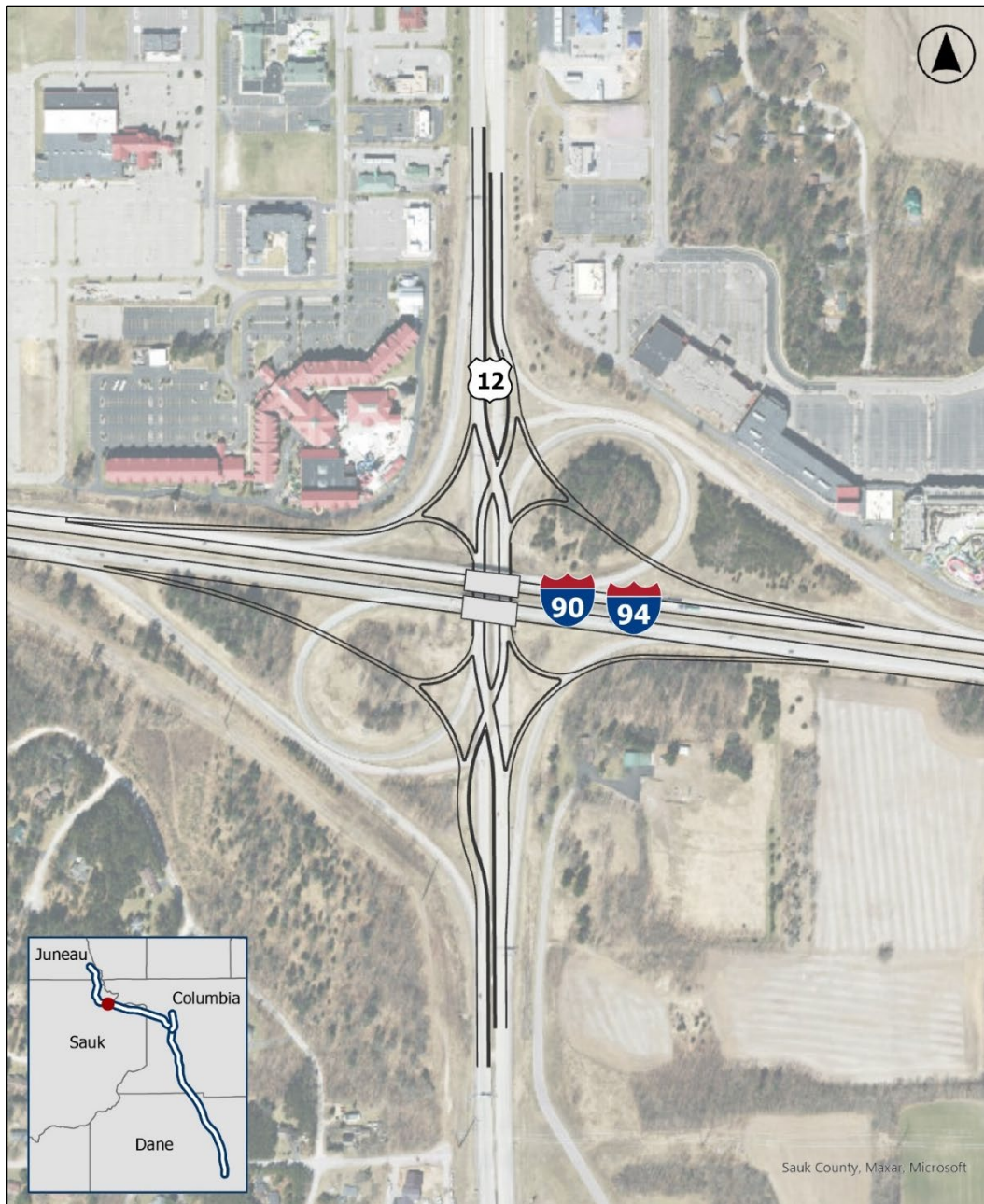
Figure 3-36: US 12 – Diverging Diamond Interchange
