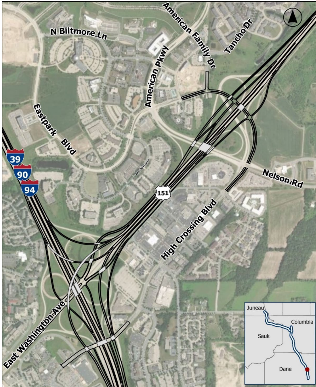
Figure 3-12: US 151/High Crossing Boulevard – Directional Interchange
