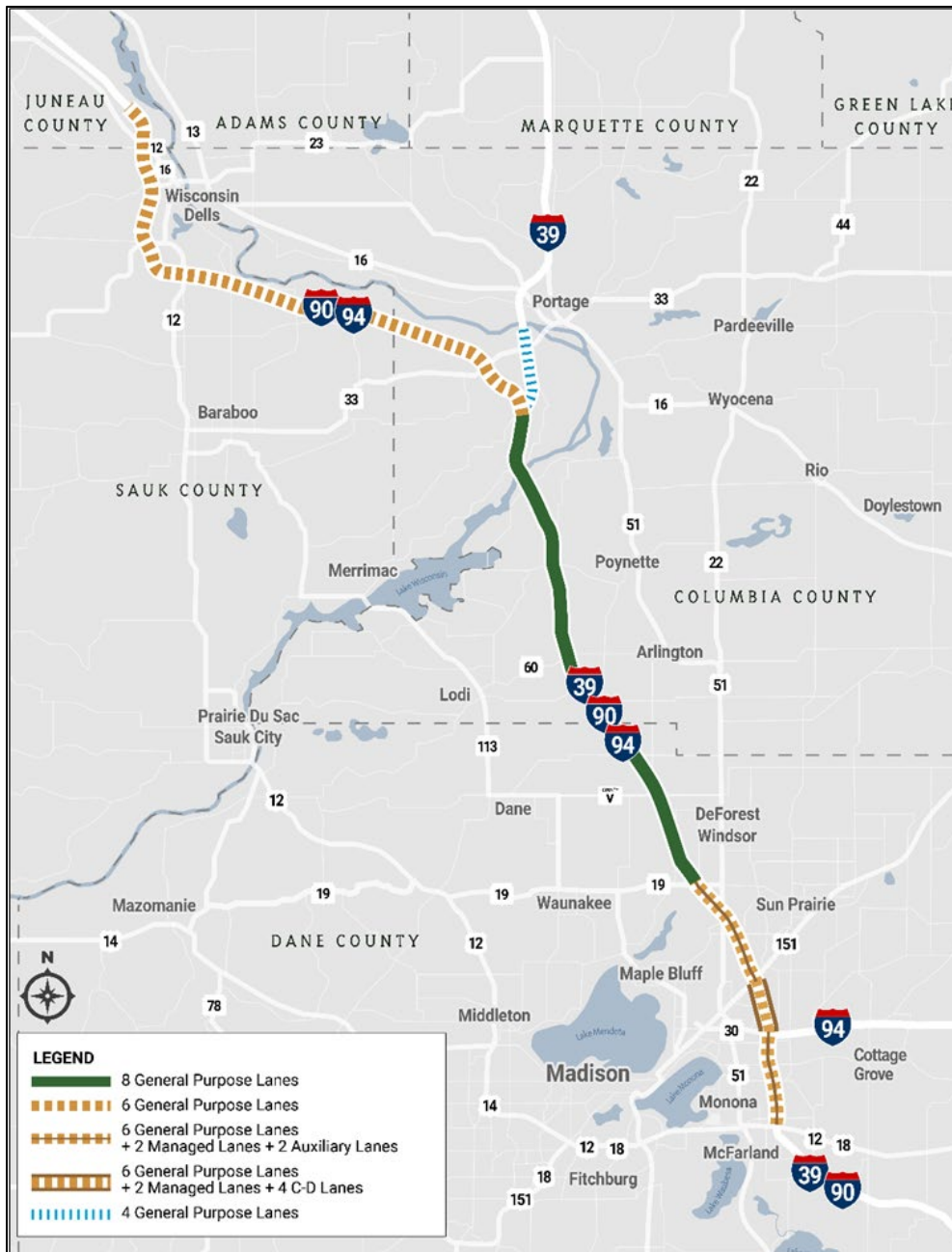
Figure 3-5: Modernization Hybrid; General-Purpose Lanes
