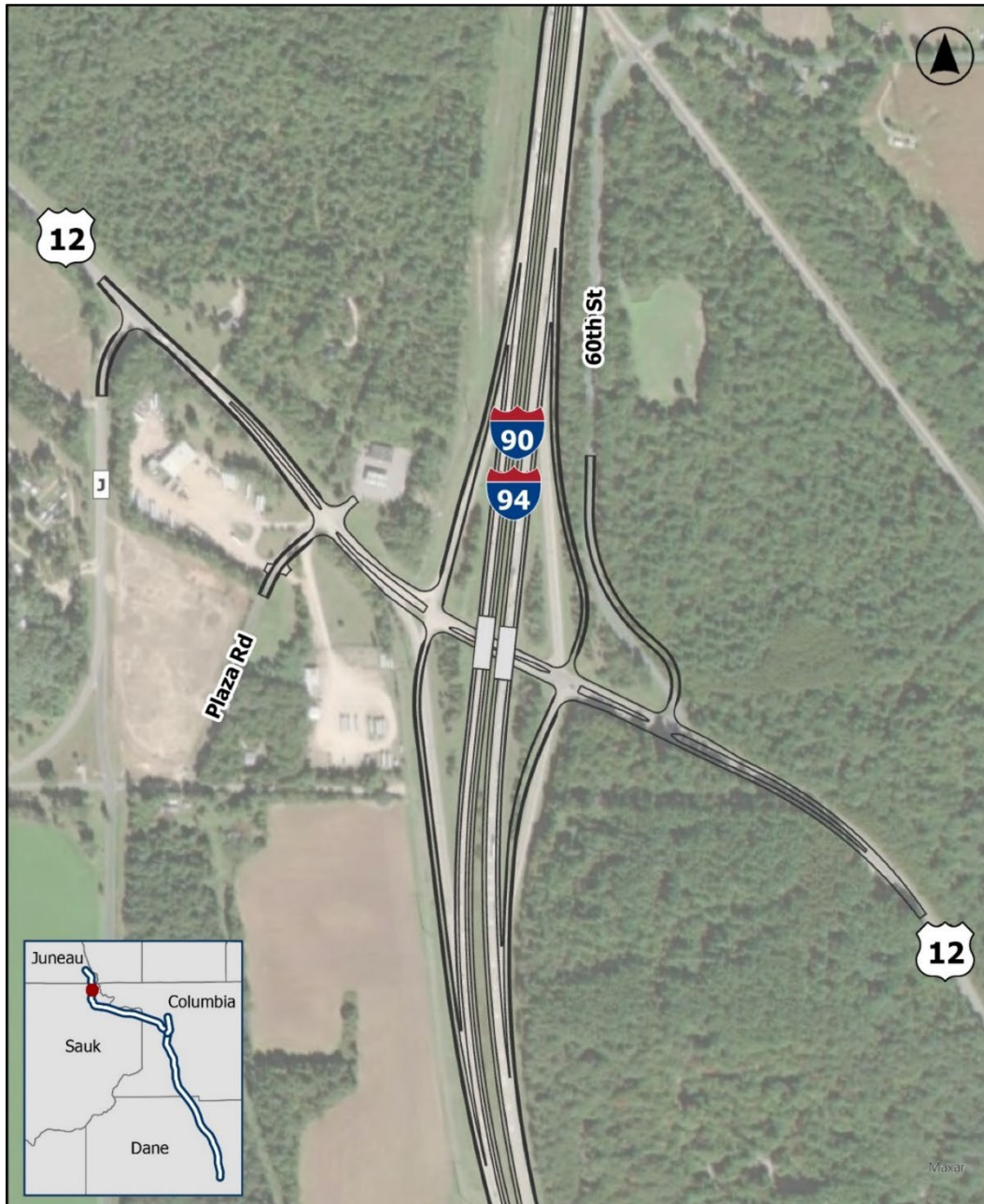
Figure 3-44: US 12/WIS 16 – Diamond Interchange
