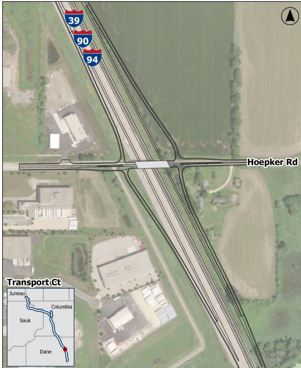
Figure 3-18: Hoepker Road – Shifted Diamond Interchange
