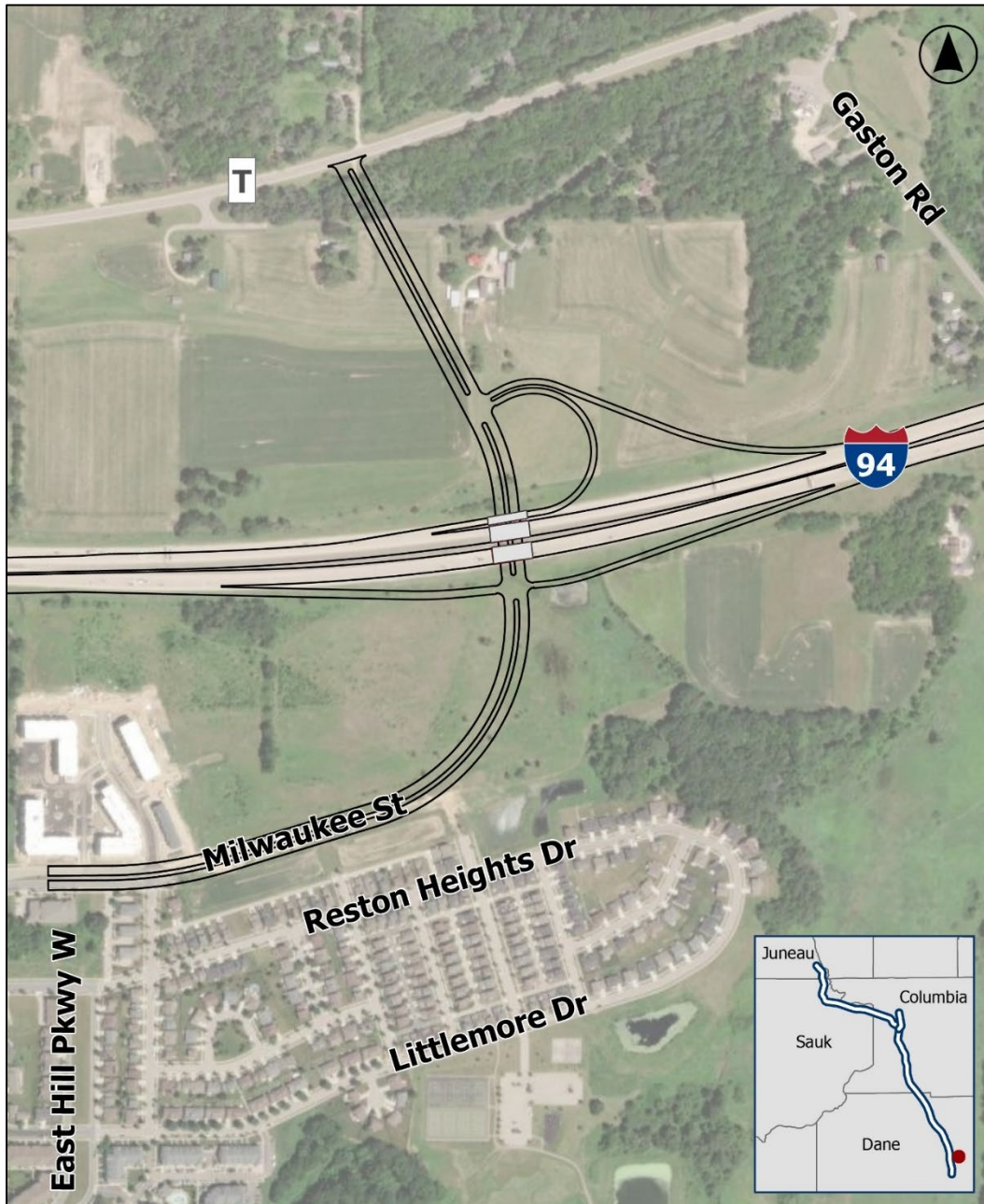
Figure 3-10: Milwaukee Street – Partial Cloverleaf Interchange
