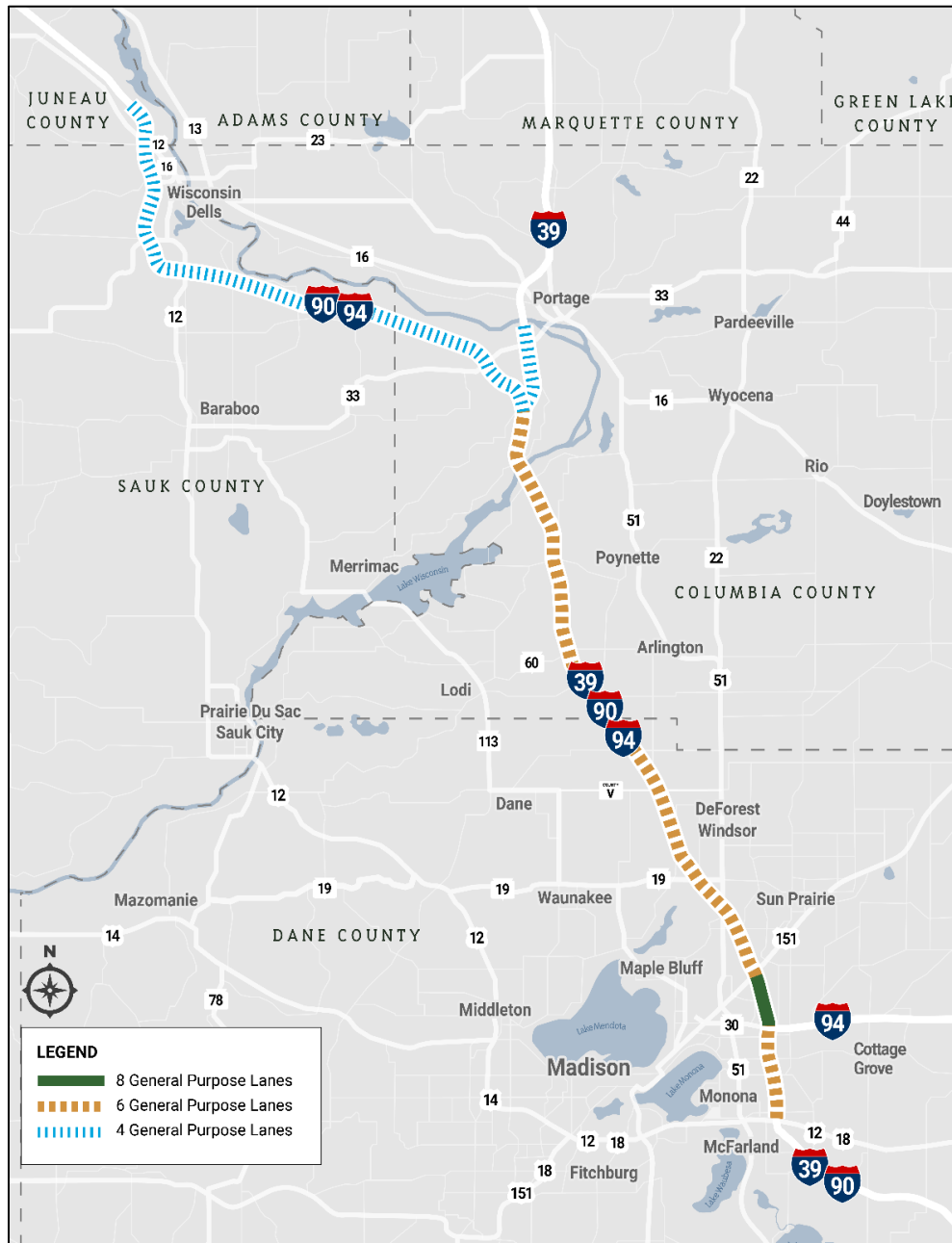
Figure 3-3: Modernization of Existing Travel Lanes; General-Purpose Lanes
