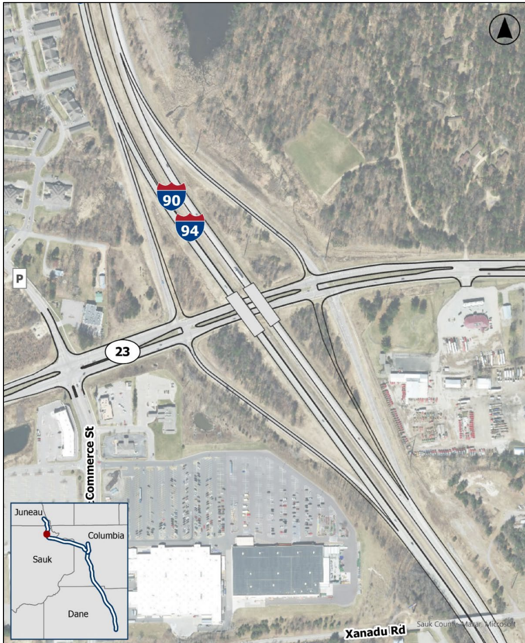
Figure 3-39: WIS 23 – Diamond Interchange
