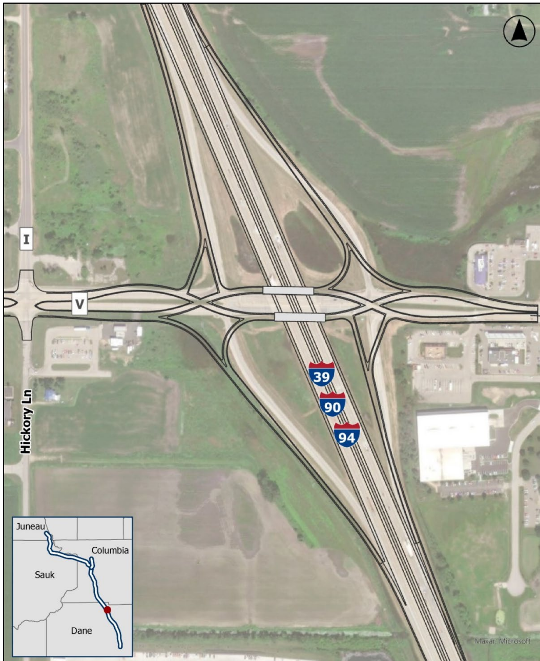
Figure 3-27: County V – Diverging Diamond Interchange
