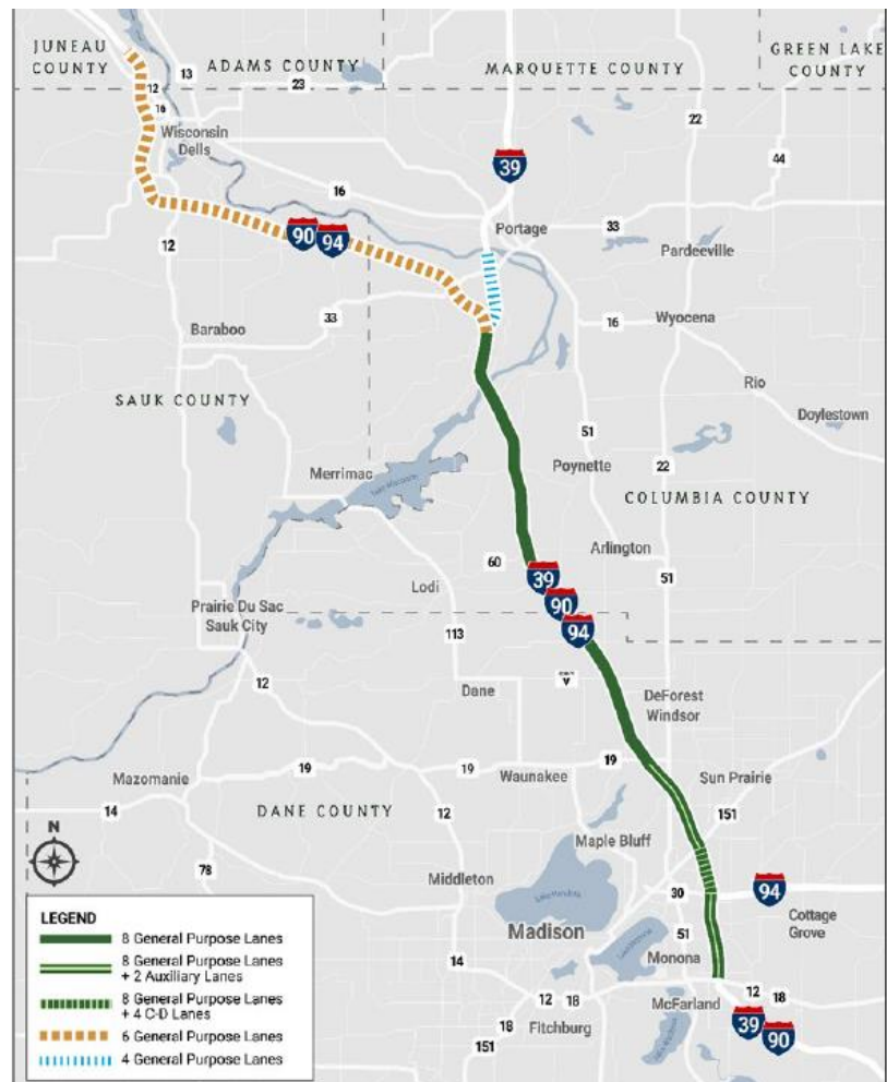
Figure 2: Modernization of Existing Travel Lane Alternative with Number of General-Purpose Lanes (WisDOT 2024b)
