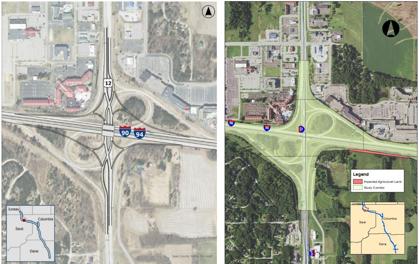
Figure 20: US 12 Diverging Diamond Alternative Design (WisDOT 2024c); Figure 21: Proposed Agricultural Land Acquired by US 12 Diverging Diamond Alternative Design, Credit: DATCP
