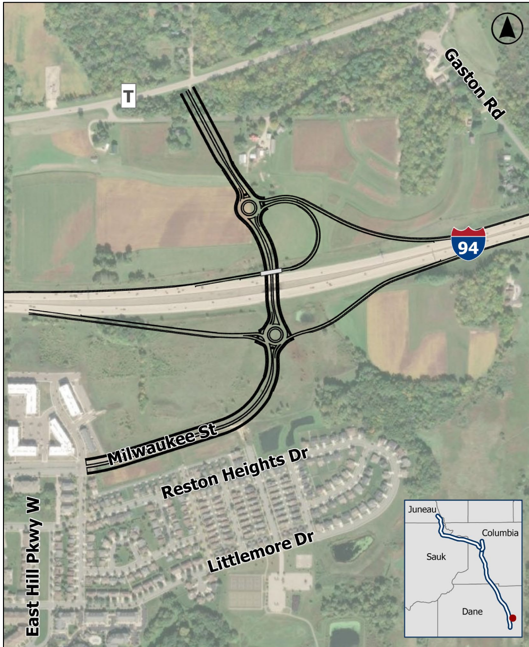
Figure 2-9: Milwaukee Street – Partial Cloverleaf Interchange
