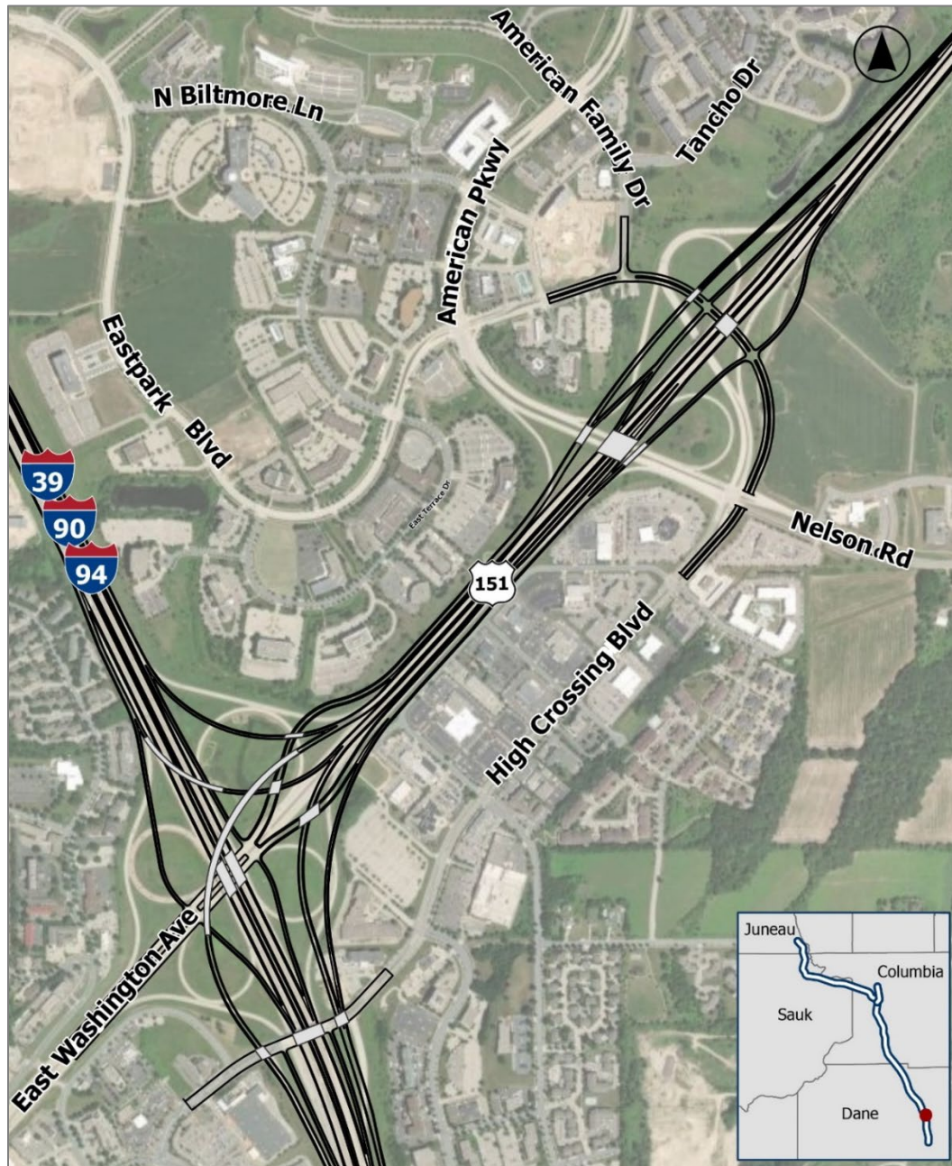
Figure 2-10: US 151/High Crossing Boulevard – Directional Interchange
