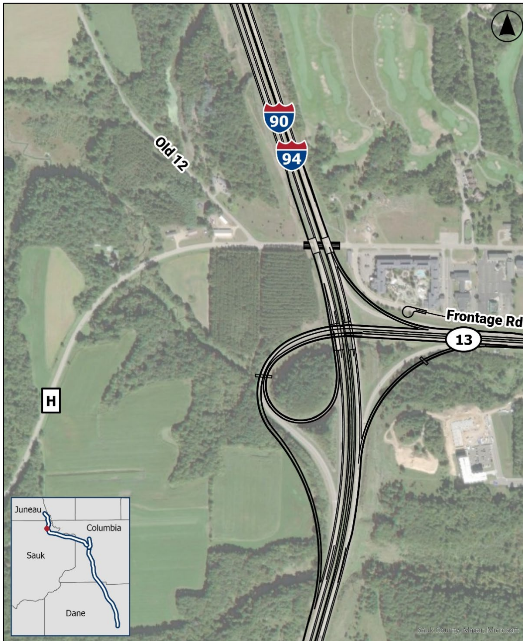
Figure 2-22: WIS 13 – Trumpet Interchange
