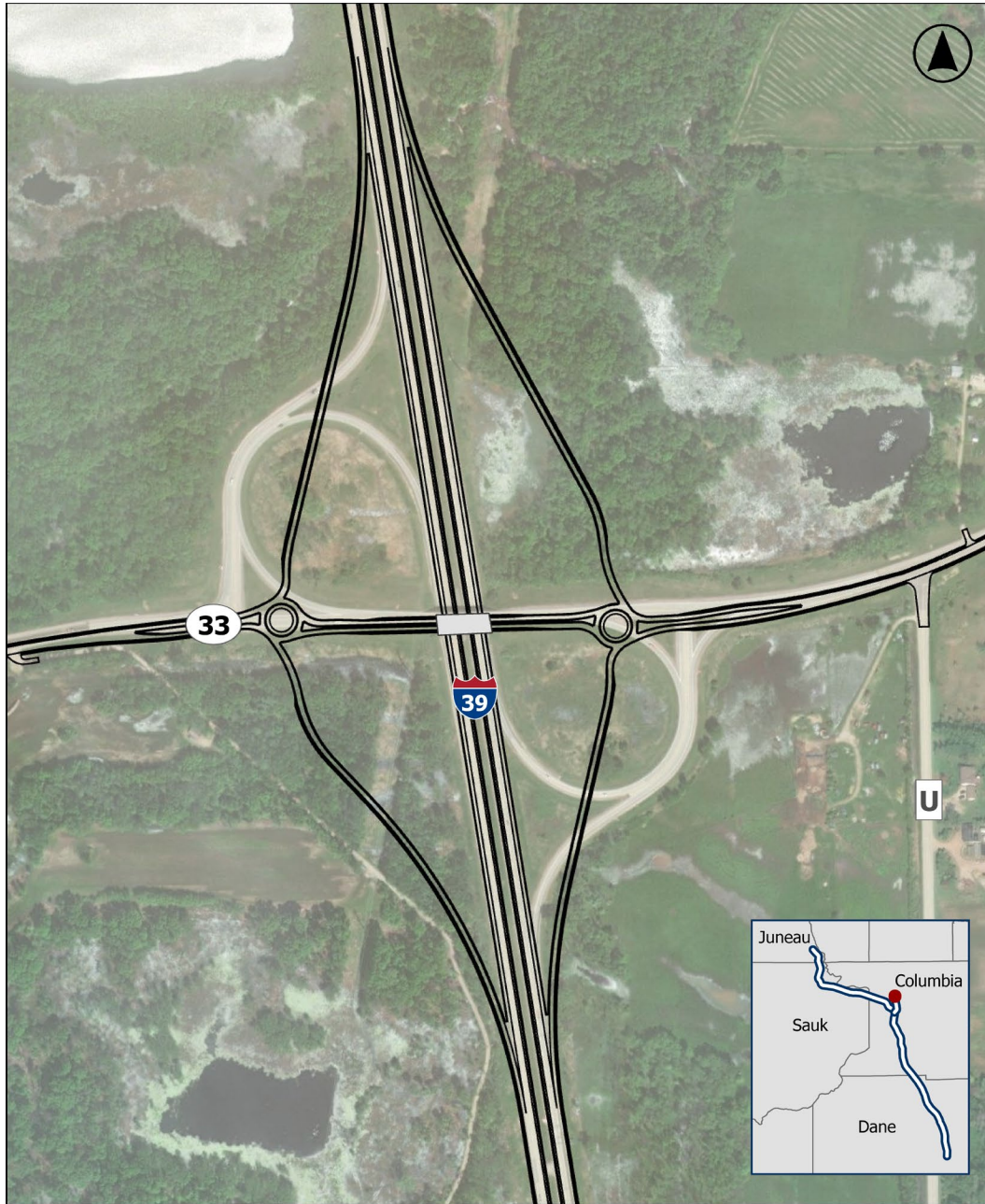
Figure 2-17: WIS 33 at I-39 – Diamond Interchange
