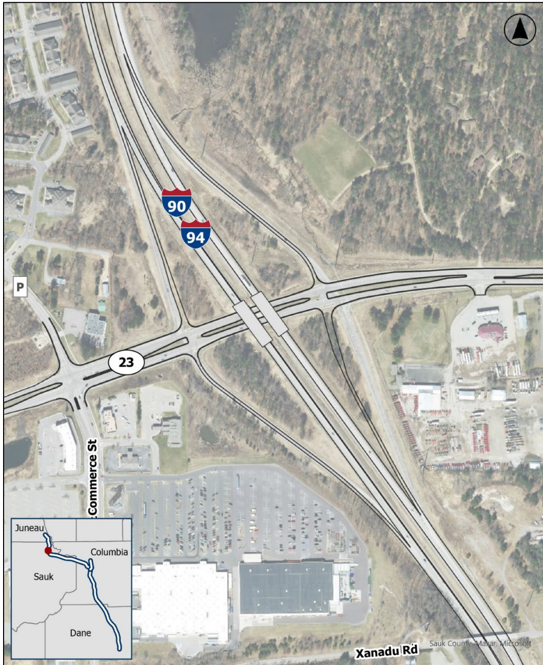
Figure 2-20: WIS 23 – Diamond Interchange
