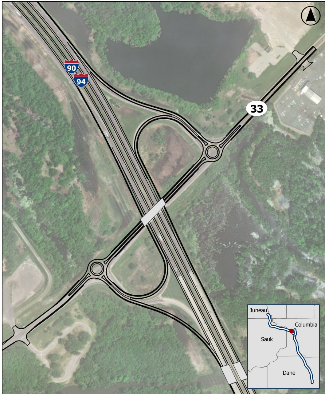
Figure 2-18: WIS 33 at I-90/94 – Partial Cloverleaf Interchange
