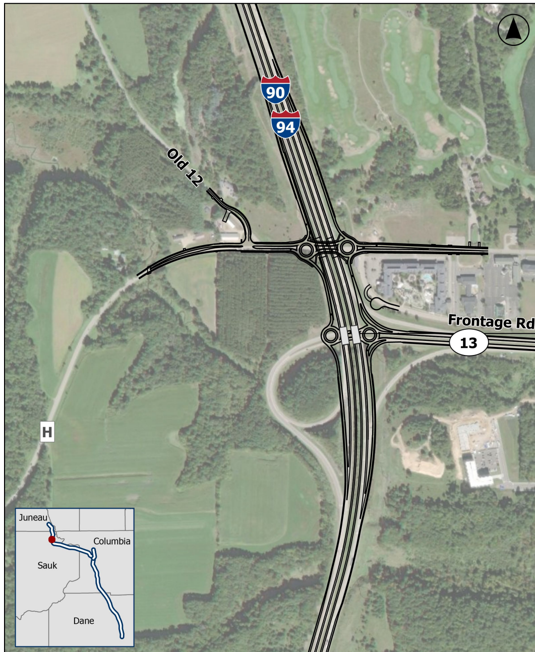
Figure 2-21: WIS 13 – Split Diamond Interchange
