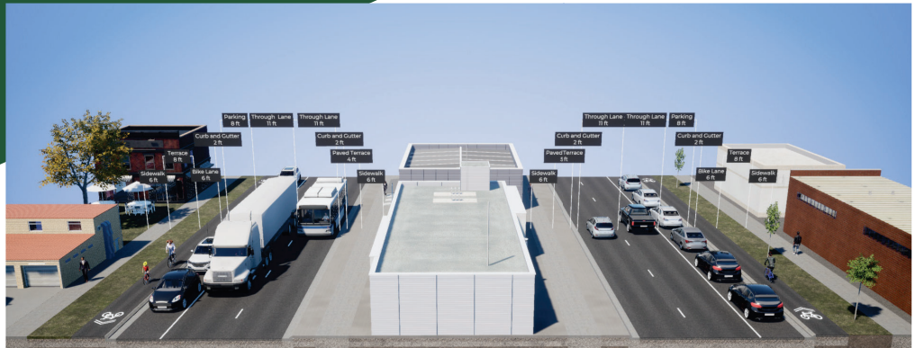
Lane Reconfiguration (Parking-Protected Bike Lanes) Total Width (Curb to Curb): 34 ft (SB US 14/61), 34 ft (NB US 14/61)
