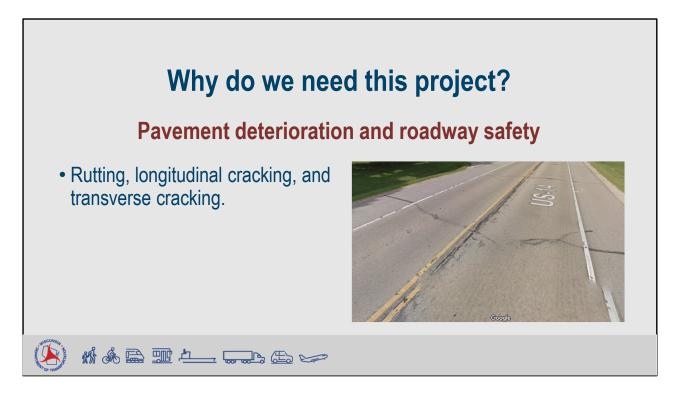
The project will improve the safety, comfort, and longevity of the highway. This section of US 14 is exhibiting pavement cracking and wheel path rutting. These pavement deficiencies are increasing both safety concerns and maintenance costs. If no action is taken, this roadway will continue to deteriorate, and maintenance costs will continue to increase.
