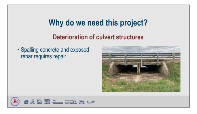
Within the project area, there is also a culvert and a cattle pass that are showing spalled concrete and exposed rebar which require repair to extend the life of the structures.
