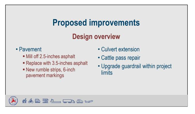
The proposed improvements include resurfacing of US 14, installation of centerline and shoulder rumble strips, upgrading the guardrail, and updating the pavement markings. Structure repairs will occur to the cattle pass west of the Mazomanie village limits along with repairs and culvert extensions to the box culvert just west of Arena village limits.
