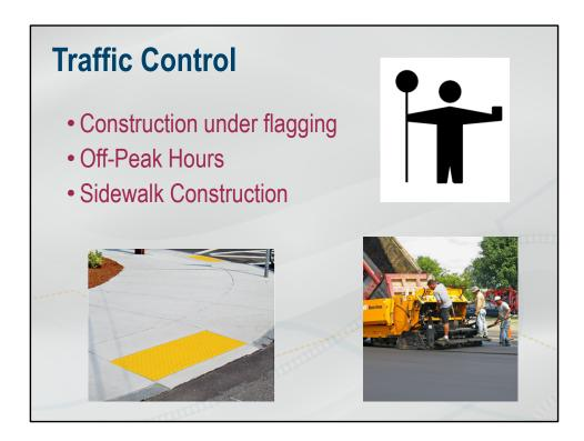
We are anticipating that US 51 will remain open during construction. During milling and paving operations, flagging will occur to ensure traffic is able to safely move through the work zone. Milling and paving will take place during off-peak hours to minimize the impact to traffic.
