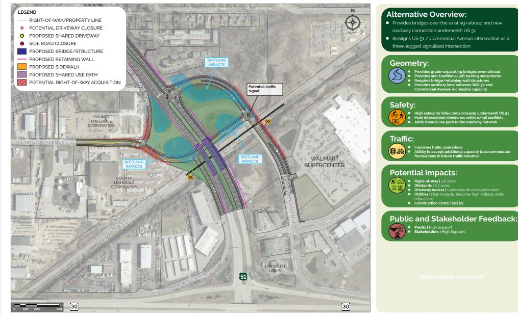
Grade separated intersection, bridges required for this alternative. Railroad south of intersection is being investigated for potential high-speed rail. The design presented in this exhibit is preliminary and specific details may be refined in final design.
