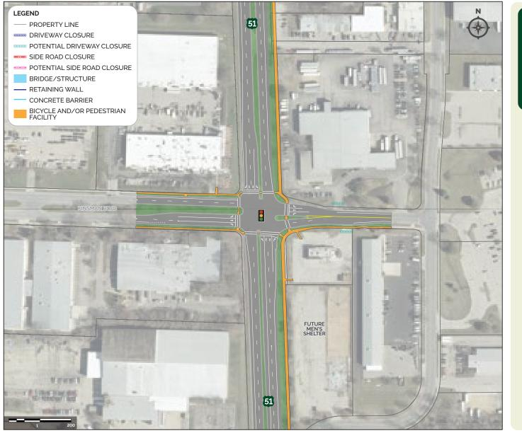
At-grade intersection, no bridges required for this concept alternative. Number of lanes, length of turn lanes, and other geometric elements are conceptual and may not reflect final design.
