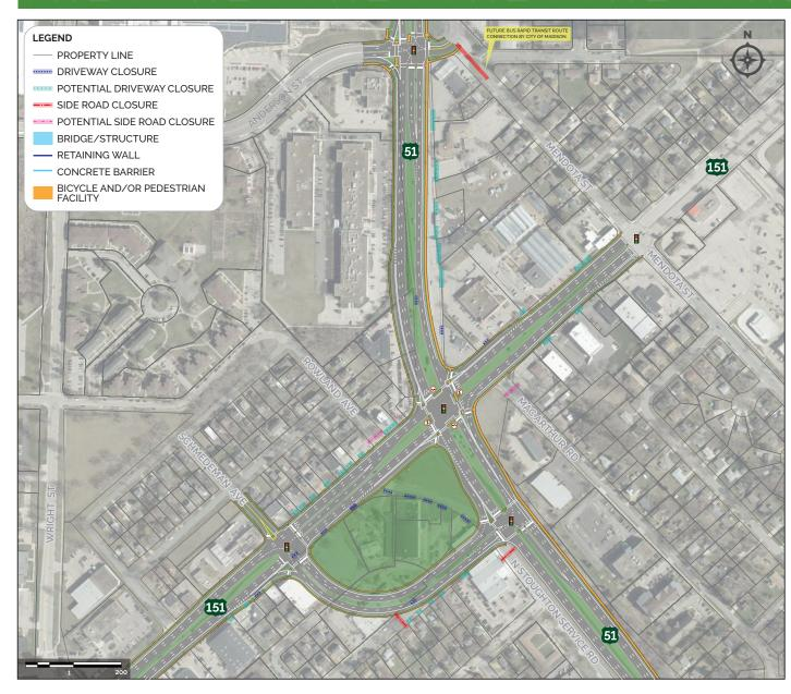
At-grade intersection, no bridges required for this concept alternative. Number of lanes, length of turn lanes, and other geometric elements are conceptual and may not reflect final design.
