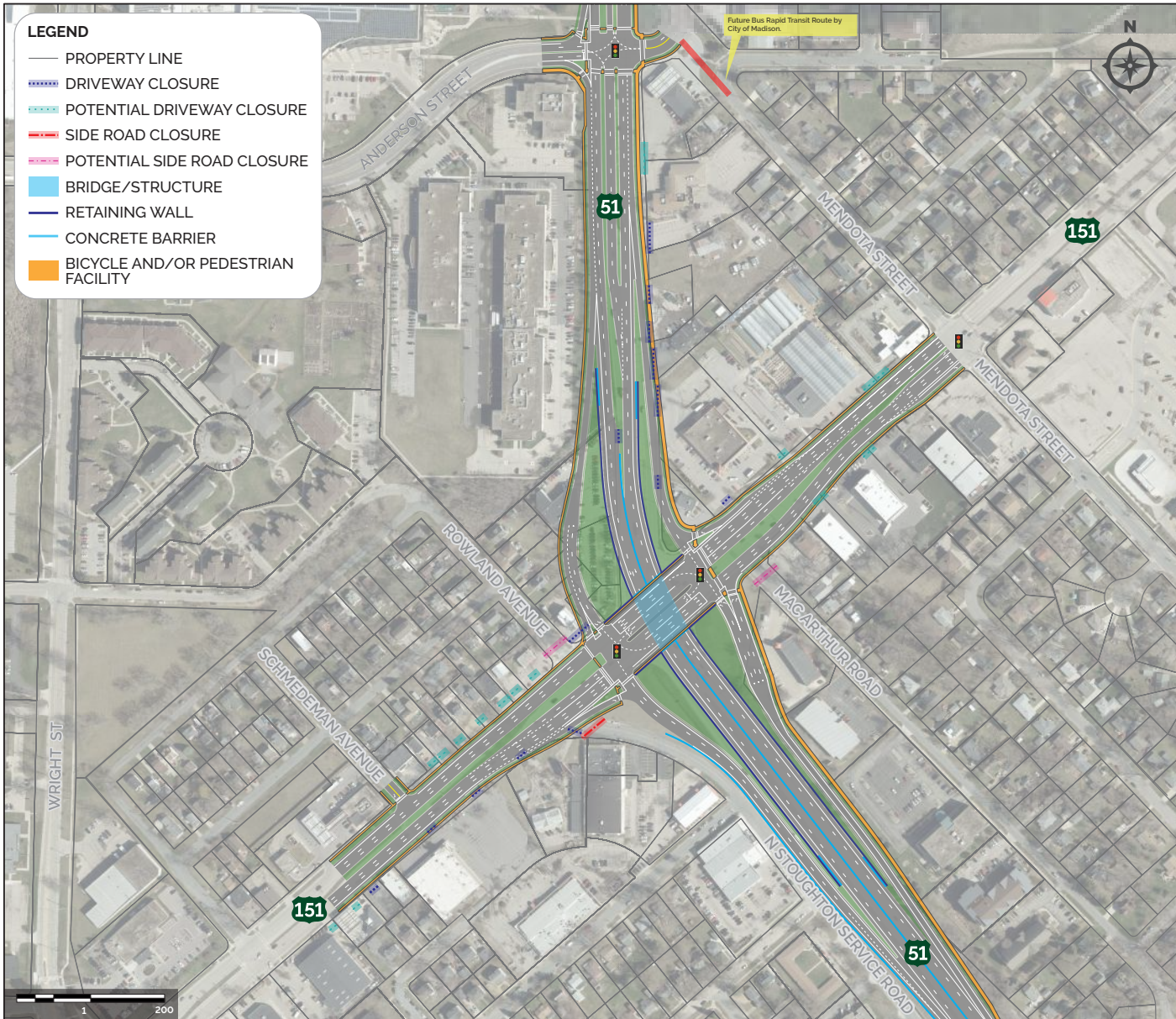
Grade separated intersection, recessed roadway introduced along US 51 for this concept alternative. Number of lanes, length of turn lanes, and other geometric elements are conceptual and may not reflect final design.
