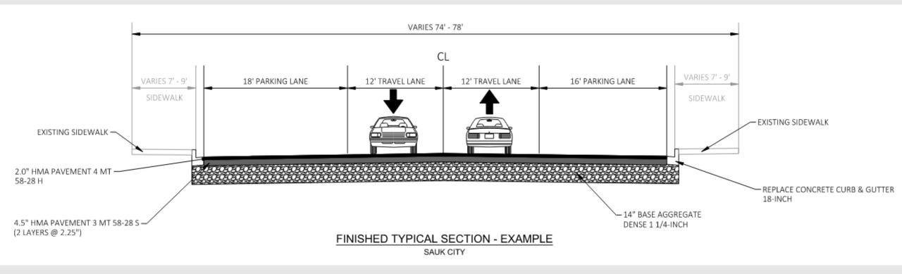
Proposed pavement structure: 14" base aggregates, 6.5" asphalt
