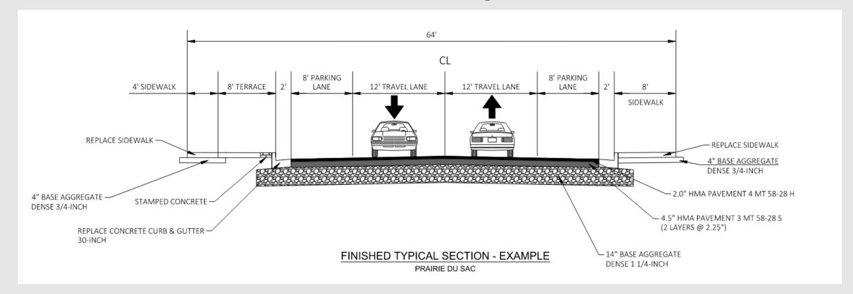
Proposed pavement structure: 14" base aggregates, 6.5" asphalt
