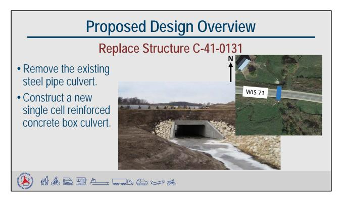
Remove the existing 9-ft wide by 100 ft long steel sectional pipe culvert, C-41-0131, and replace it with a new 12.5-ft wide by 112-ft long single-cell reinforced concrete box culvert.
