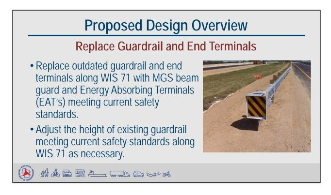
The existing outdated end terminals and guardrail will be replaced with Midwest Guardrail System (MGS) guardrail and Energy Absorbing Terminals (EAT's) meeting current safety standards at structures B-41-280, B-41-329, B-41-113, B-41-114, B-41-133 and 4 other locations along WIS 71.
