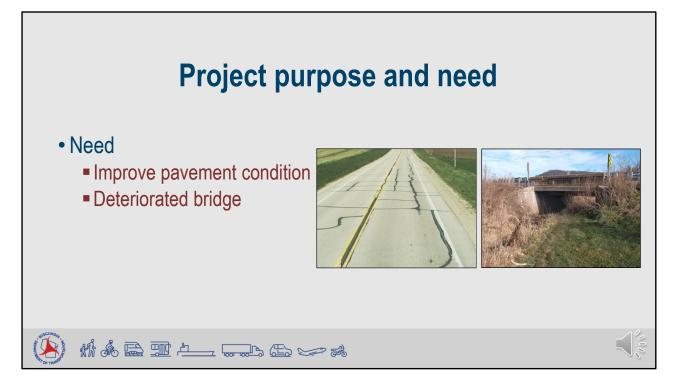
The existing pavement on WIS 80 is experiencing longitudinal and transverse cracking in the wheel paths of vehicles and along the centerline of the roadway. This results in a decreased ride quality and increased maintenance expenditures. The existing bridge 500 feet north of the Dry Dog Road intersection was built in 1930 and received an asphalt overlay in 2014. The bridge has met/exceeded its service life and requires a replacement with a new bridge structure that meets Department's standards.
