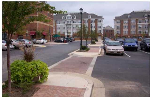
Surface parking lots at King Farm in Rockville, Maryland, incorporate brick pavers to distinguish pedestrian walkways from the parking area.
