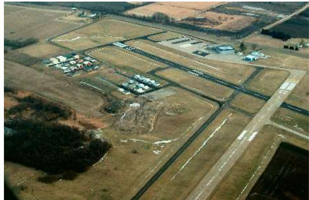
The primary runway (08/26) is 5,060 feet long by 100 feet wide. Lighting aids on this runway include a Medium Intensity Approach Light System with sequenced flashing lights (MALSF), Precision Approach Path Indicators (PAPI), and Medium Intensity Runway Lights (MIRL).
