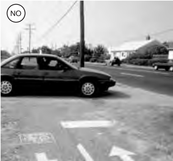
Figure 4-3: A path next to an arterial street. Bicyclists on the path are required to stop at each minor cross street.
