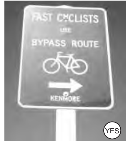
Figure 4-18: A green information sign directing faster bicyclists to nearby roadway.
