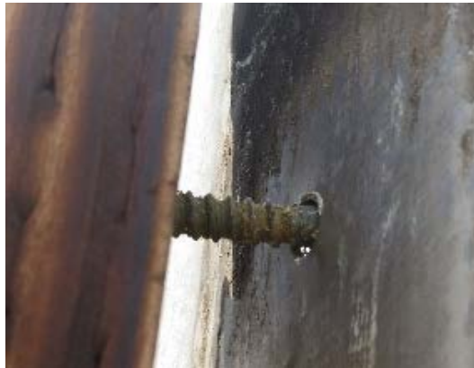
Figure 2: Lag screw after 2 years
