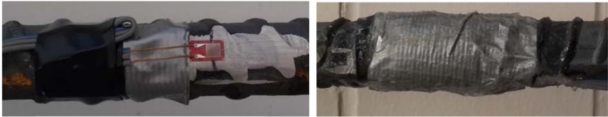
Figure 5-7. Strain Gauge on re-bar (left), and after water-proof (right).
