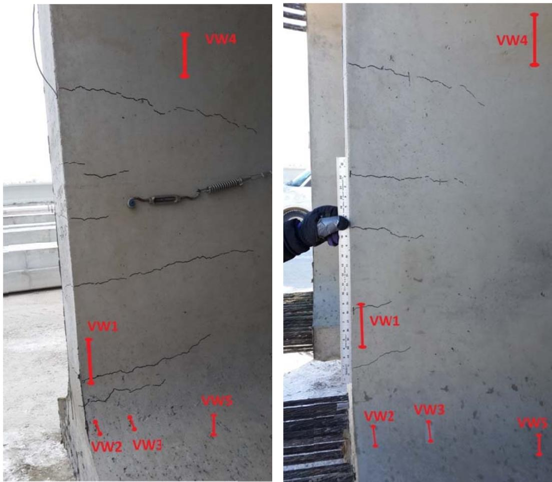
Figure 5-24. Location of vibrating wire gauges in bonded (left) and de-bonded (right) girders.
