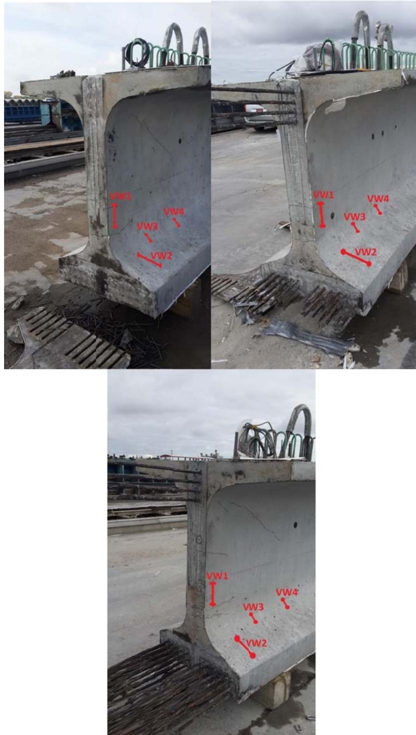
Figure 6-25. The location of vibrating wire gauges in bonded (top left), 38% debonded (top right), and the girder that is debonded 8 in. from end (bottom).
