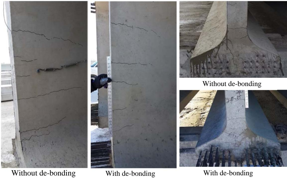
Figure 5-25. Cracks at the ends of bonded and de-bonded girders.
