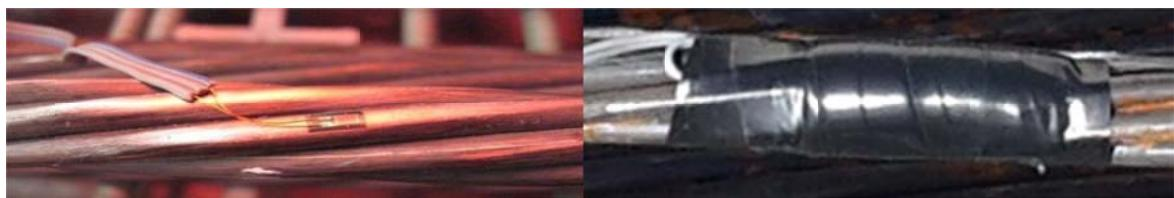
Figure 6-8. At the left, strain gauge on strand and at the right, the gauge after protection.
