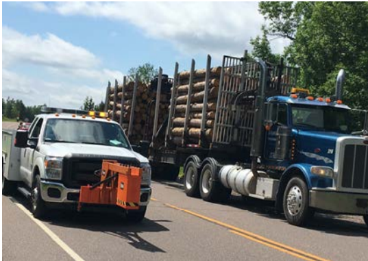
(e) The 2 GHz GPR antenna
