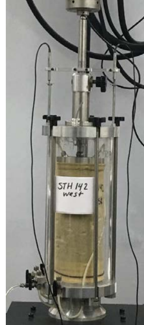
(b) 6 in diameter triaxial cell
