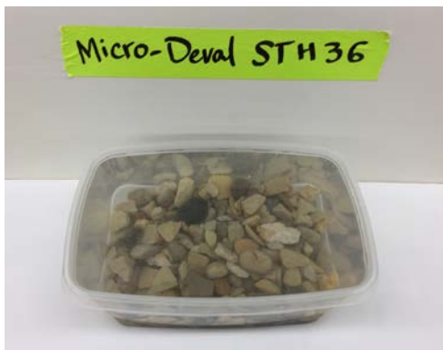
(c) Soaking Micro-Deval test specimen
