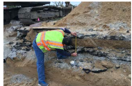
(i) Pavement layer thickness at STH 36
