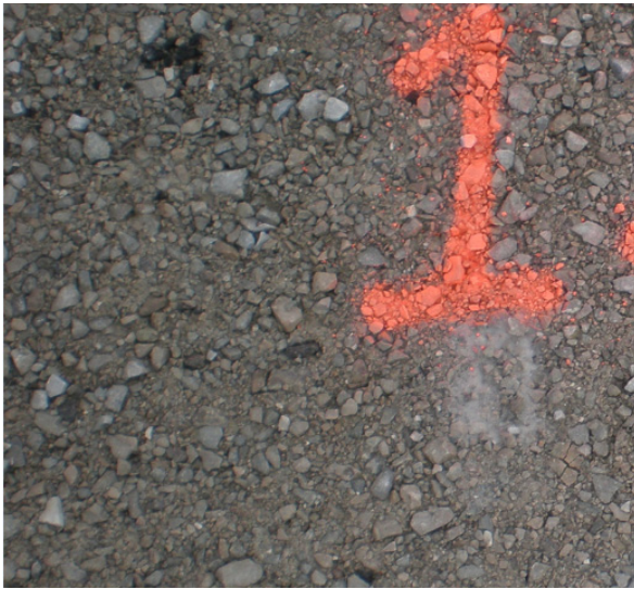
CTH JJ – Appleton: Crushed aggregate of sedimentary origin (carbonates: dolostone/limestone). Angular and semi-angular particles with rough surface texture.
