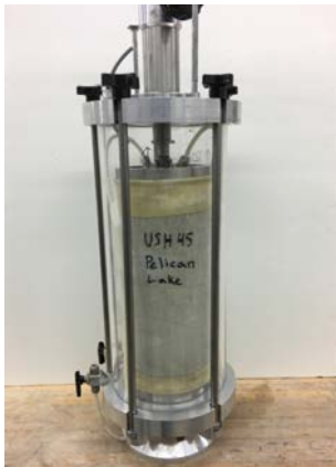
(g) Specimen in triaxial cell
