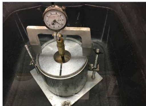
(b) Soaking CBR test specimen
