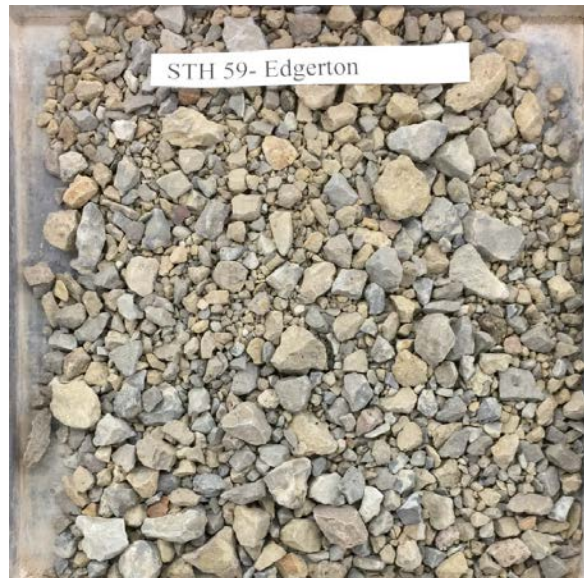
STH 59 – Edgerton: Crushed aggregate of sedimentary origin (carbonates: dolostone/limestone). Angular and semi-angular particles with rough surface texture.
