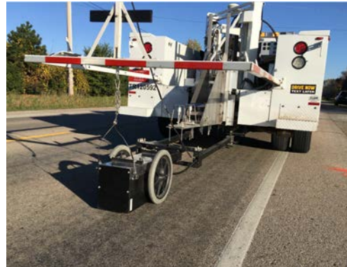
(f) The 900 MHz GPR antenna
