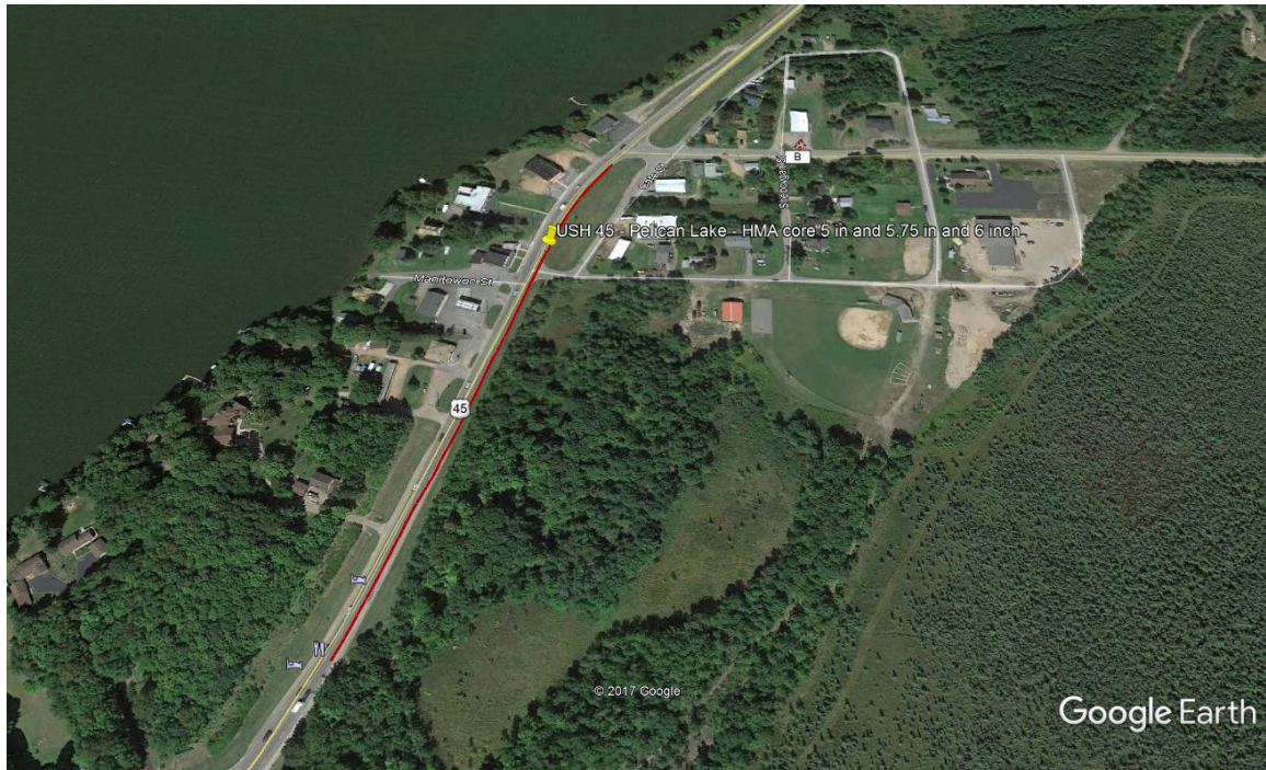
(a) Track of the GPR testing at USH 45 Pelican Lake: outside wheel path of the northbound lane (bottom to top in the picture)
