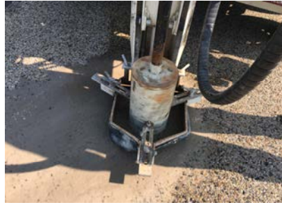
(b) 8-inch coring barrel
