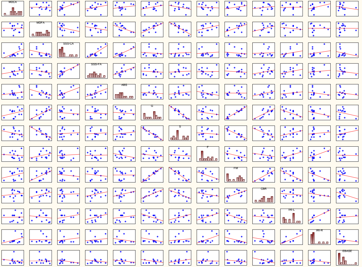
Figure 6.1: Plots and histograms of the individual properties and parameters of the investigated base layer aggregates.
