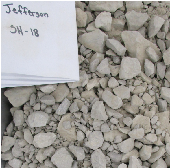
STH 18 – Jefferson: Crushed aggregate of sedimentary origin (carbonates: dolostone/limestone). Angular and semi-angular particles with rough surface texture.
