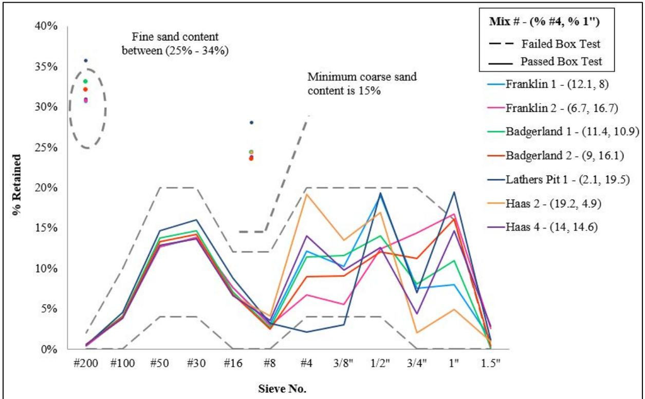
Figure 22: The Mixtures Plotted on the Tarantula Curve for the Mixtures from Part II. Dashed Lines Failed and Solid Lines Passed the Box Test.
