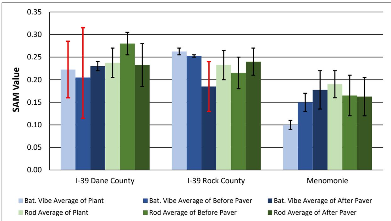
Figure 68: Consolidation method comparison for SAM values by location. Error bars represent the measured low and high SAM values.
