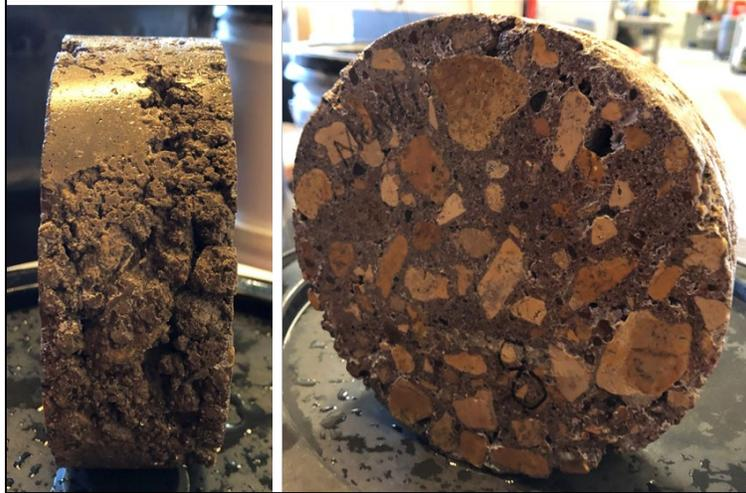
*Figure 77: Example of specimens from Menomonie with poor consolidation.*
