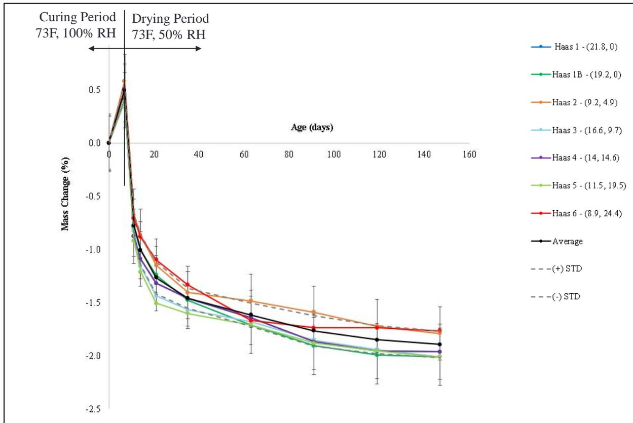
Figure 20: The Mass Change of the Mixtures on Each Day of Interest from Drying for the Testing in Part I.
