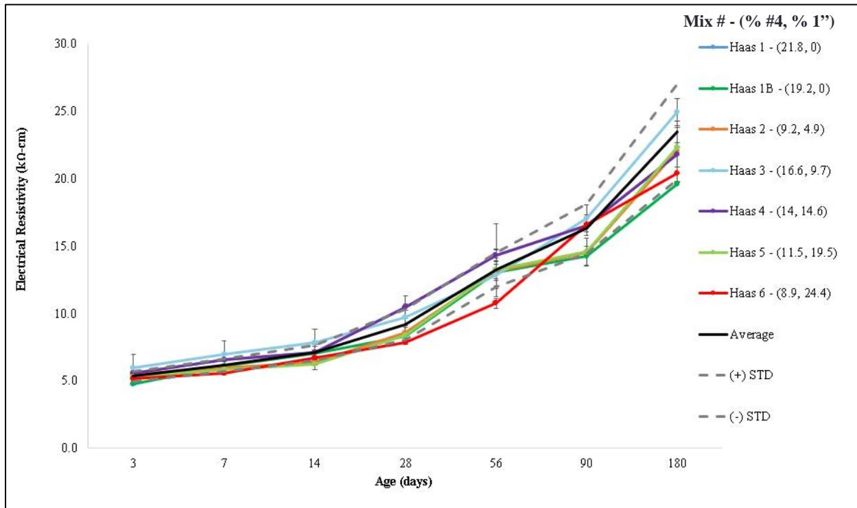
Figure 19: Average Apparent Surface Resistivity Measurements for Mixtures on Each Day of Interest.
