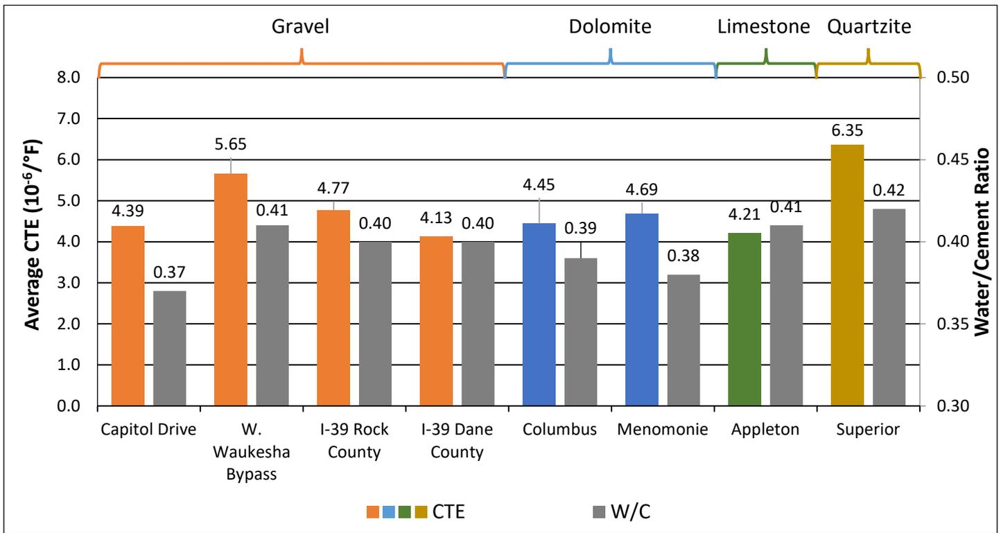
Figure 79: Average Coefficients of Thermal Expansion by w/c Ratio and Aggregate Type.
