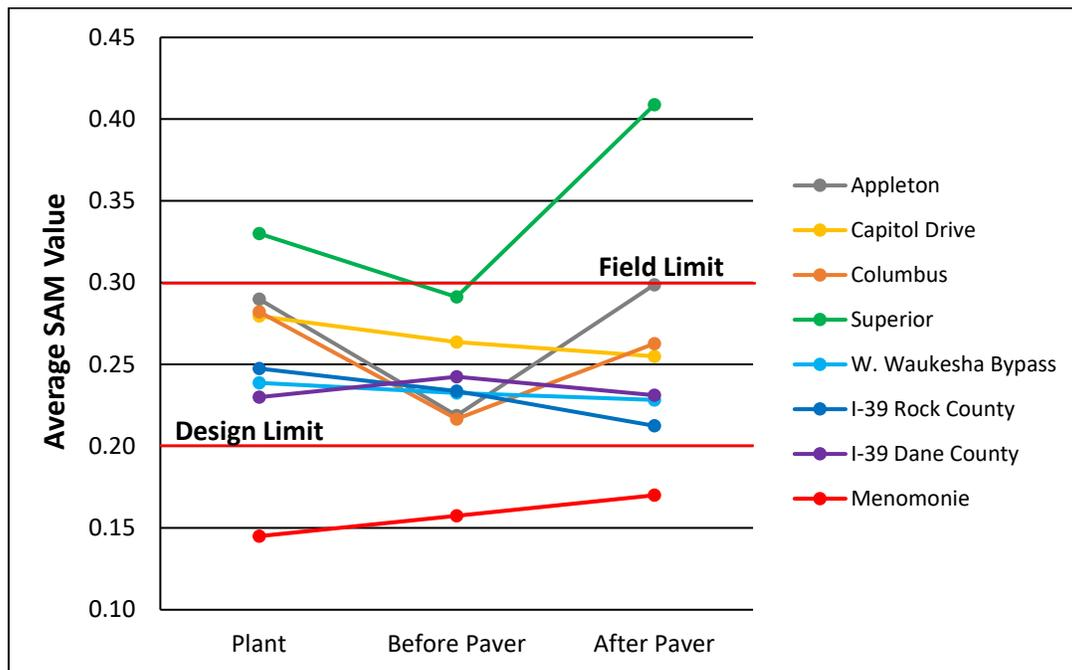
Figure 64: SAM value changes throughout production and placement from the plant to before and after the paver.
