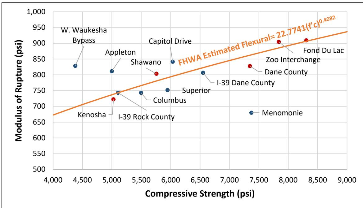
Figure 60: Phase I and II 28-Day Modulus of Rupture vs. Estimated Modulus of Rupture from Compressive Strength. Phase I Projects are Shown with Blue Dots and Phase II Projects are Shown with Red Dots.
