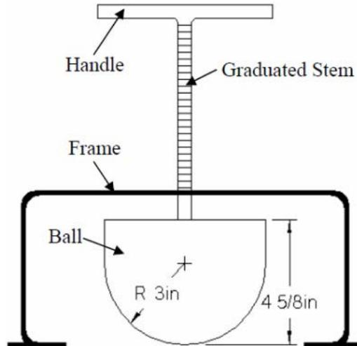
Figure 8: Schematic of the testing apparatus for ASTM C360-92. [31]
