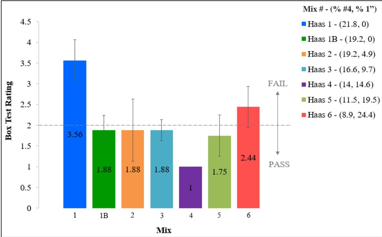
Figure 16: Average Box Test of all Mixtures.
