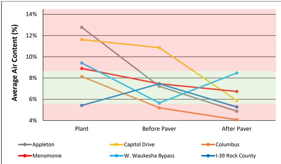
Figure 65: Hardened Air Contents from Samples taken from the Plant, Before, and After the Paver.
