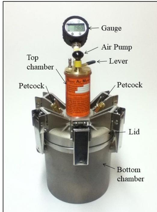
*Figure 6: SAM testing device.*
