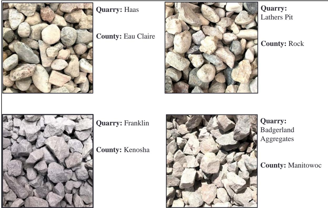
Figure 13: Pictures of the Coarse Aggregate Used in the Testing.
