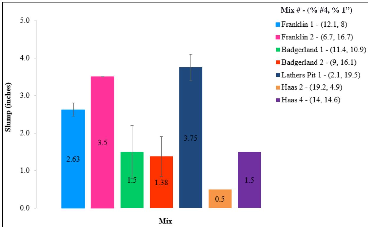
Figure 24: The Slump Test Results for the Mixtures in Part II.
