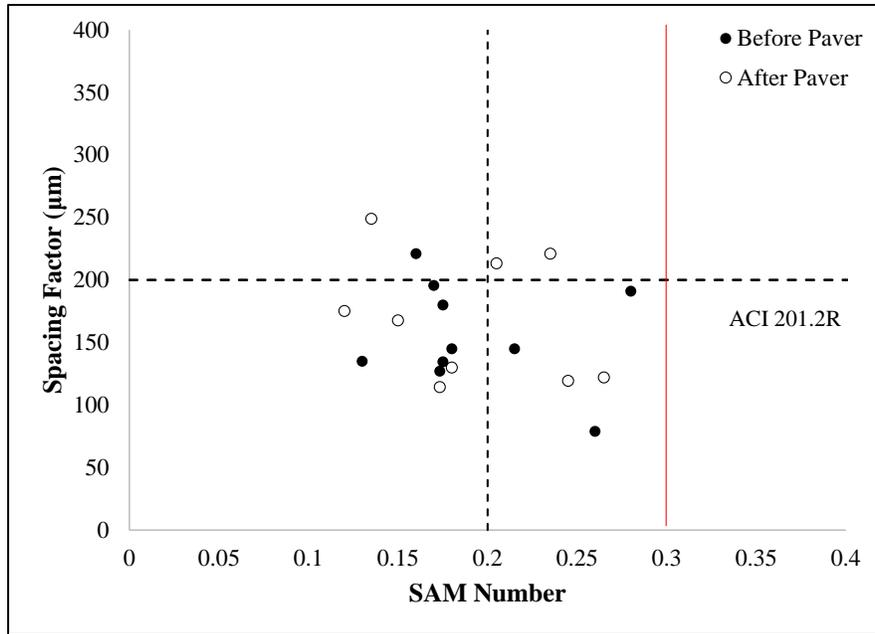
Figure 62: A comparison of the SAM Number and Spacing Factor.
