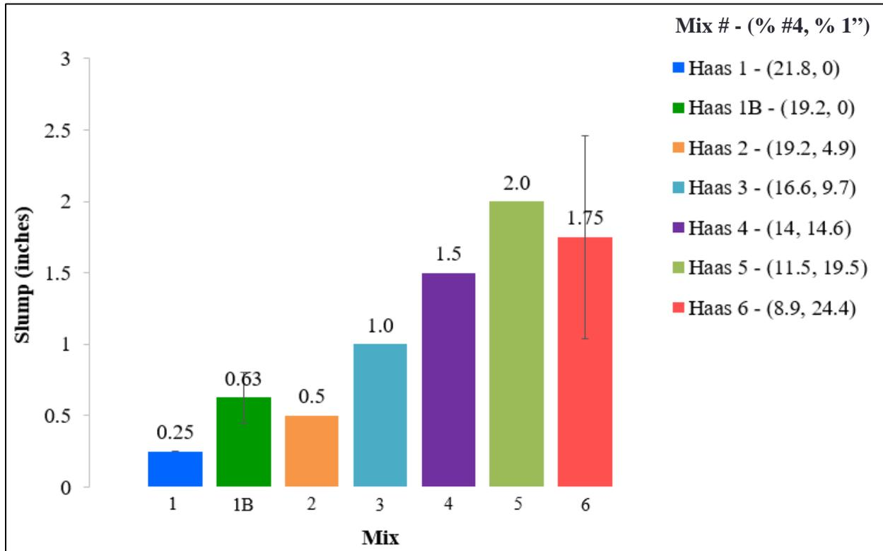
Figure 17: Average Slump Test Results for the Mixtures.
