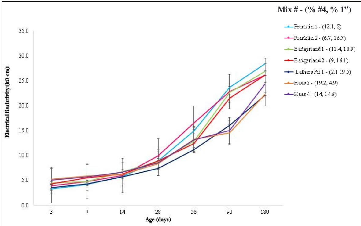
Figure 26: Average Apparent Surface Resistivity Measurements for Mixtures on Each Day of Interest.
