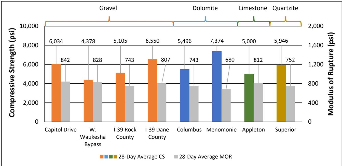
Figure 59: Phase I 28-Day Compressive Strength vs. 28-Day Modulus of Rupture.
