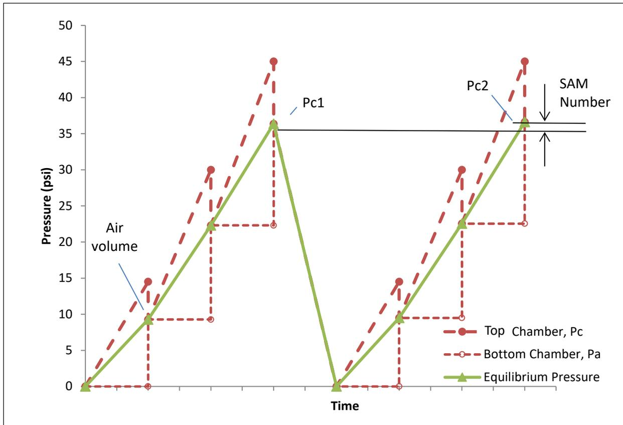
Figure 7: SAM pressure steps graphically shown for the top and bottom chambers.
