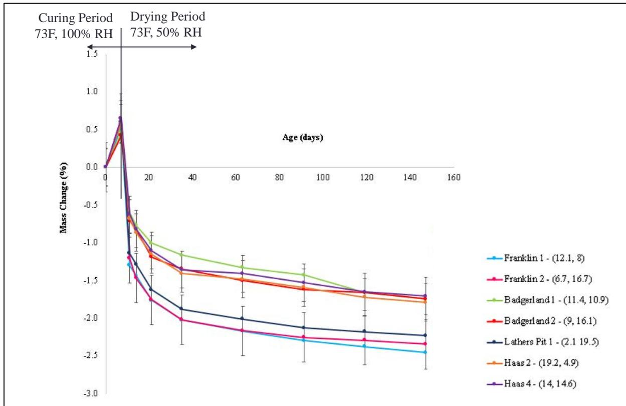
Figure 27: The Mass Change of the Mixtures on Each Day of Interest from Drying for the Testing in Part II.
