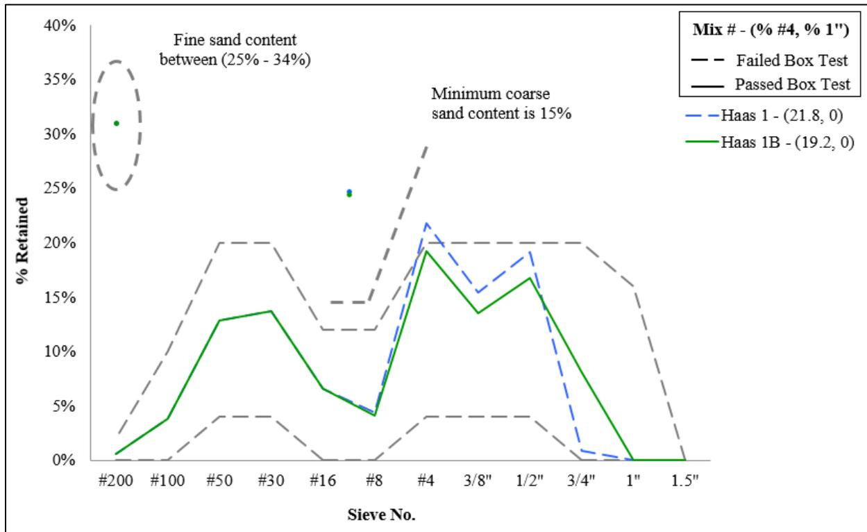
Figure 14: Mixture 1 and 1B Plotted on the Tarantula Curve. Dashed Lines Failed and Solid Lines Passed the Box Test.
