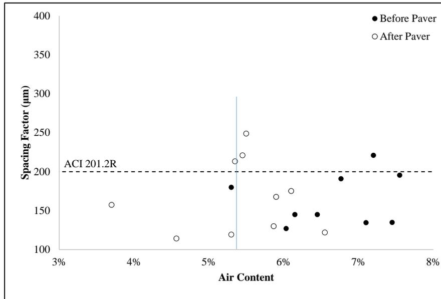
Figure 61: Air content compared to Spacing Factor for the samples investigated with a hardened air void analysis.
