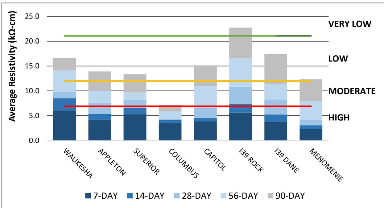
Figure 74: Resistivity Gain by Location using Surface Resistivity.
