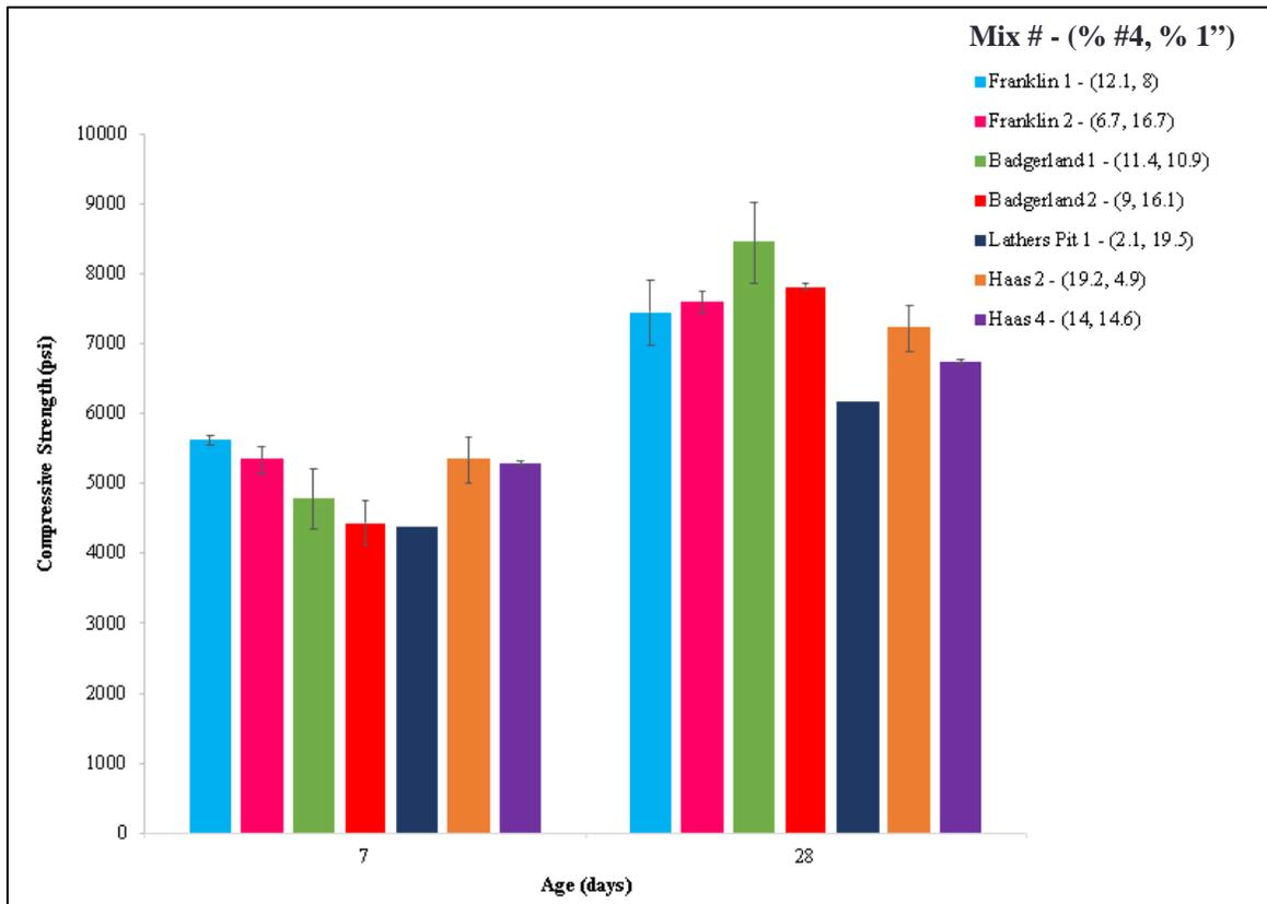
Figure 25: Average Compressive Strength of the Mixtures on Each Day of Interest.
