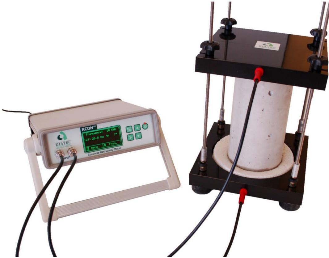
Figure 5: Bulk Resistivity Apparatus.
