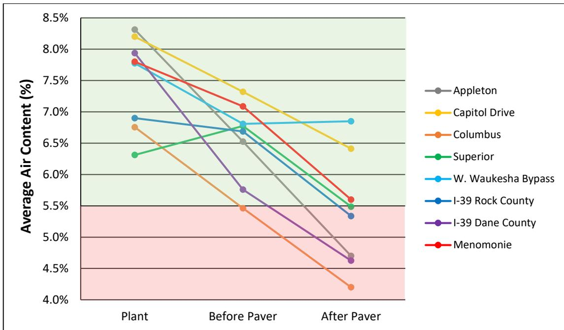
Figure 63: Air content changes throughout production and placement from the plant to before and after the paver.
