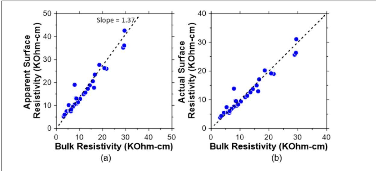
Figure 72: (a) Bulk Resistivity vs. Measured (Apparent) Surface Resistivity. (b) Bulk Resistivity vs. Corrected (Actual) Surface Resistivity.
