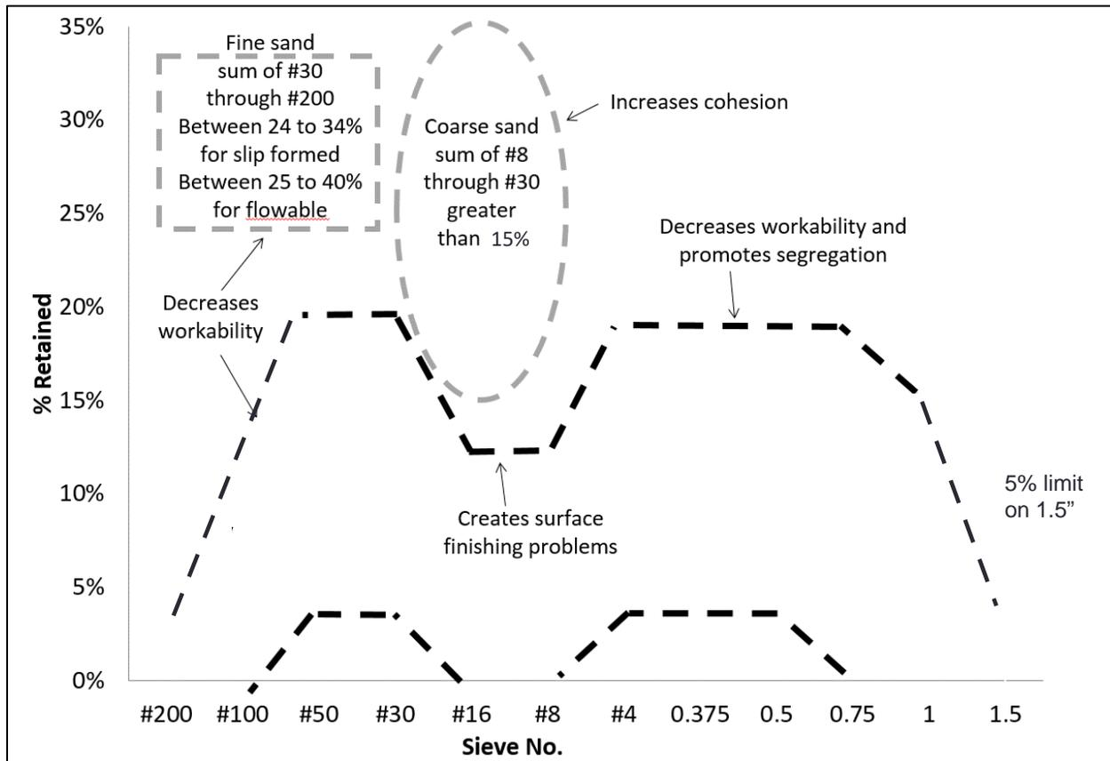
Figure 28: The Tarantula Curve Limits are Adjusted for Slip Formed Concrete that Uses Up to 1.5-in. (38.1 mm) Stone in the Concrete Mixture.
