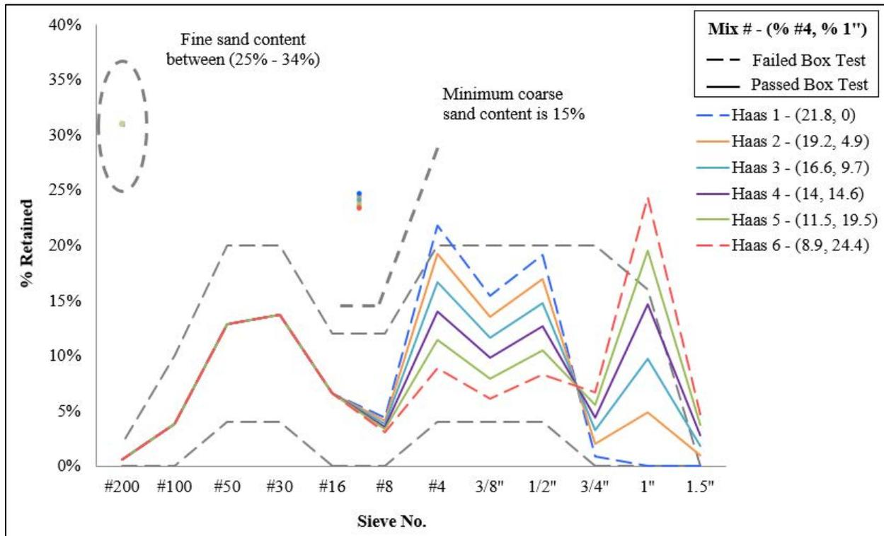
Figure 15: The Mixtures Plotted on the Tarantula Curve for Mixtures 1 through 6. Dashed Lines failed and Solid Lines Passed the Box Test.
