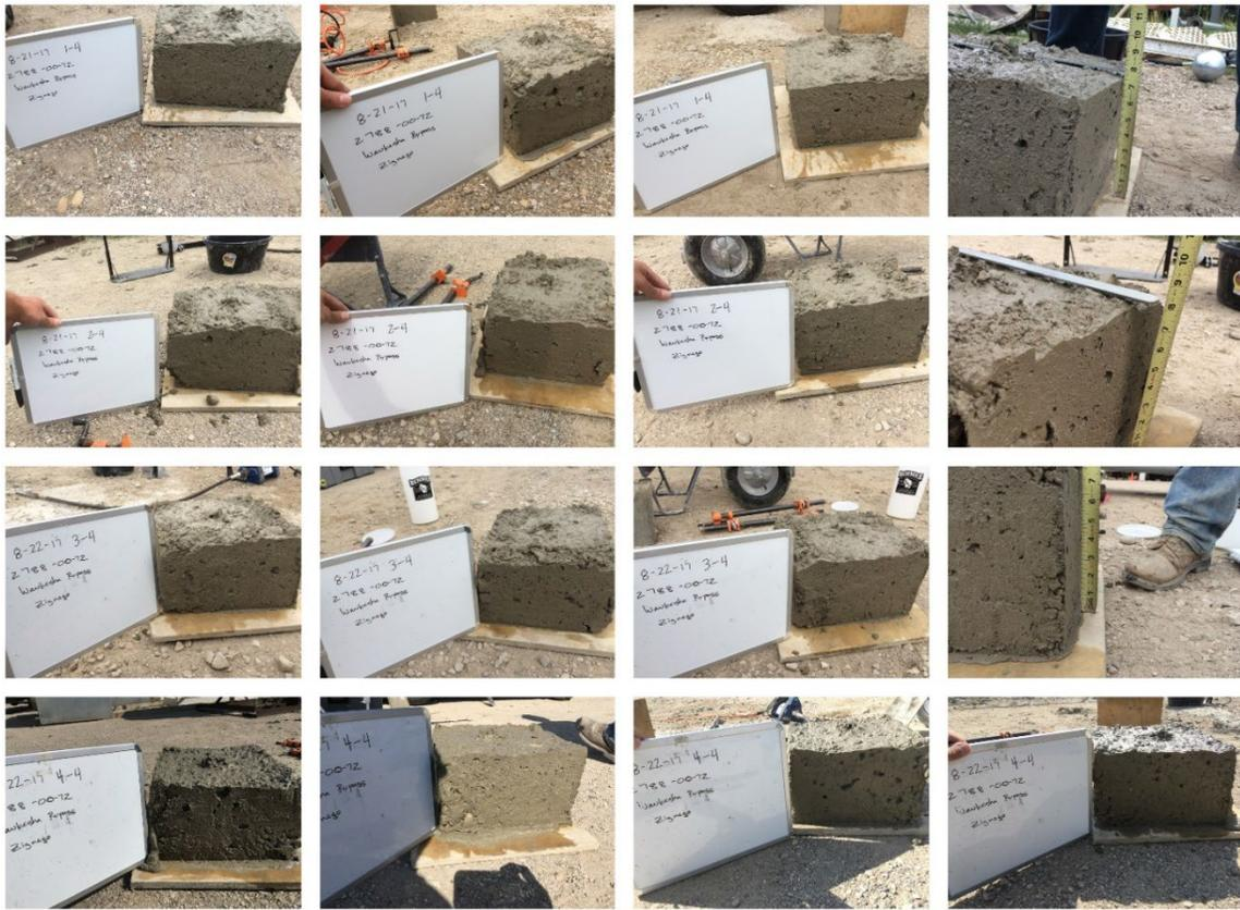
Figure 40: West Waukesha Bypass Box Test Photos.
