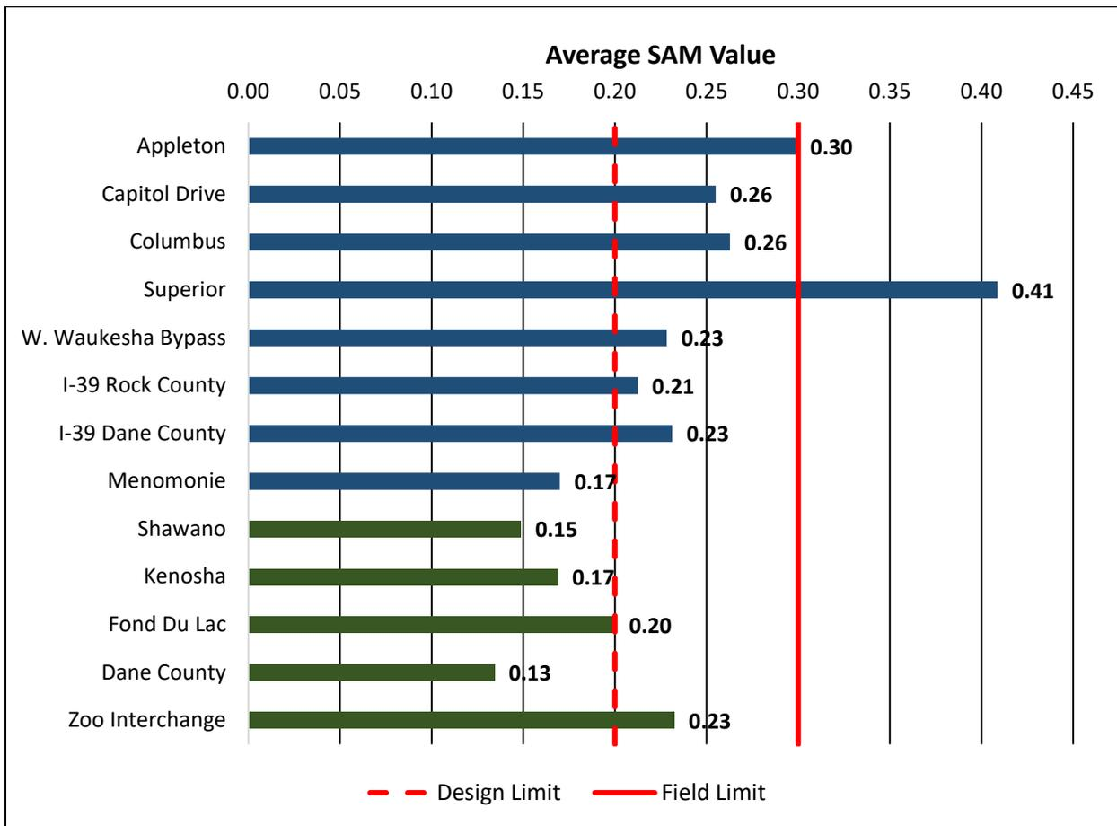
Figure 67: Comparison of Average SAM values from Phase I Projects using Rodding and Battery Vibration Consolidation to Phase II Projects using MinT Consolidation. Phase I Projects are Shown with Blue Bars and Phase II Projects are Shown with Green Bars.
