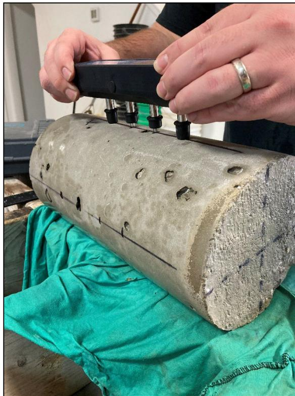
*Figure 4: Surface Resistivity Apparatus measuring a 6 in. x12 in. (152.4 mm x 304.8 mm) cylinder.*
