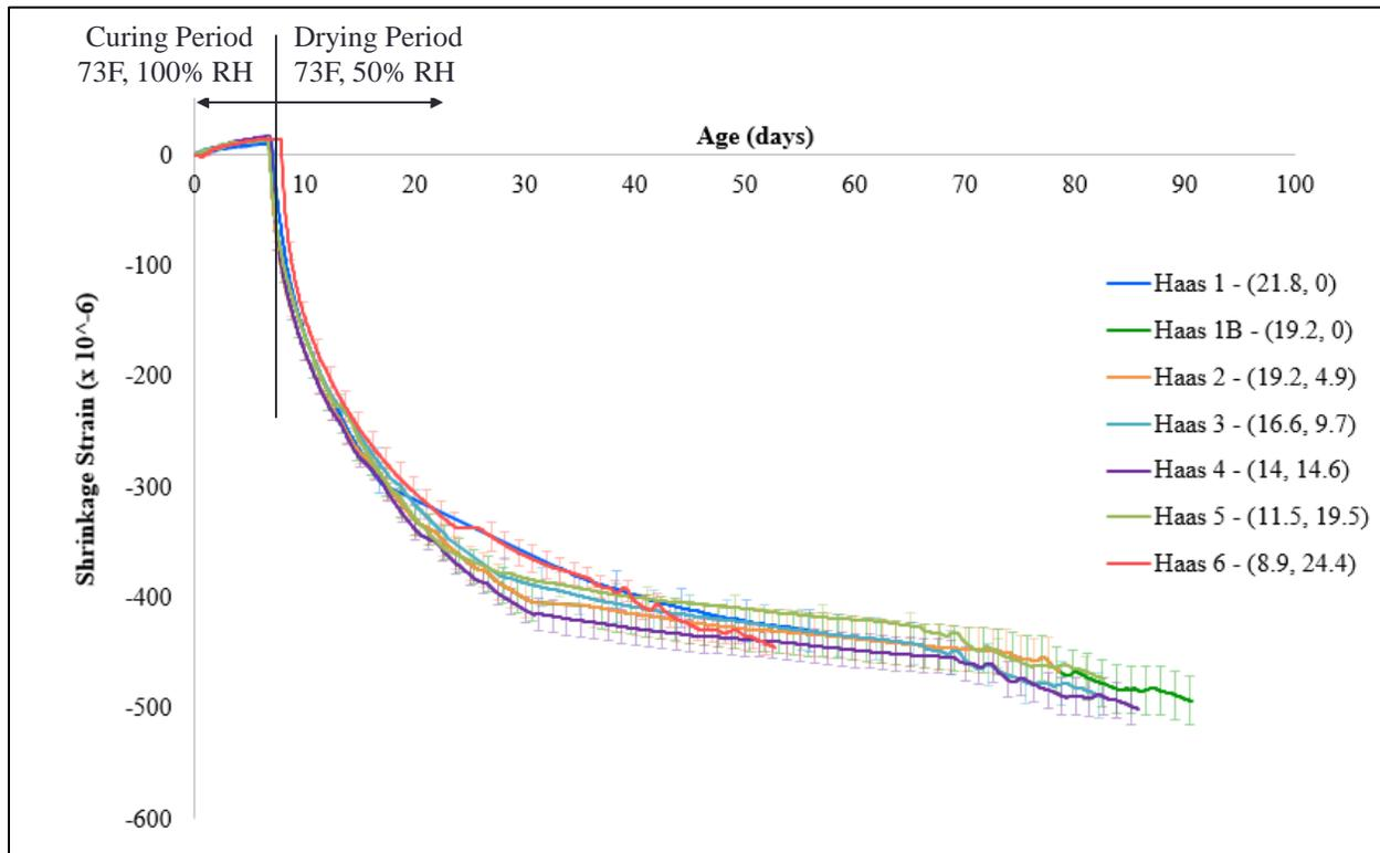
Figure 21: Average Shrinkage Strains from Mixtures During Curing and Drying Periods.
