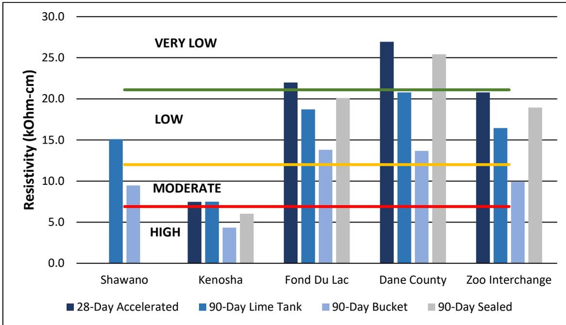
Figure 75: Surface Resistivity 28-Day Accelerated vs. Multiple 90-Day Curing Methods.
