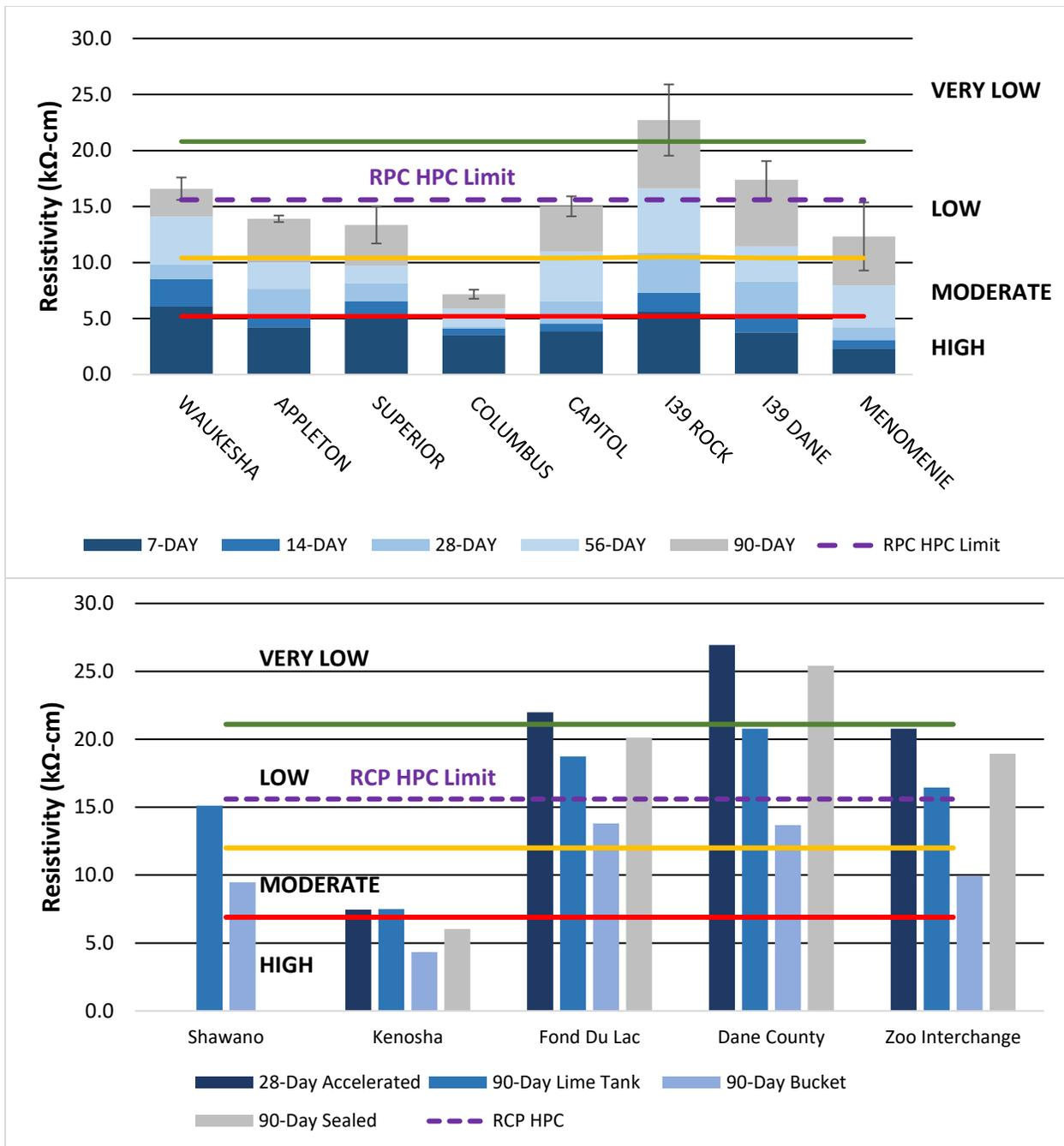
Figure 83: Phase I and II Resistivities Compared to the Rapid Chloride Penetration High Performance Concrete Equivalent Surface Resistivity Specification.
