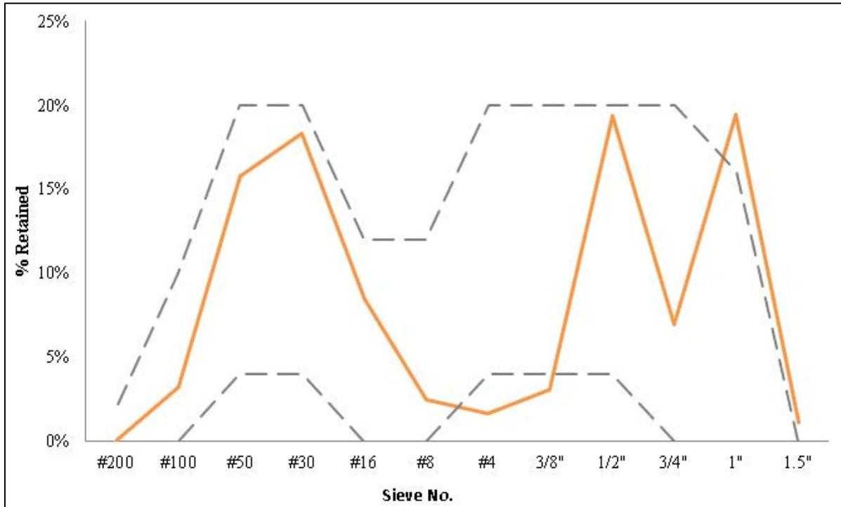
Figure 29: The Combined Aggregate Gradation Used for the Testing.
