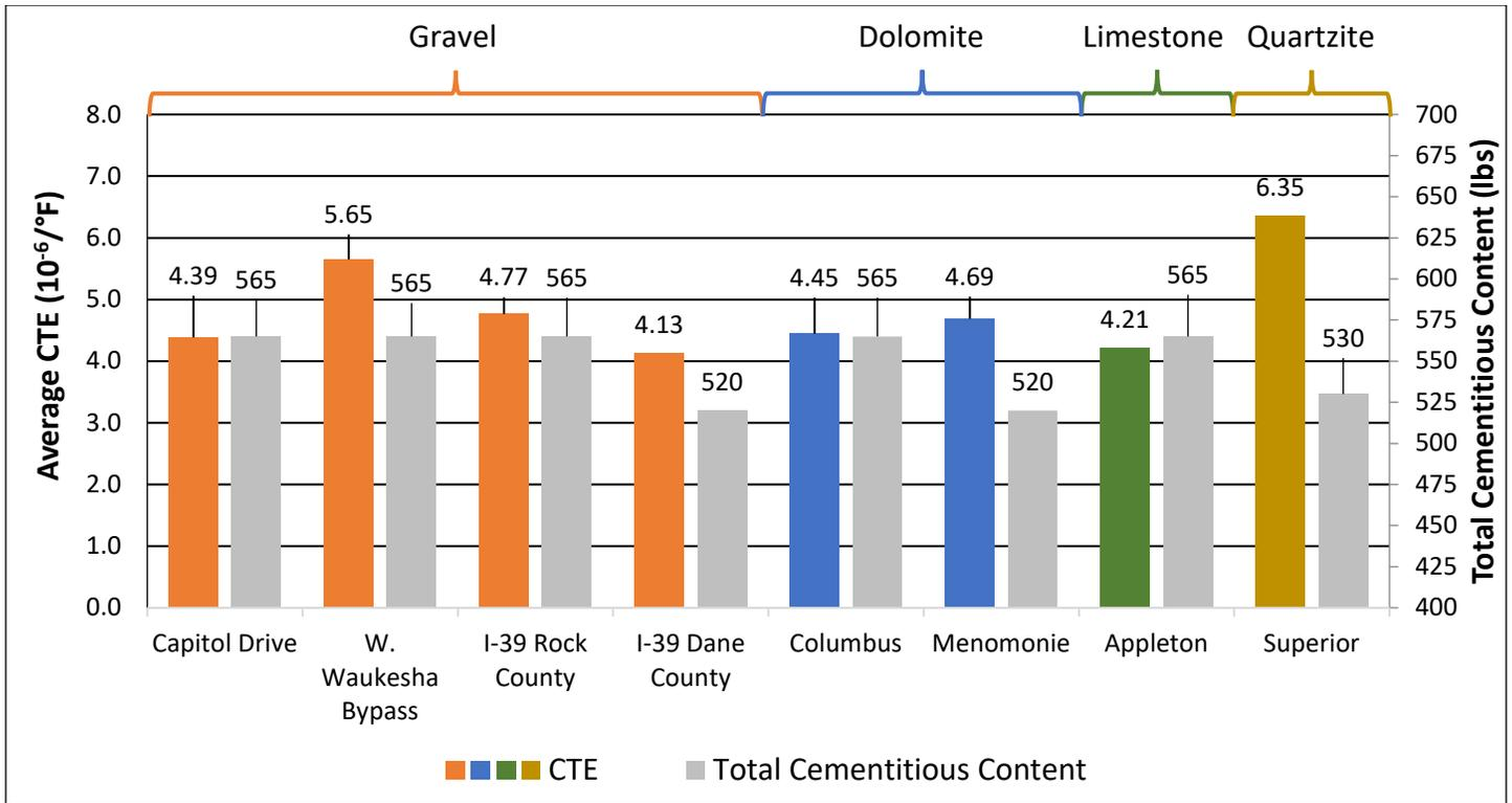
Figure 78: Average Coefficients of Thermal Expansion by Total Cementitious Content and Aggregate Type.
