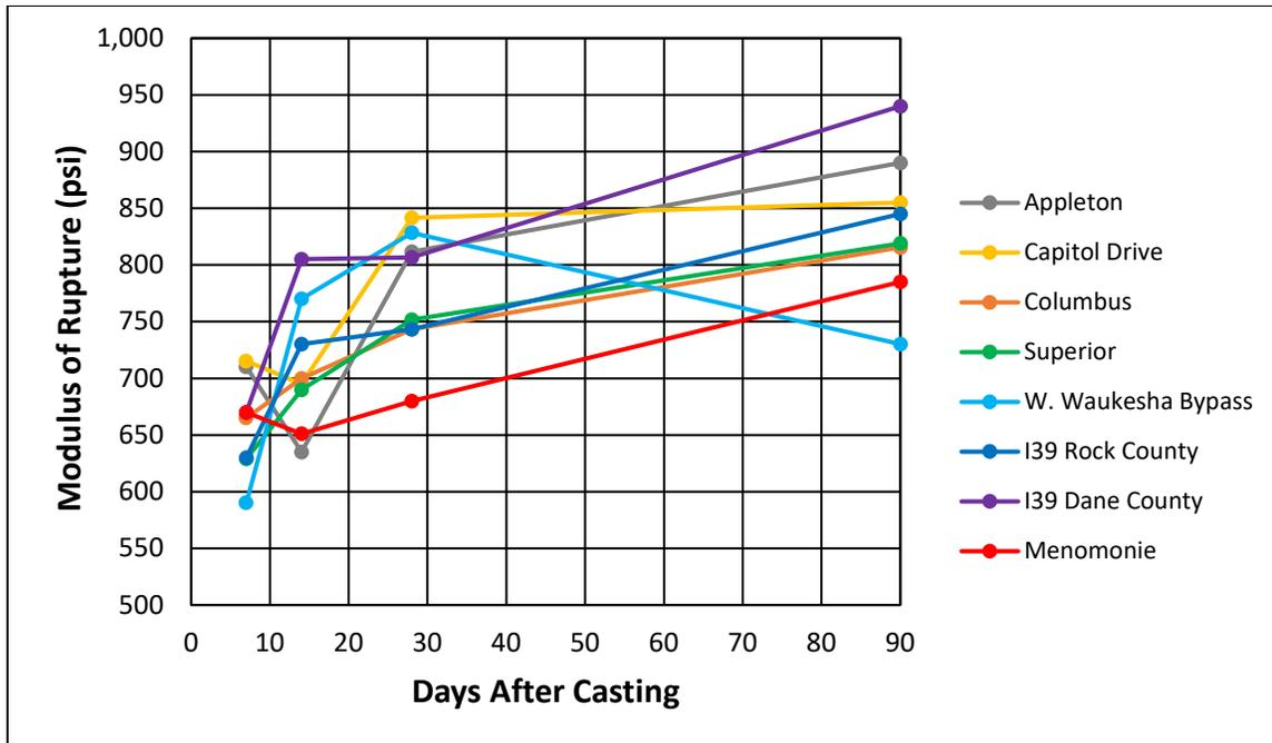
Figure 58: Phase I Modulus of Rupture strength development with curing time.
