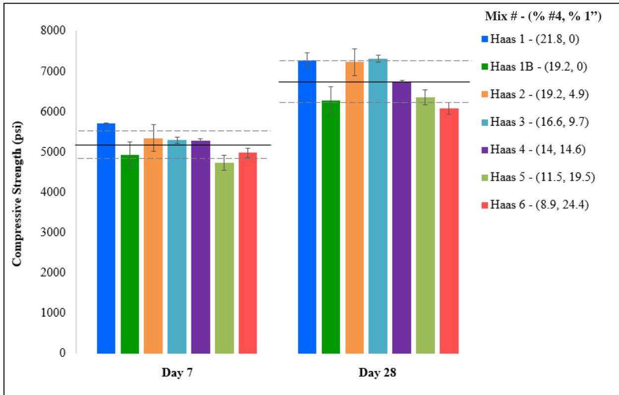
Figure 18: Average Compressive Strength of the Mixtures on Each Day of Interest.
