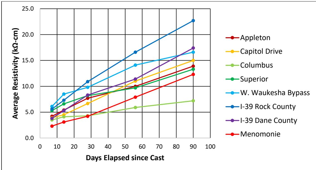
Figure 73: Resistivity vs. Days Elapsed Since Casting using Surface Resistivity.
