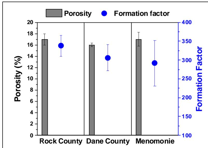
Figure 76: Porosity and formation factor based on bulk electrical resistivity measurement.
