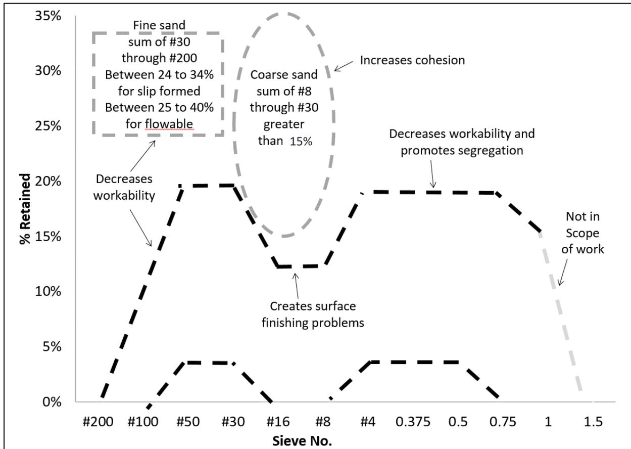
Figure 12: The Tarantula Curve with the three design criteria highlighted and the description of what will happen if these criteria are not met.
