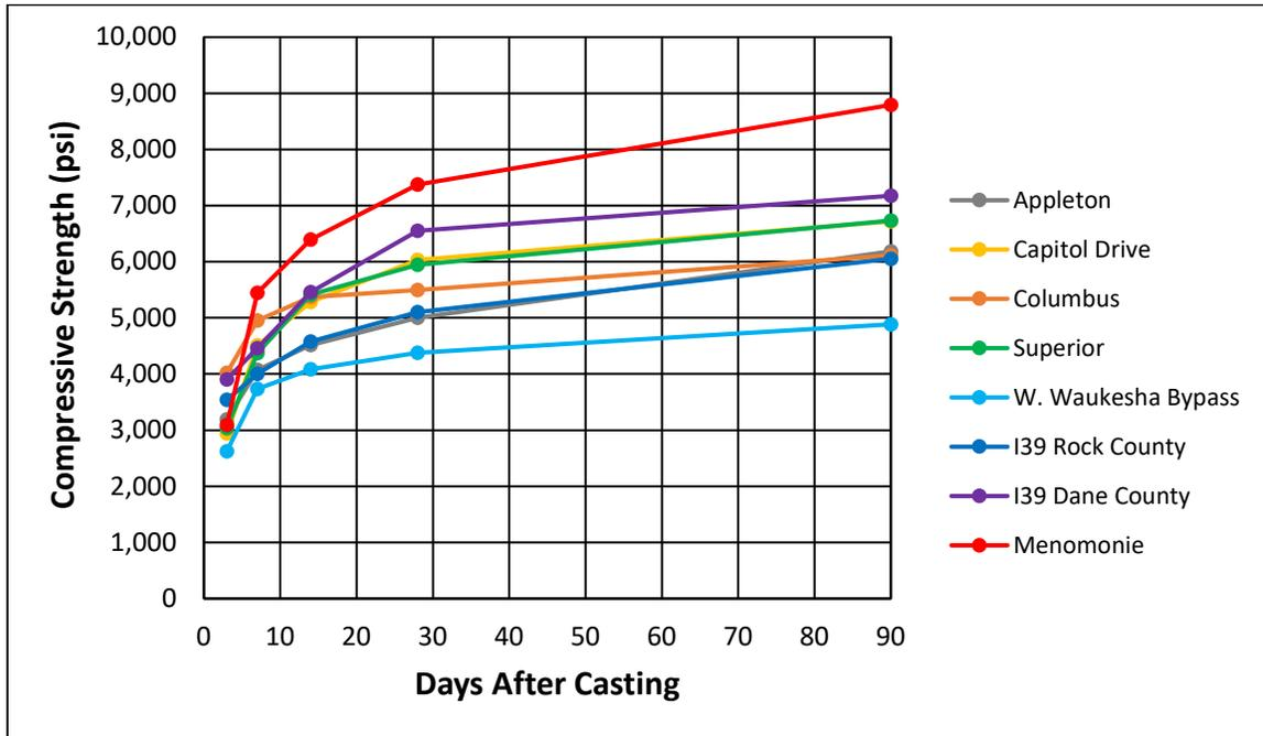
Figure 57: Phase I Compressive Strength development with curing time.
