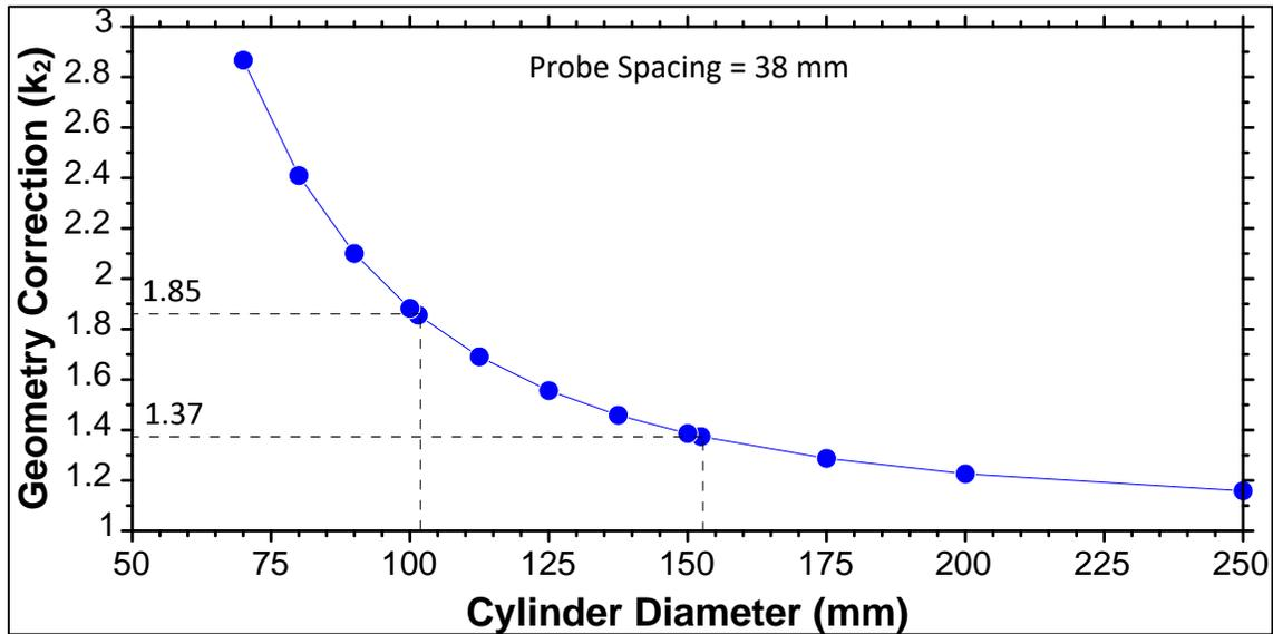
Figure 71: Geometrical Correction for Surface Resistivity Determination
