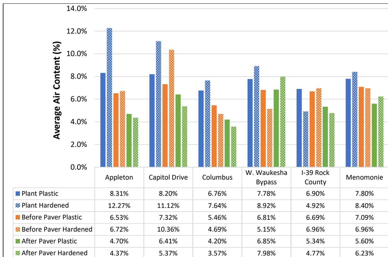
Figure 66: Comparison of Plastic Air to Hardened Air Content.
