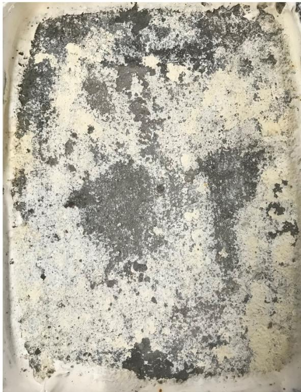
**Figure C.7 FA SME-PS applied dry after 50 Cycles**
