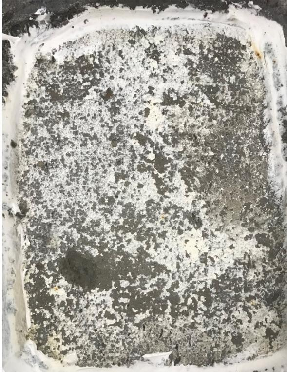
**Figure C.4 FA Control after 50 Cycles**
