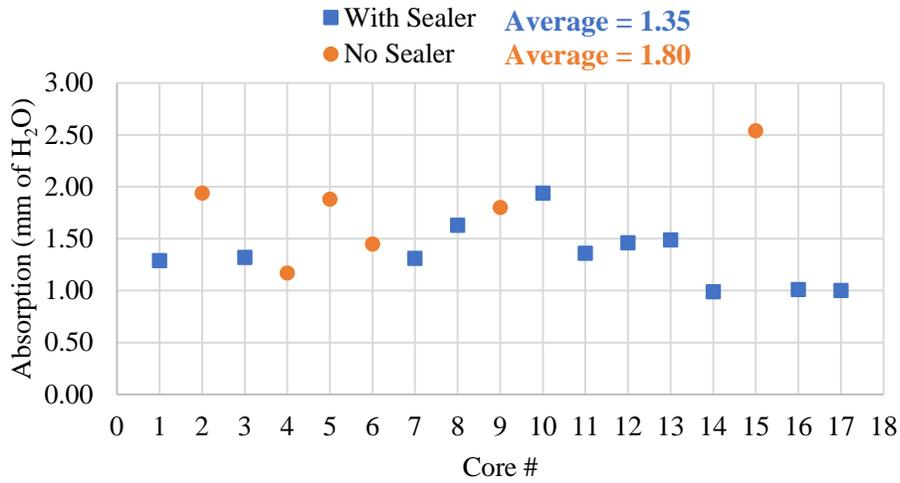
**Figure A.3 Absorption of Core Samples from I-94, I-41, and I-39**
