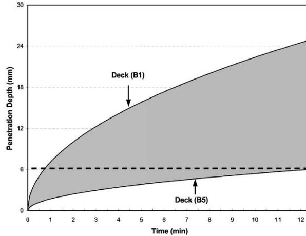
Fig. 4. Silane penetration depth against time
