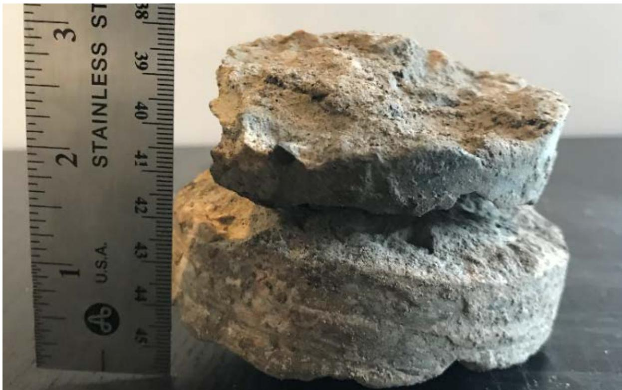
Figure A-14. Site #8, RM-3 Core #1—concrete pavement core pieces
