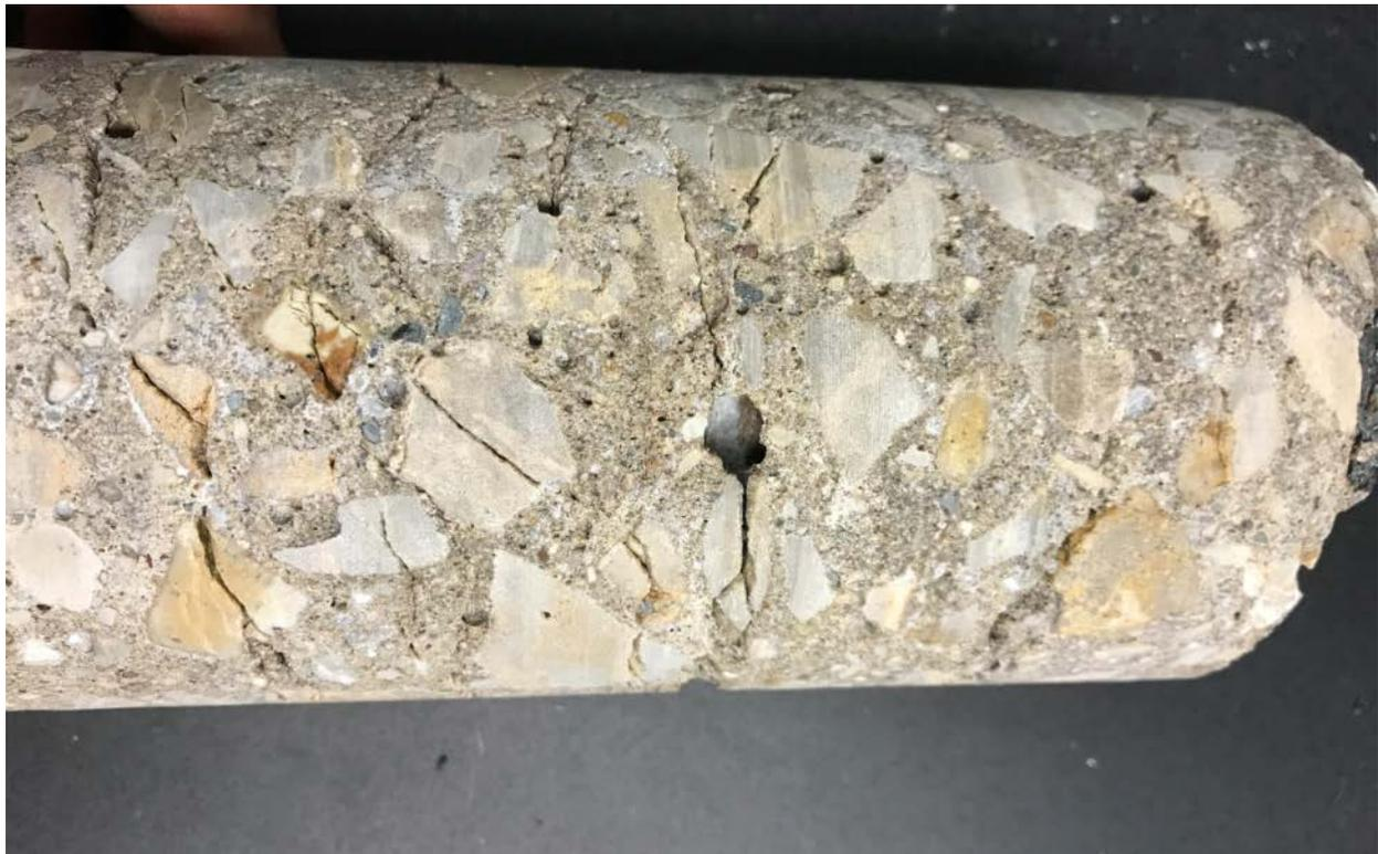
Figure A-6. Site #1, RM-1 Core #2—Closeup of PCC core
