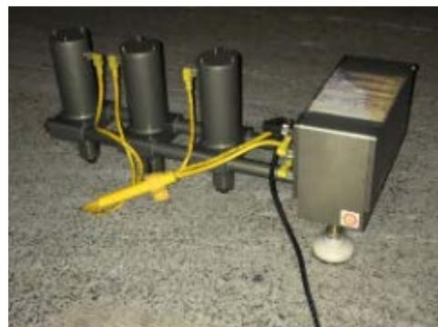
Figure 3-1. Portable seismic pavement analyzer (PSPA).
