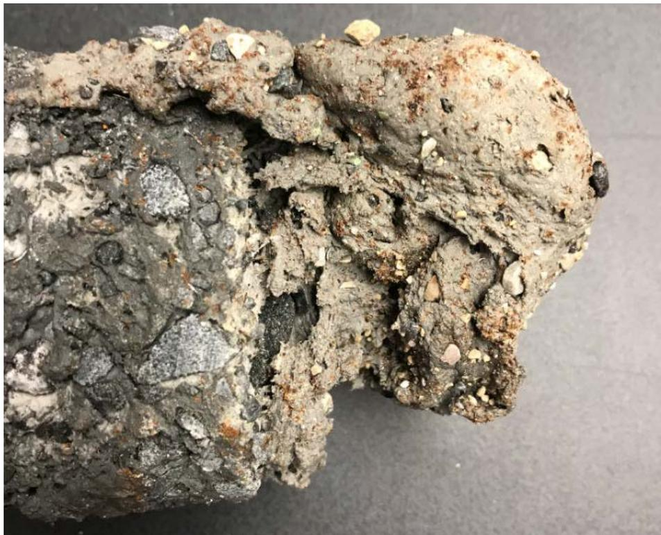
Figure A-10. Site #1, RM-1 Core #3—Closeup of melted material (US 12/18, Madison Beltline).
