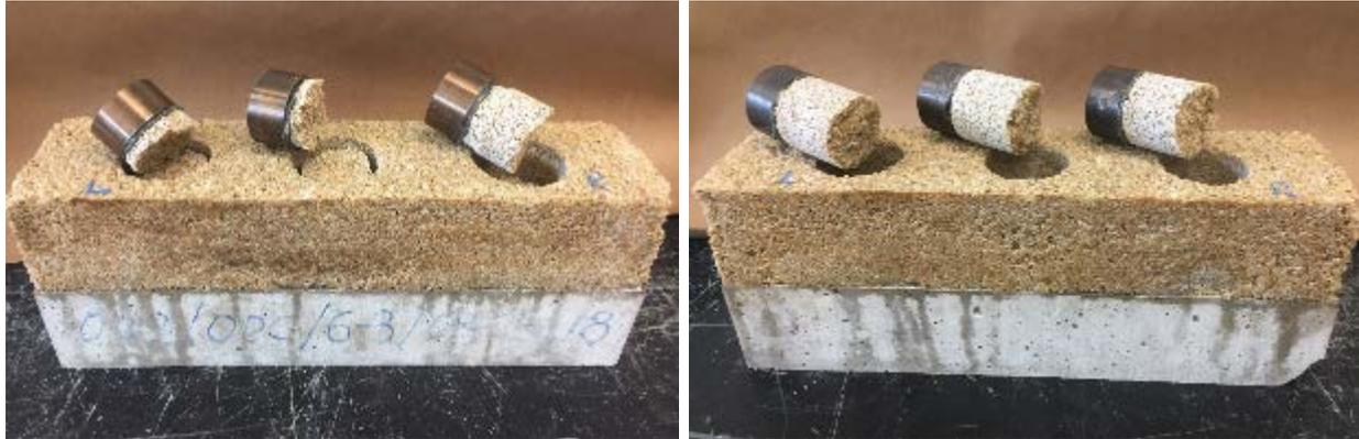
Figure 4-12. Failures observed after pull-off testing at 23 °C (left, shallow failures) and -10 °C (right, deep failures).
