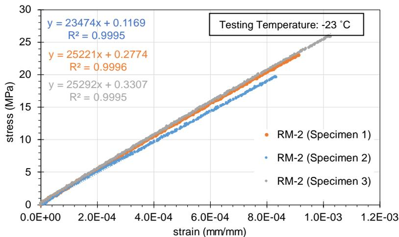
Figure 4-13. Stress-strain response curves for RM-2.
