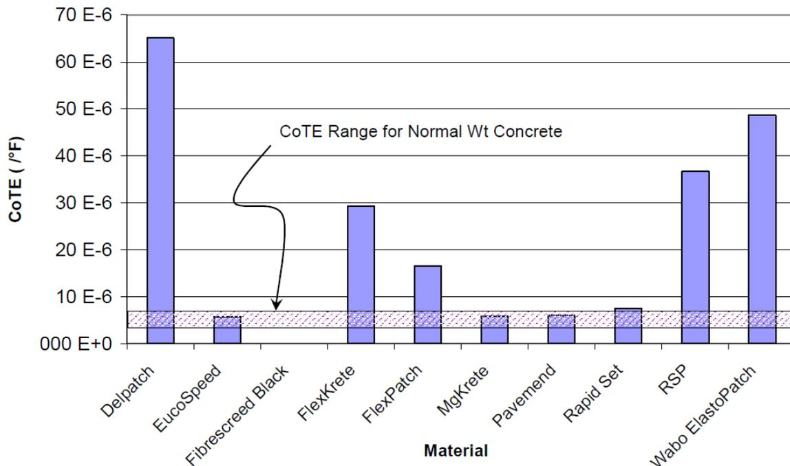
Figure 2-5. CTE of the repair materials in Texas study (Markey et al. 2006).
