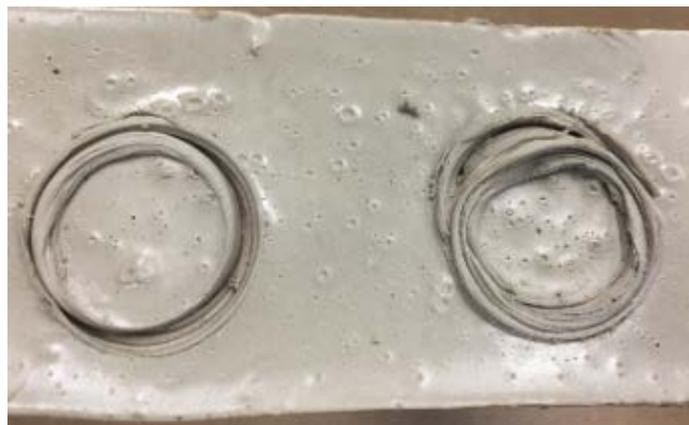
Figure 4-8. Unsuccessful specimen preparation effort for bond testing.
