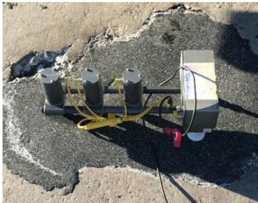
Portable seismic pavement analyzer testing of a repaired pavement section on WIS 66 in Stevens Point
