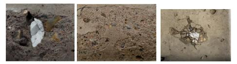
Photos of PCC cylinders during F-T cycles showing the effect that CA quality had on the cylinders. Photos show CA fracture, PCC surface scaling and CA initiated cracking in the PCC cylinder surface, respectively.
