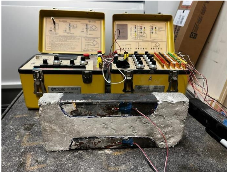
Figure 32. Restrained dog bone specimens.
