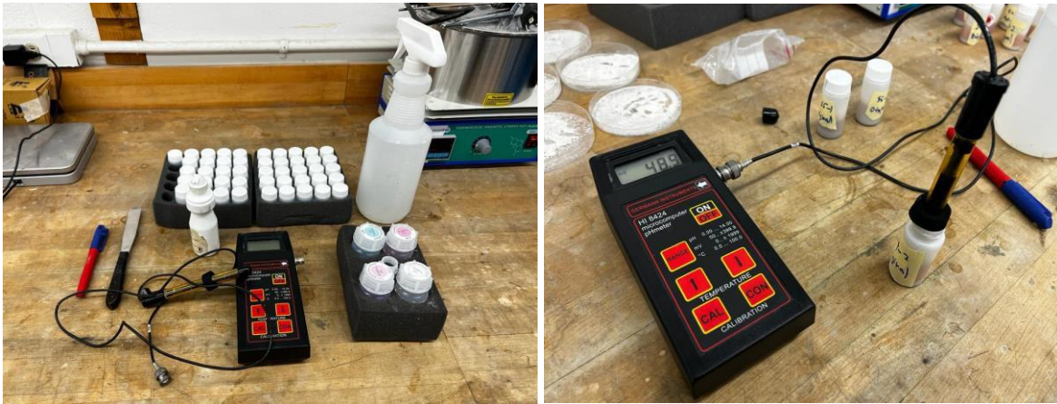
Figure 30. Rapid Chloride test setup and measurement
