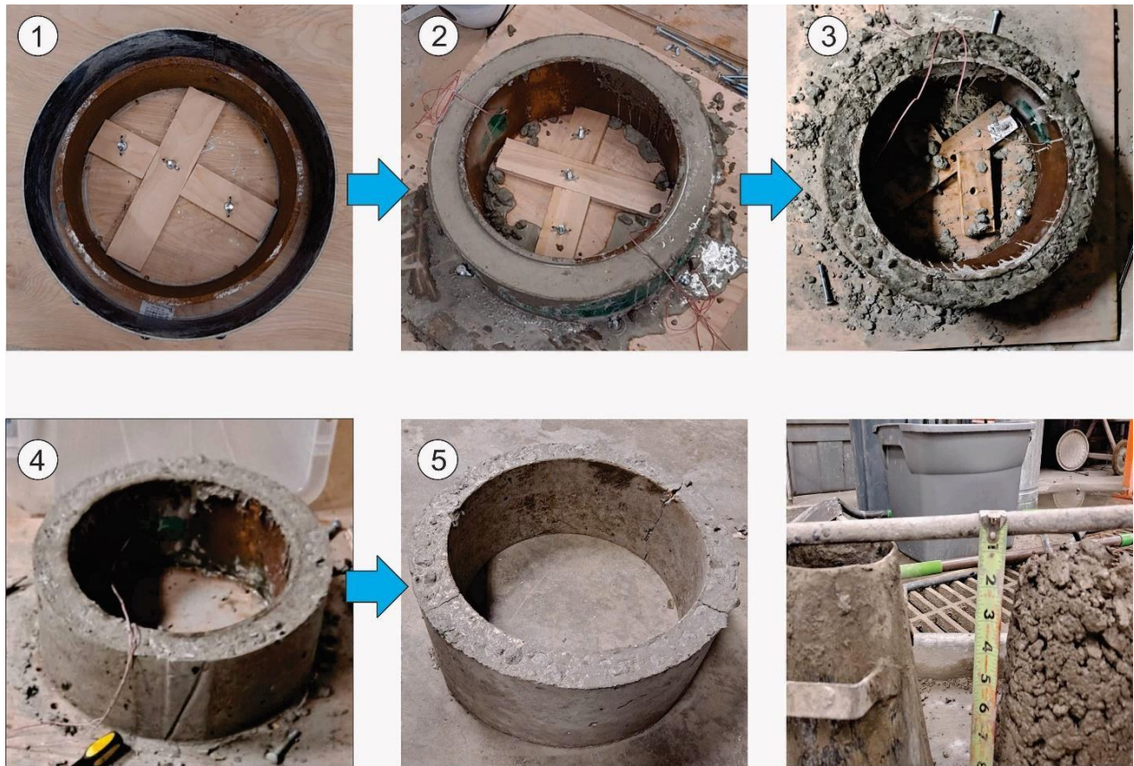
Figure 28. The ring testing process and samples.
