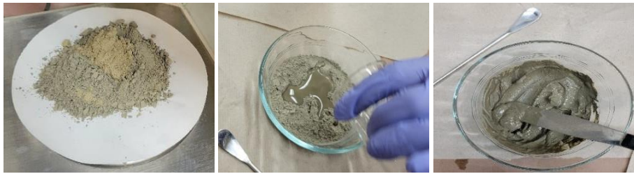
Figure 27. The sequence of HOH sample preparation from left to right.
