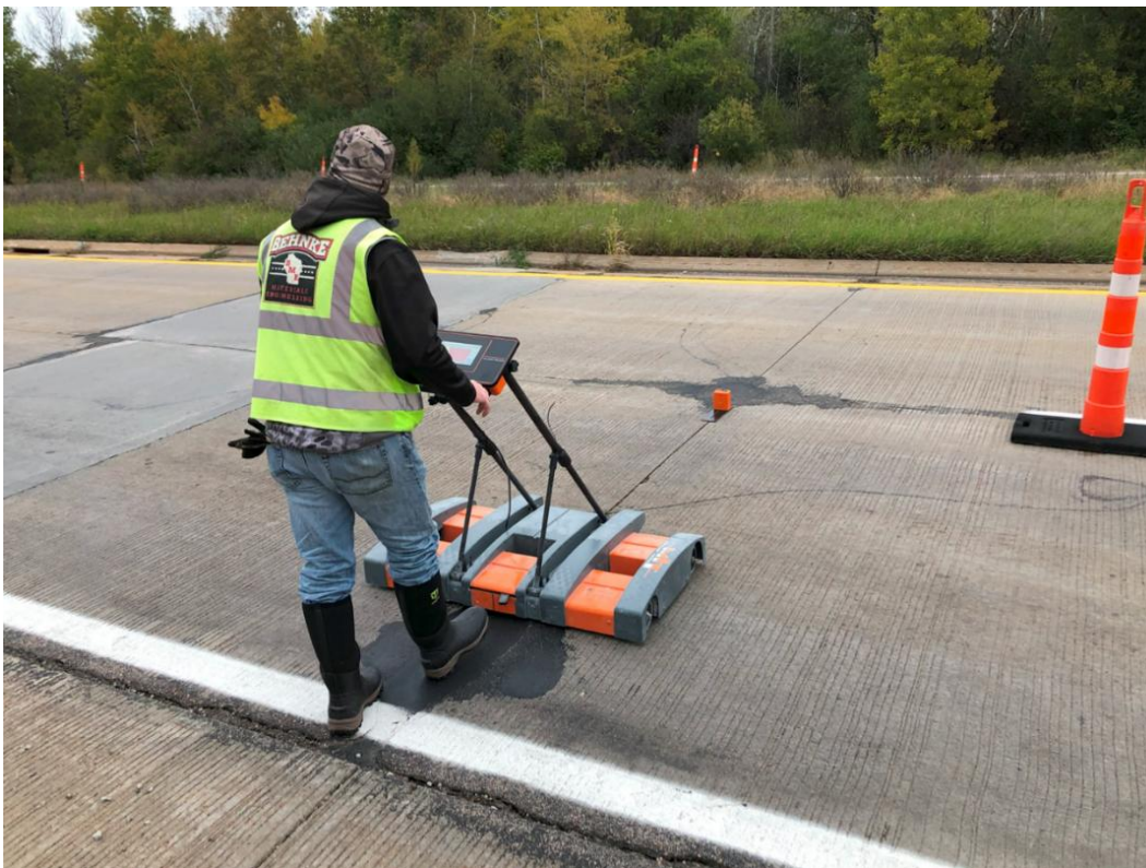
Figure 4. MIT-DOWEL-SCAN testing in Chippewa County on STH 178 NB.
