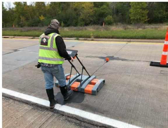
MIT-DOWEL-SCAN testing in Chippewa County
