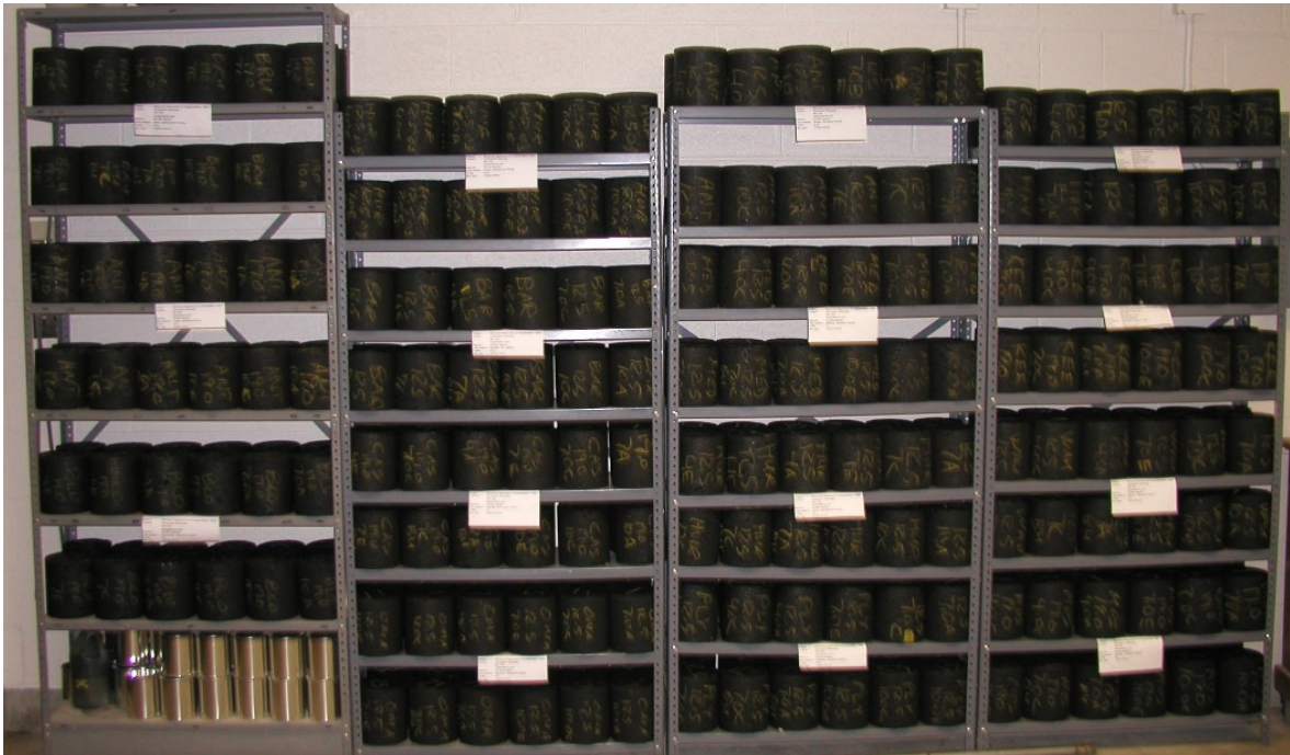
Figure 5.4. Prepared gyratory specimens
