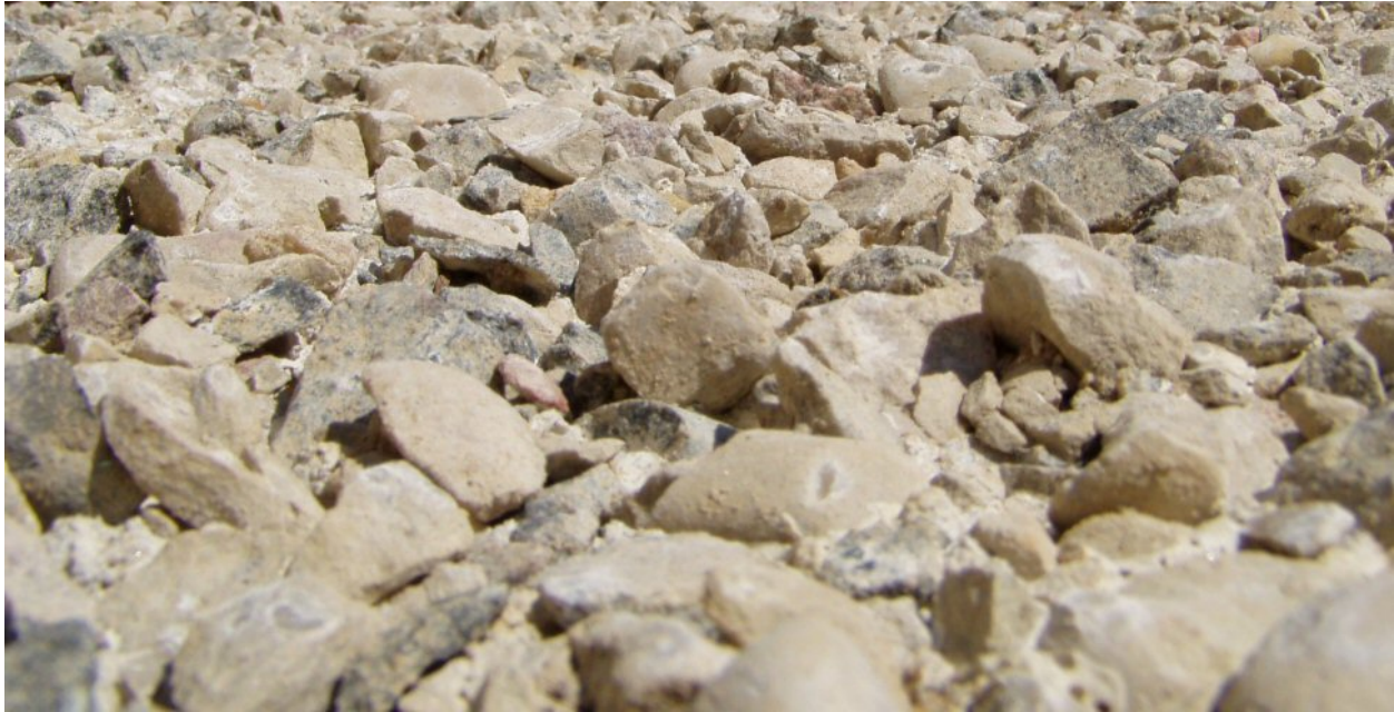
Figure 14. Open-graded base material (adhered to bottom of slab).
