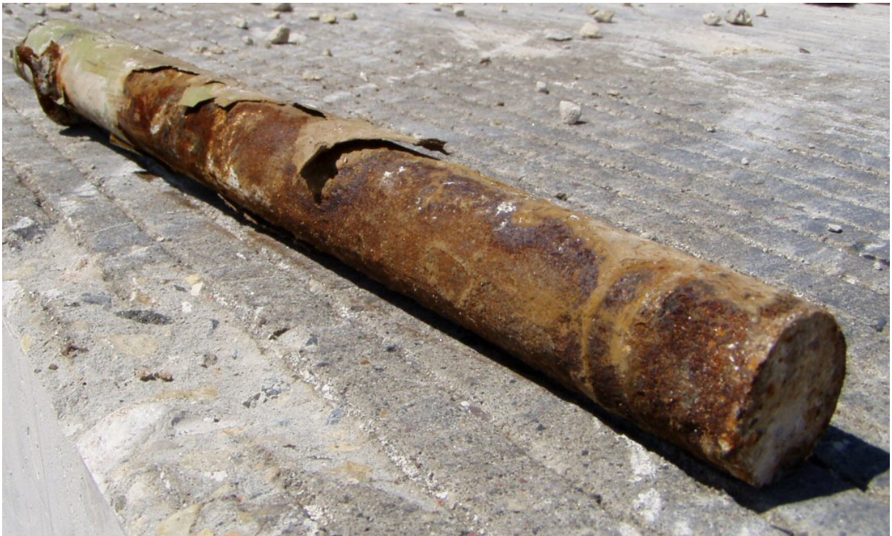
Figure 13. Loose dowel showing ineffectiveness of epoxy coating once damaged. Note abrasion due to loose state and interaction with concrete.
