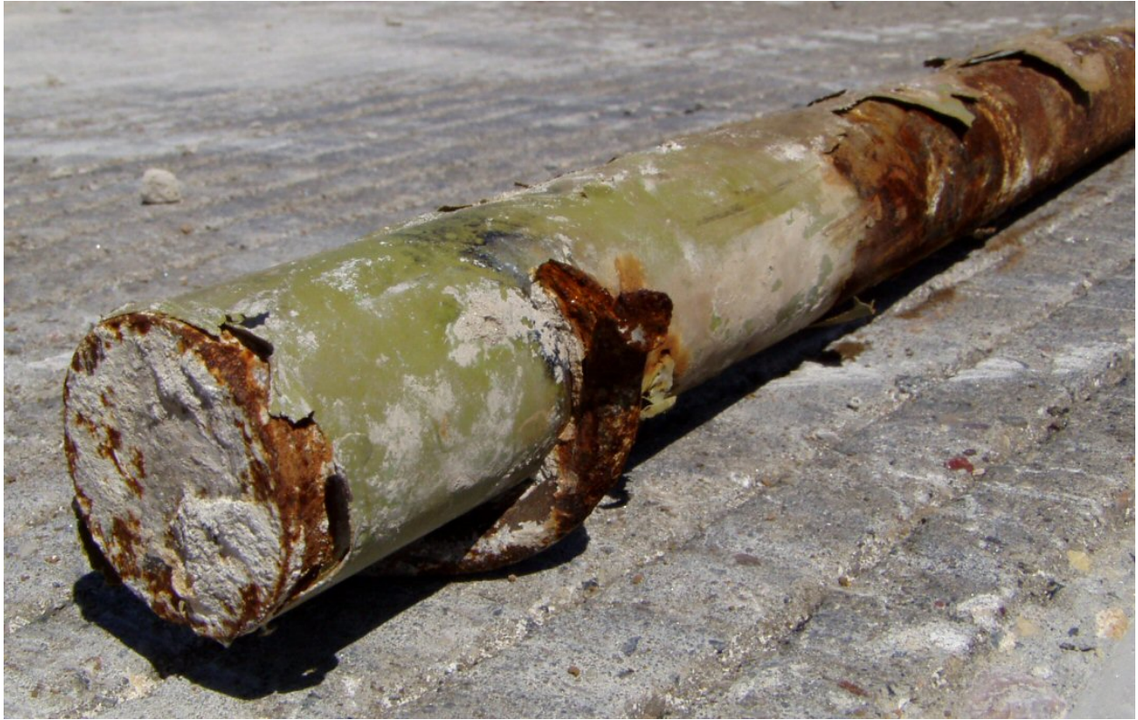
Figure 12. Loose dowel showing ineffectiveness of epoxy coating once damaged.
