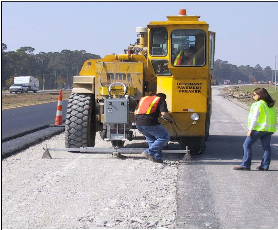
Figure 12 RMI bulk modulus test on rubblized PCC highway pavement.
