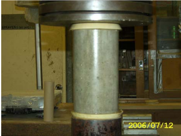
Fig. 4-1. Compressive strength test of concrete
