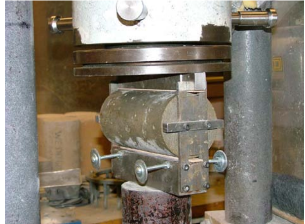
Fig. 4-2. Splitting tensile strength test of concrete
