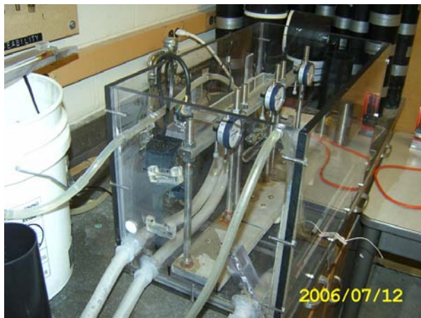
Fig. 4-4. CTE apparatus (Left Side View)
