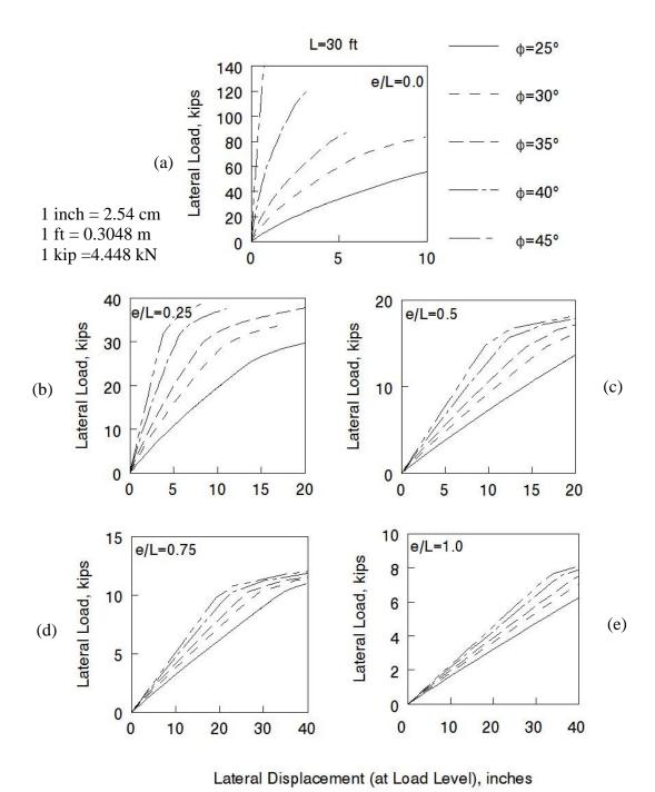
Figure 64: Design Criterion 2 for Piles in Cohesionless Soils with Embedded Length  $L=30~{\rm ft}$
