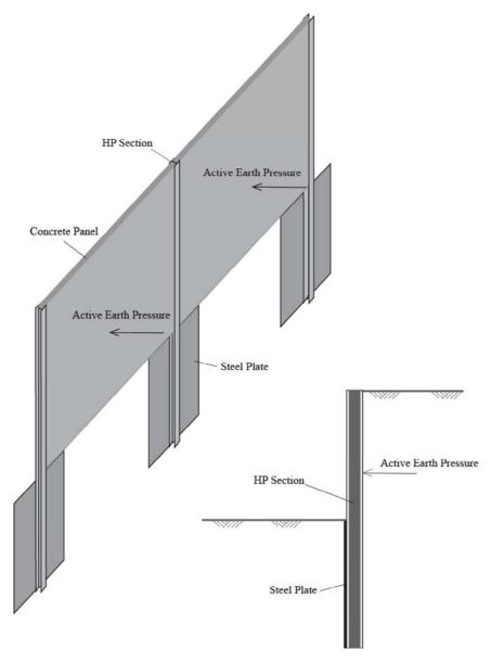
Figure 2 Alternative System (Pile with Plate)
