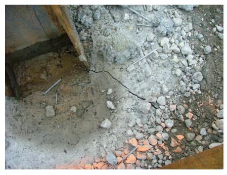
Figure 47: Cracking at 556 kN-667 kN (125,000 lb-150,000 lb)
