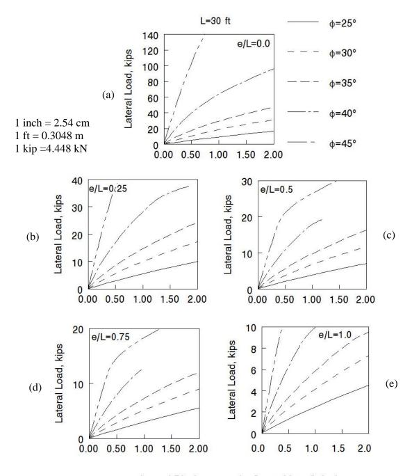
Lateral Displacement (at Ground Level), inches
