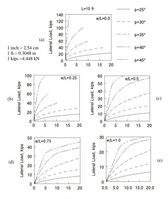
Lateral Displacement (at Load Level), inches
