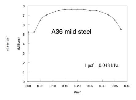
Figure 54: Stress-Strain Curve of Steel Used in the FE Analysis (Elasto-Plastic Model)
