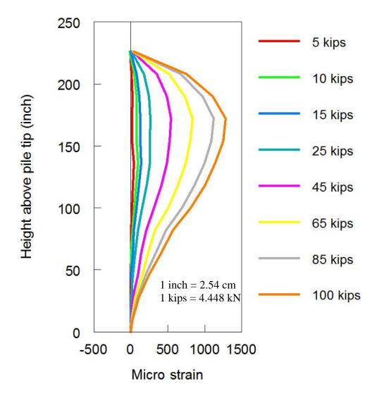
Figure 35: Measured Strains (Pile with Steel Plate)
