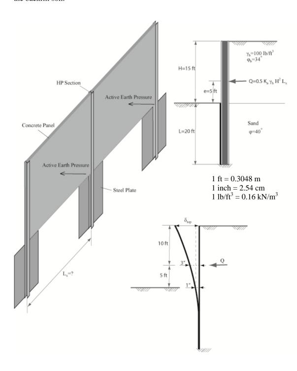
Figure 65: Design Example 1--Pile in Sand
