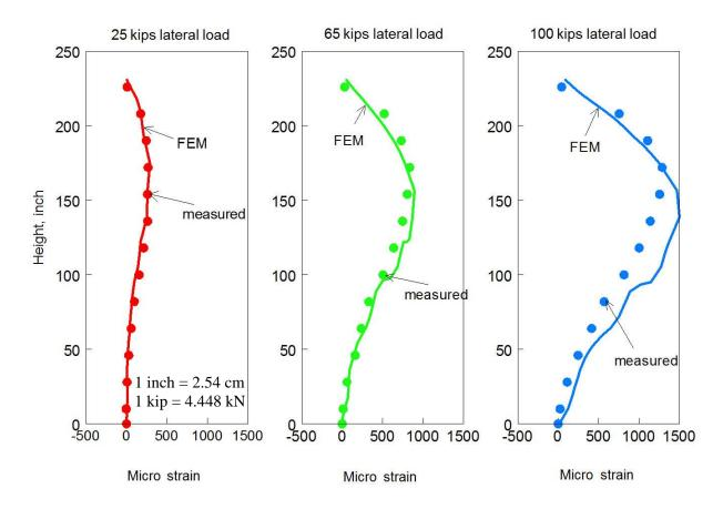
Figure 58: Comparison between Measured and Calculated Strains (Pile with Steel Plate)
