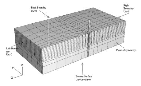
Figure 8: FEM Discretization (ODOT Test)
