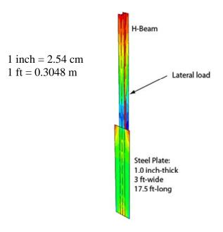
Figure 15: Alternative: Steel Plate
