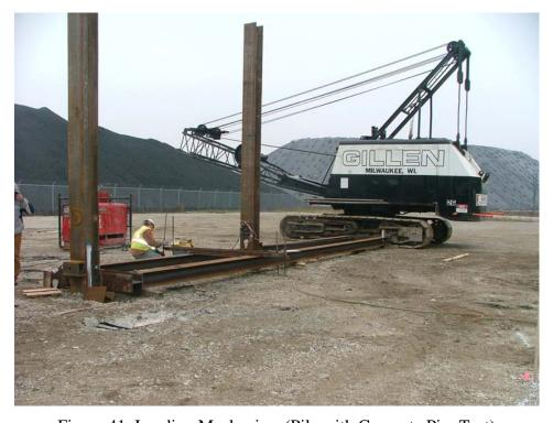
Figure 41: Loading Mechanism (Pile with Concrete Pier Test)
