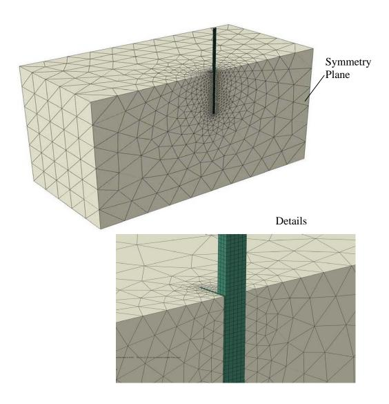
Figure 55: Finite Element Discretization of the Pile with Plate System
