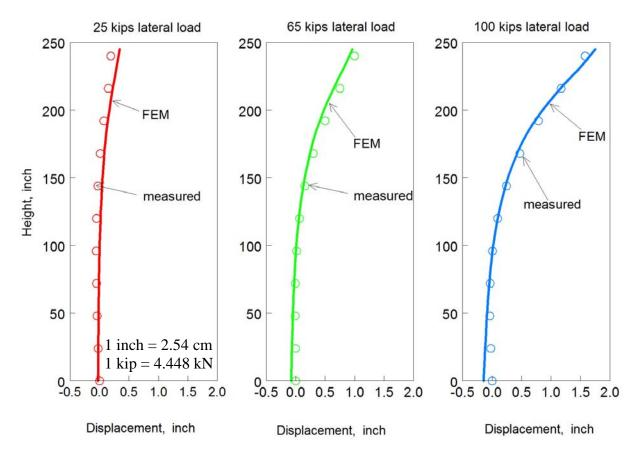
Figure 57: Comparison between Measured and Calculated Lateral Displacement Profiles (Pile with Steel Plate)
