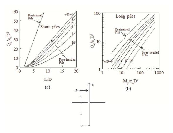
Figure 4: Broms' Method: Cohesive Soil
