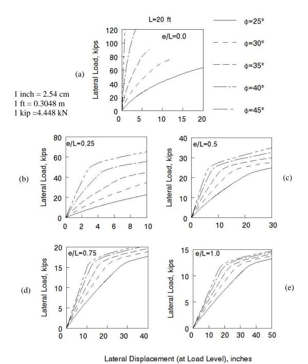
Figure 62: Design Criterion 2 for Piles in Cohesionless Soils with Embedded Length  $L=20~\mathrm{ft}$
