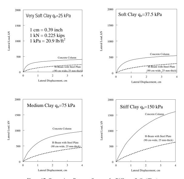
Figure 17: Comparison Between Systems for Different Soils (Clay)
