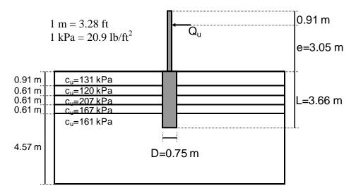
Figure 6: Ohio DOT Field Test on Laterally Loaded Post-and-Panel System
