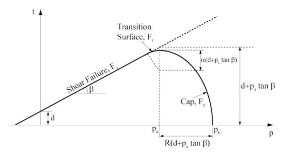
Figure 9: Modified Drucker-Prager/Cap Model in the Shear Stress Versus Mean Effective Stress Plane
