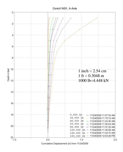
Figure 44: Measured Displacement Profiles (Pile with Concrete Pier)
