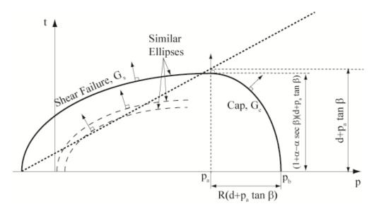
Figure 12: Flow Potential Surface in the *p-t* Plane for the Modified Drucker-Prager/Cap Model
