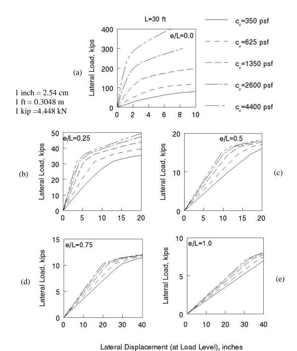
Figure 73: Design Criterion 2 for Piles in Cohesive Soils with Embedded Length L=30 ft
