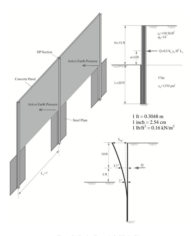
Figure 74: Design Example 3--Pile in Clay
