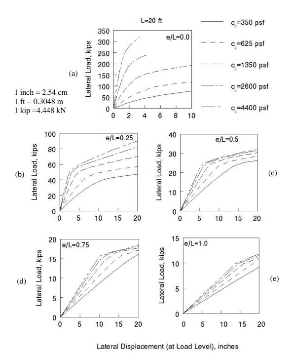
Figure 71: Design Criterion 2 for Piles in Cohesive Soils with Embedded Length L=20 ft
