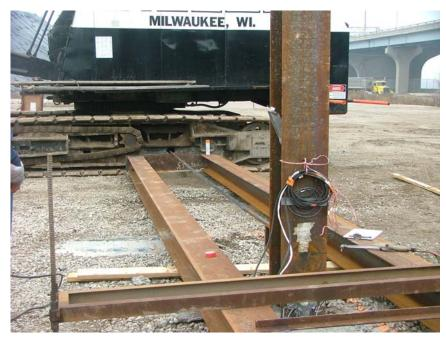
Figure 42: Loading Mechanism (Pile with Concrete Pier Test)
