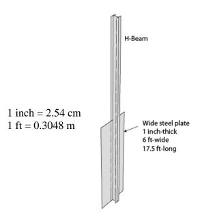
Figure 18: Alternative: Wide Steel Plate
