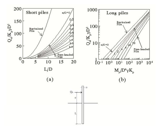
Figure 5: Broms' Method: Cohesionless Soil
