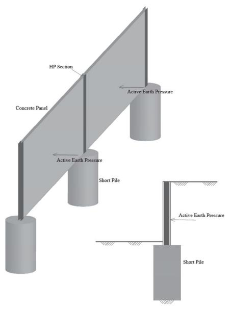
Figure 1 Post-and-Panel (Pile with Concrete Pier)
