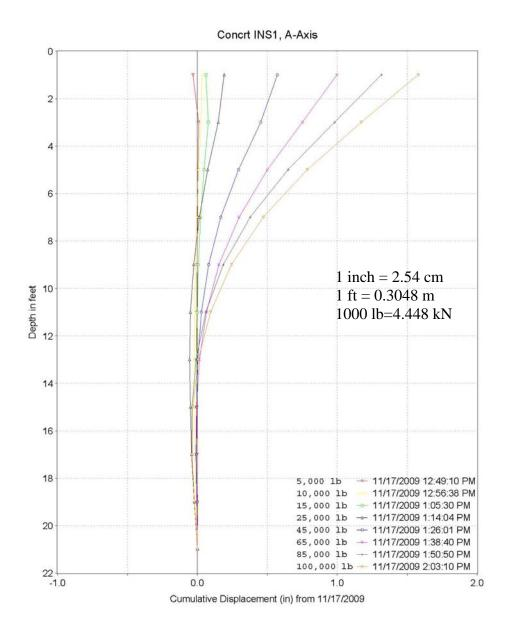
Figure 34: Measured Displacement Profiles (Pile with Steel Plate)
