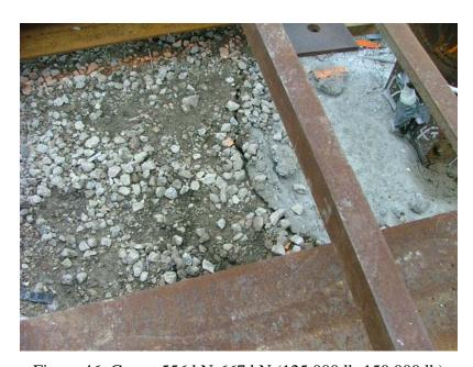
Figure 46: Gap at 556 kN-667 kN (125,000 lb-150,000 lb)
