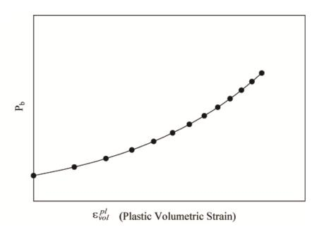
Figure 11: Hardening Curve for the Modified Drucker-Prager/Cap Model
