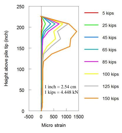
Figure 45: Measured Strains (Pile with Concrete Pier)
