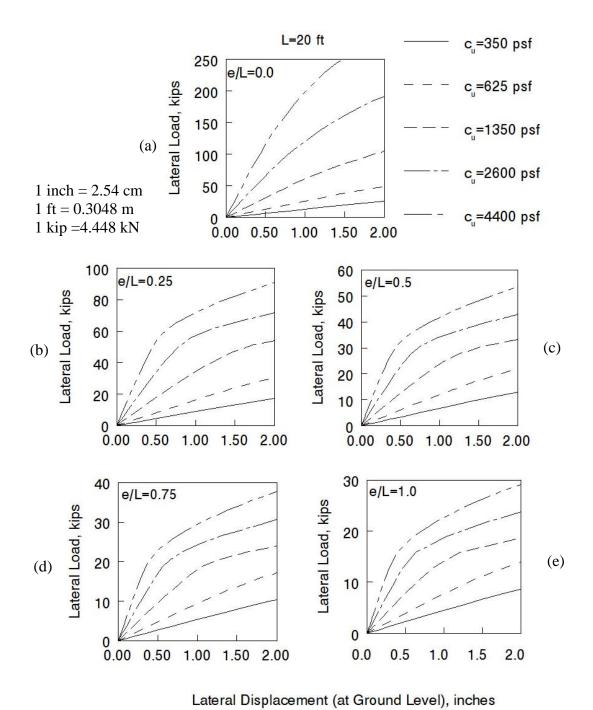
Figure 70: Design Criterion 1 for Piles in Cohesive Soils with Embedded Length L=20 ft
