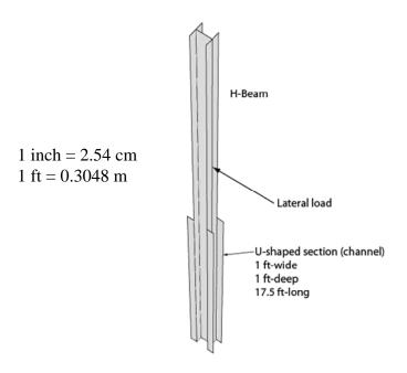
Figure 22: Alternative: Two U-Shaped Sections
