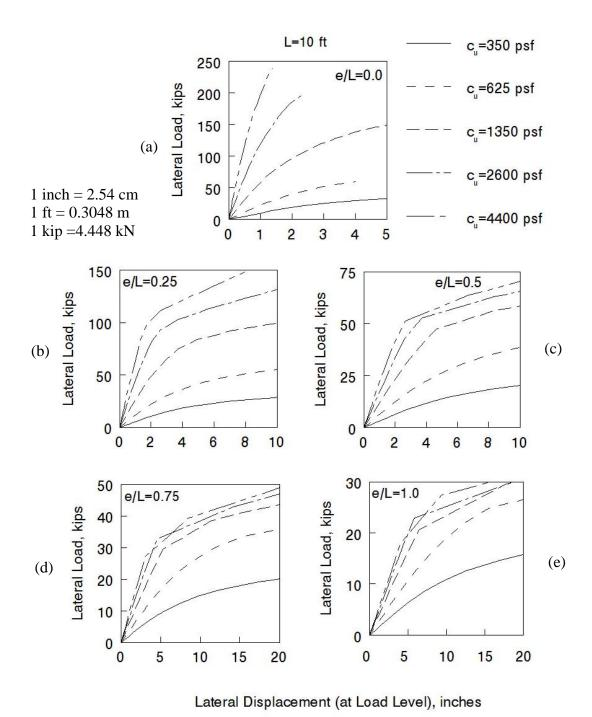
Figure 69: Design Criterion 2 for Piles in Cohesive Soils with Embedded Length L=10 ft
