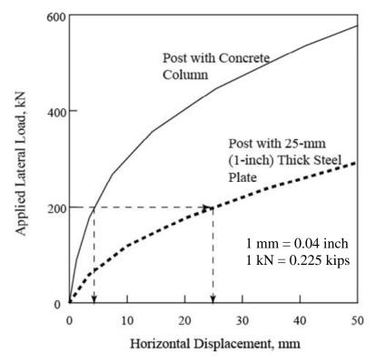
Figure 16: Comparison between Systems (Sand)
