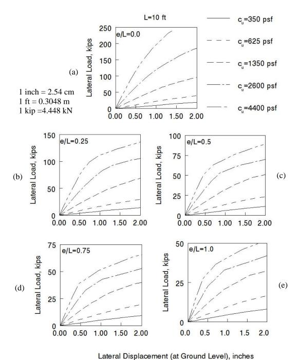
Figure 68: Design Criterion 1 for Piles in Cohesive Soils with Embedded Length L=10 ft
