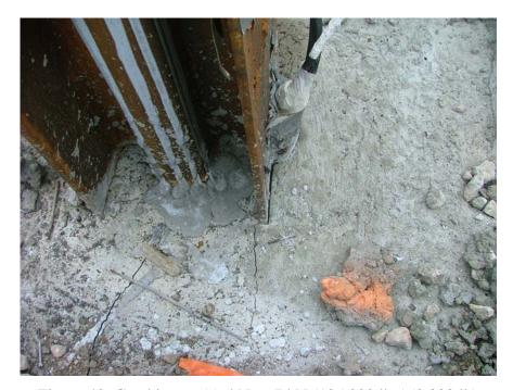
Figure 48: Cracking at 556 kN-667 kN (125,000 lb-150,000 lb)
