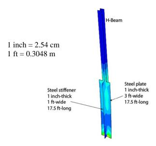
Figure 20: Alternative: Steel Plate with Stiffener
