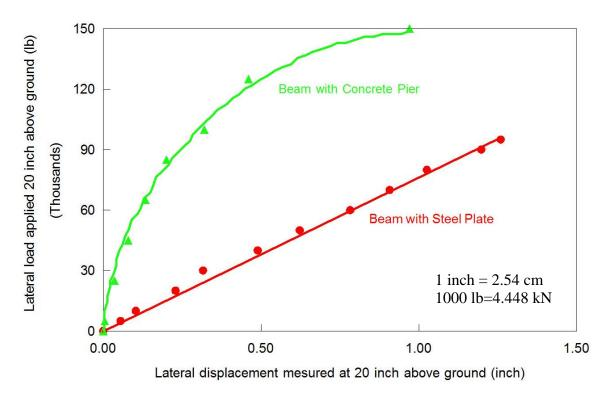
Figure 49: Comparison Between Pile with Concrete Pier and Pile with Steel Plate
