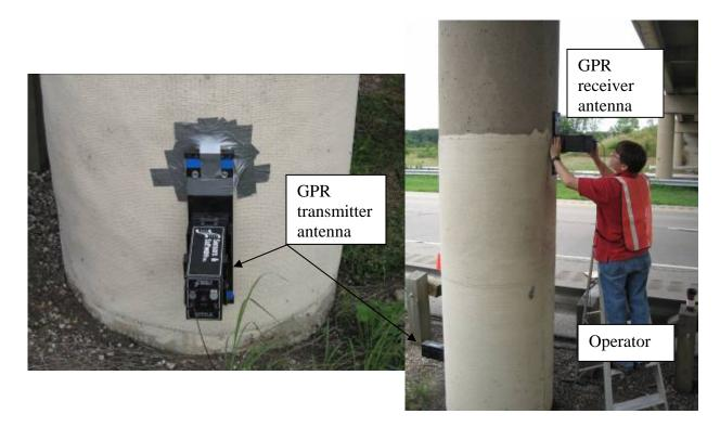
Figure 4.21: GPR testing setup and data collection on a fiberglass wrapped column.
