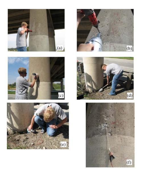
Figure 4.27: Half-cell potential and Cl<sup>-</sup> content data and sample collection: (a) Concrete column drilling. (b) Concrete powder collection for Cl<sup>-</sup> content estimation. (c) Half-cell potential measurements. (d) Access to the concrete column below the fiberglass wrap. (e) Half-cell potential measurements below the fiberglass wrap. (f) Electrode connection to steel rebar.
