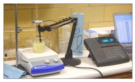
Figure 2.7: Testing set-up for measuring chloride ion content.
