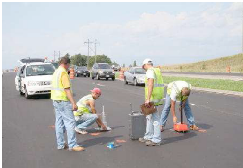
Investigators measured pavement density and air and water permeability between roller passes to compare these properties at different pavement temperatures.
