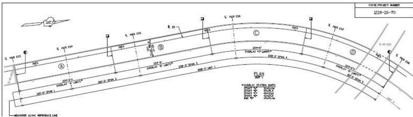
Figure 32. Four different thin polymer overlay test sections (A, B, C, and D) on the Marquette Interchange ramp (from WisDOT).
