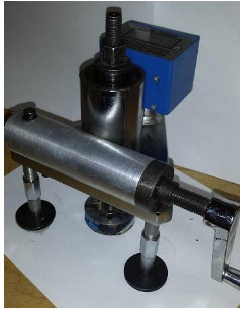
Figure 25. Pull-out test device.
