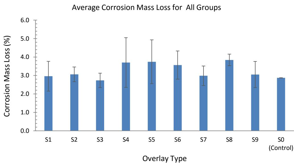
Figure 46. Average corrosion mass loss for all groups.
