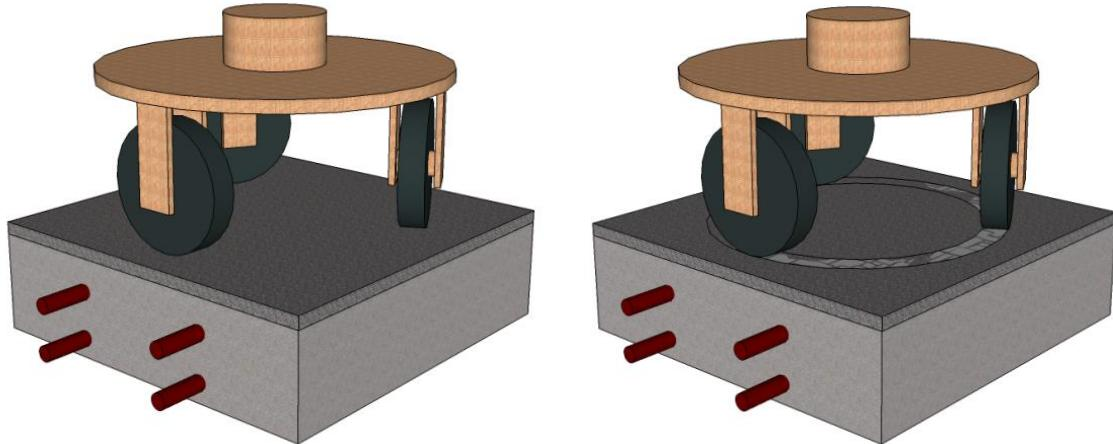
Figure 16. UWM-designed wear test device (conceptual drawing).
