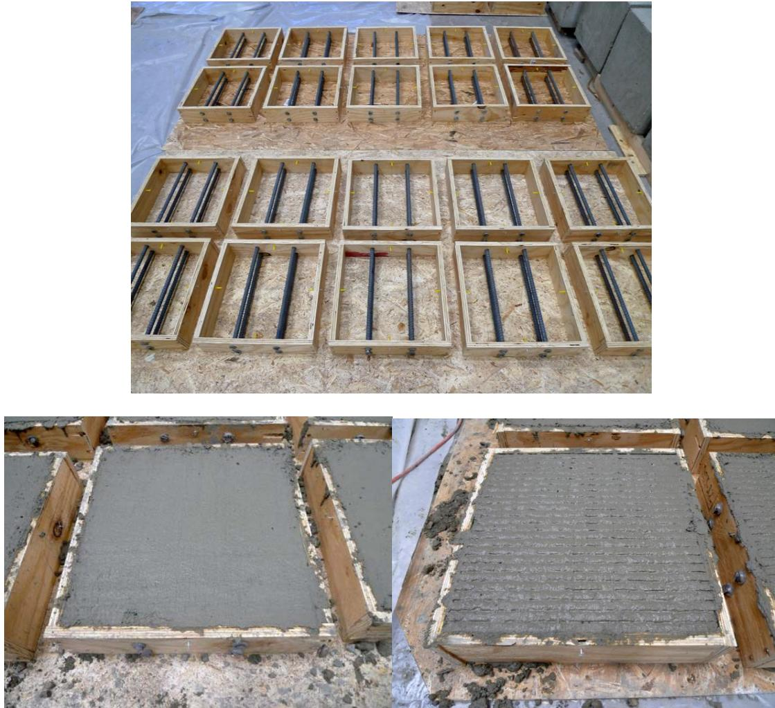
Figure 2. Concrete specimen preparation.
