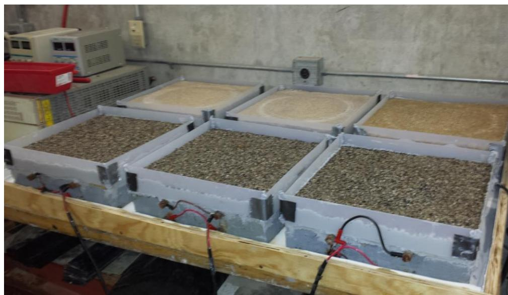
Figure 8. Accelerated corrosion setup.
