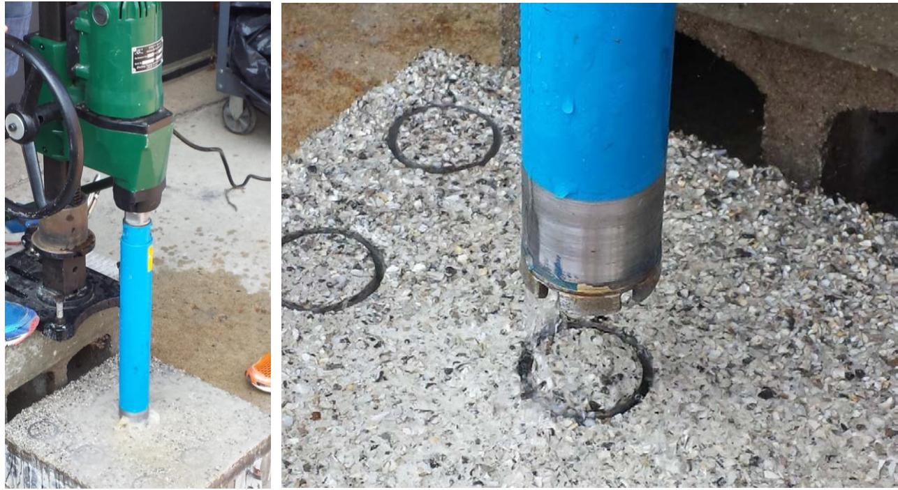
Figure 23. Coring drill setup.
