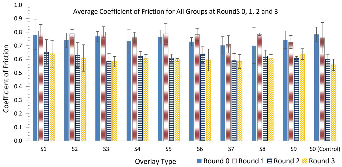
Figure 44. Average coefficient of friction for all groups at round 0, 1, 2, and 3.
