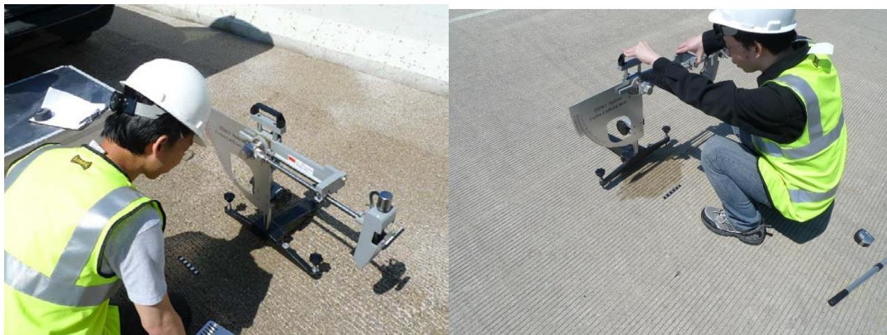
Figure 29. Friction testing using BPT.
