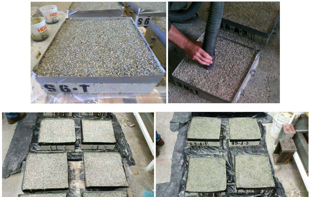
Figure 5. Multi-lift overlay placements.
