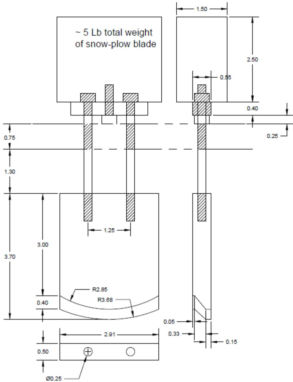
Figure 18. Dimension of the “snow plow” using in Round 3 wear test.
