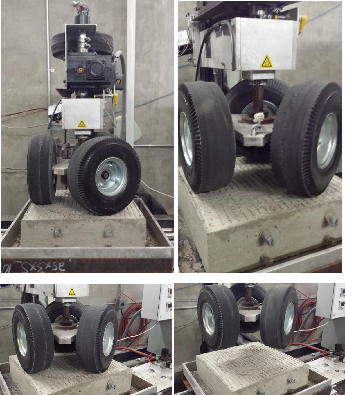
Figure 17. UWM-designed wear test device.
