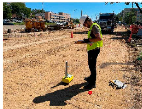
In-place density and moisture content test by nuclear density gauge (NDG) in Dane County (left) and St. Croix County (right)
