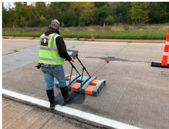
MIT-DOWEL-SCAN testing in Chippewa County
