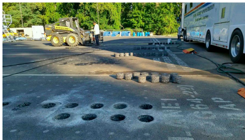
Field Cores recovered from FHWA Accelerated Loading Facility for asphalt mixture and binder testing
