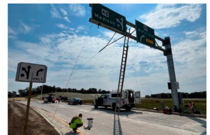
Static tests for torsional upstream and torsional downstream forces
