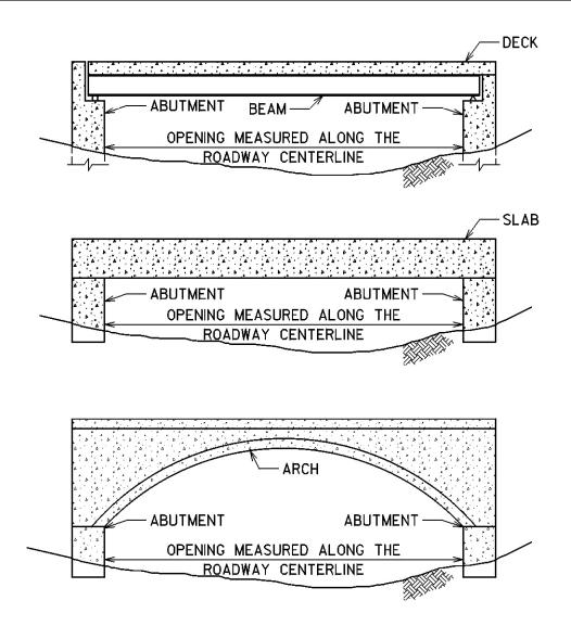
Figure 1.2.2.1-1: Measurement for Definition of a Bridge.
