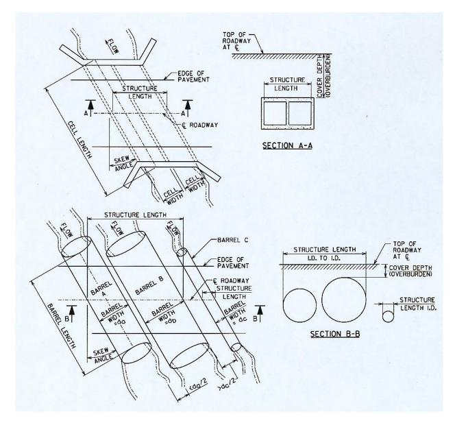
**Figure 1.2.2.1-2:** Measurement for Definition of a Culvert Structure.
