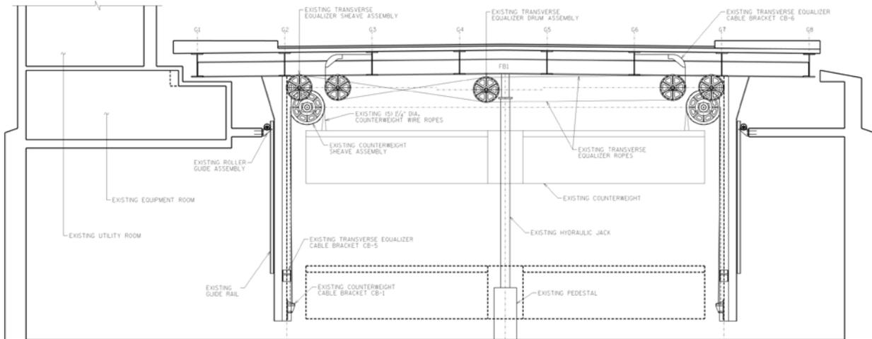
**Figure 3.3.5.1-2:** Elevation view of previous Wisconsin Avenue Bridge lifting and equalizing components. Note only single hydraulic piston used to lift superstructure.
