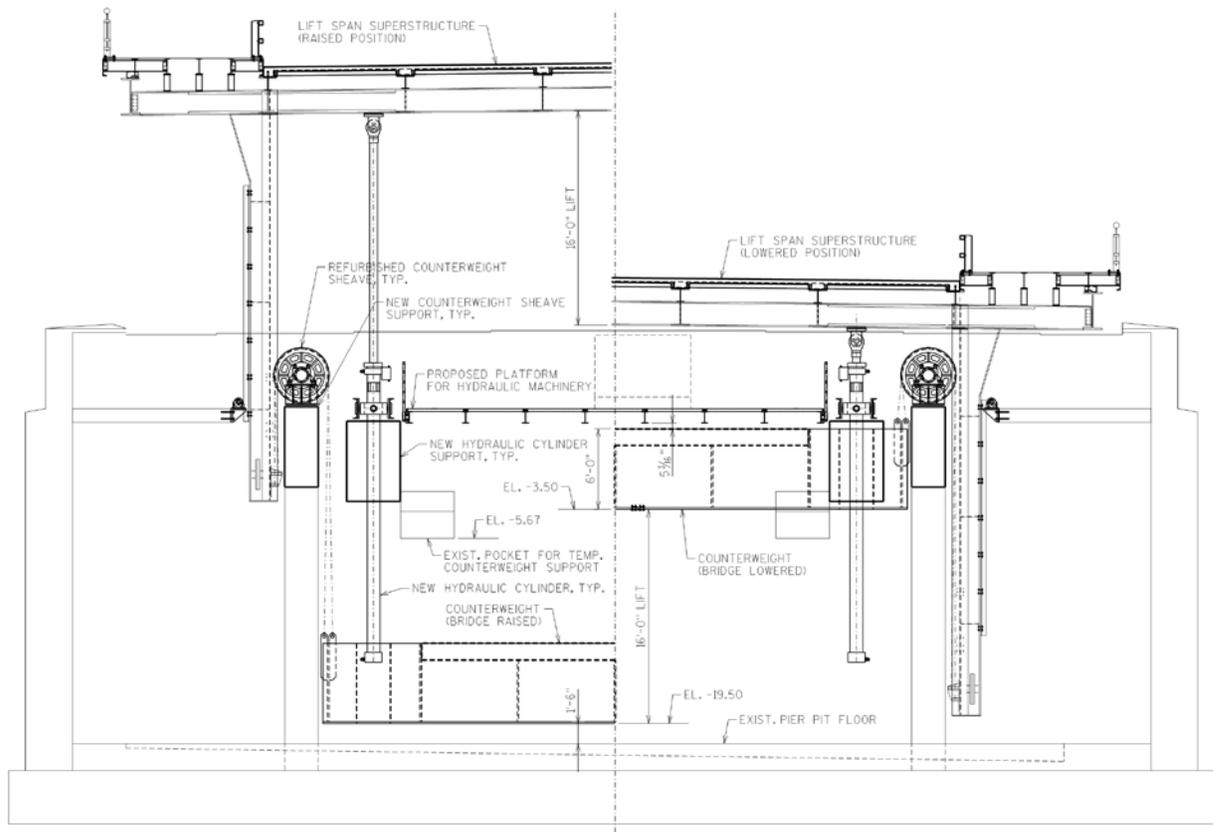
**Figure 3.3.5.1- 3:** Elevation view of rehabbed Wisconsin Avenue Bridge lifting components. Note two hydraulic pistons used to lift superstructure and absence of equalizing cables.
