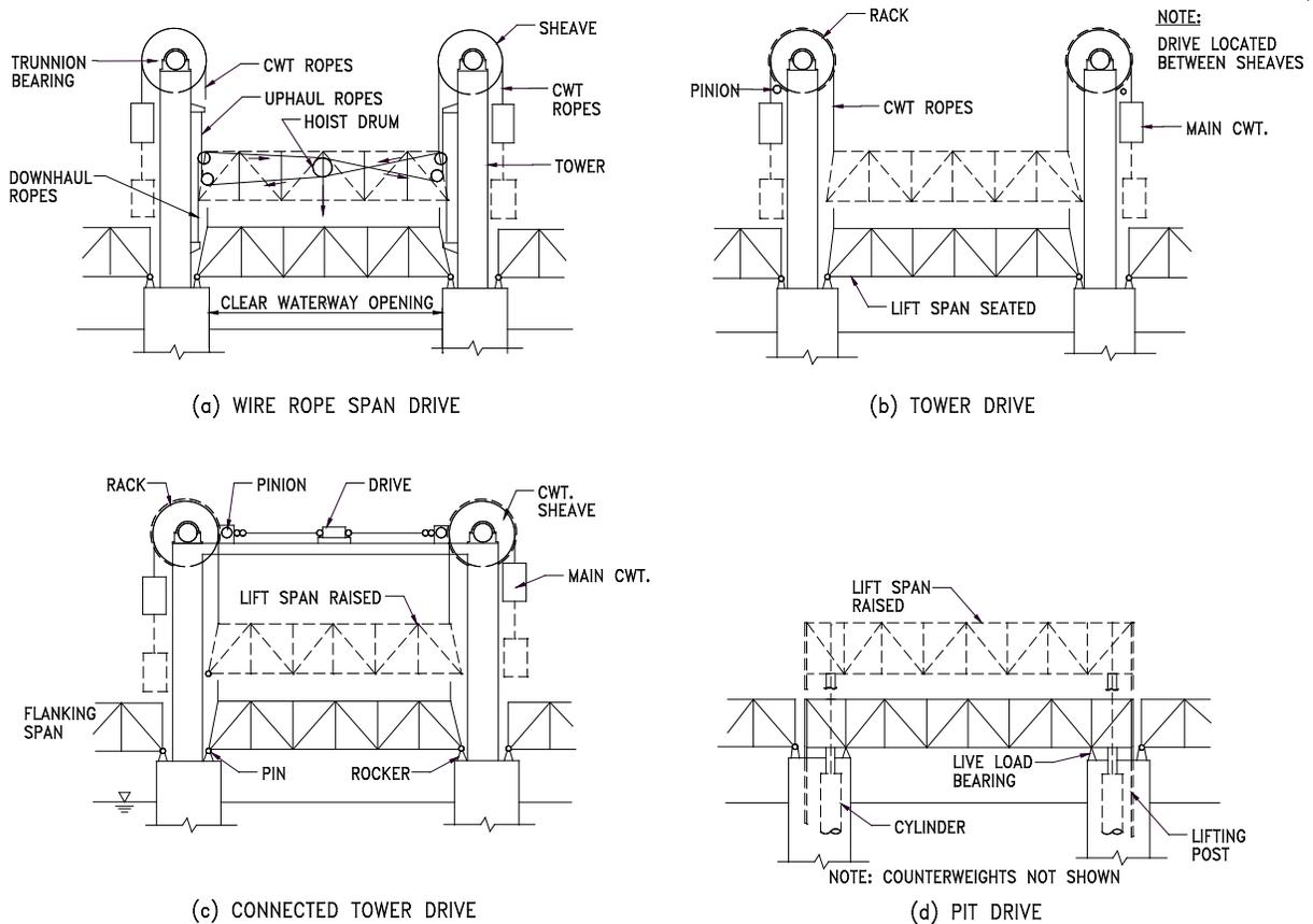
Figure 3.3.1-1: Types of Vertical Lift Bridges.
