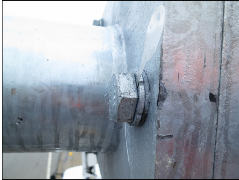
Figure 4.2.2-11: Non-Refusal of Feeler Gauge at DTI Installation.
