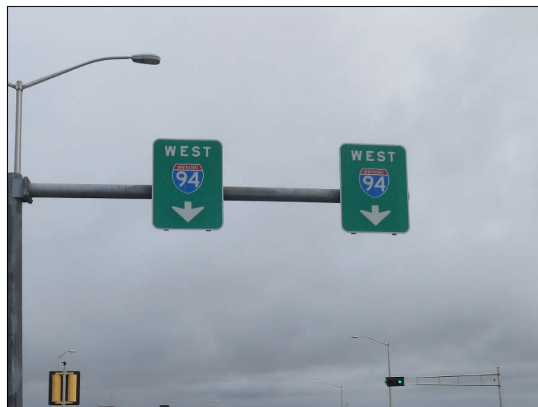
Figure 4.2.3-41: Typical Type II Reflective Sign Panel.
