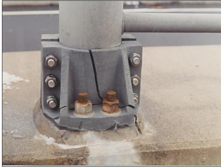
Figure 4.2.3-16: Failed Aluminum Base Casting Clamp Initiated by Over-tightening the Stainless Steel Horizontal Column Bolts.
