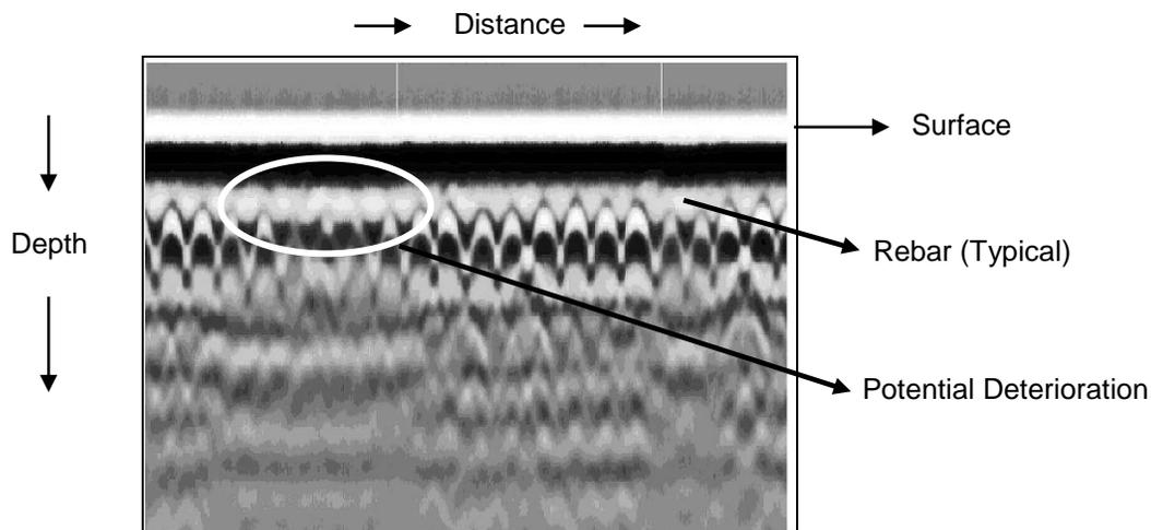
**Figure 5.10.1-1:** Typical Radar Output Image with Notations.
