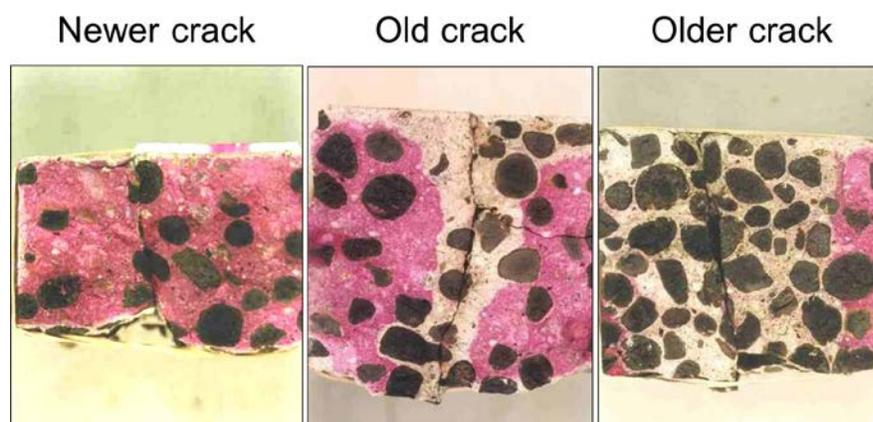
**Figure 5.17.1- 1:** Image of Cracked Concrete Samples After Carbonation Testing. Note the Older Crack and the Amount of Carbonation in the Concrete.
