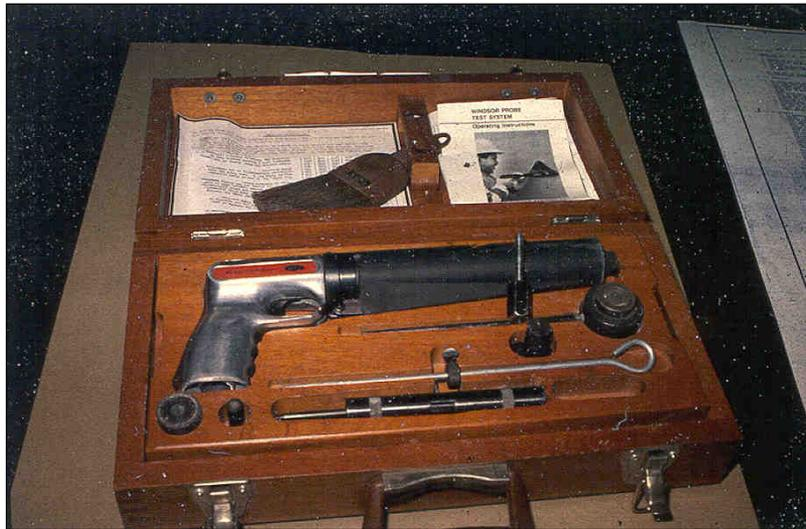
Figure 5.19.1-1: Windsor Probe Test Kit.
