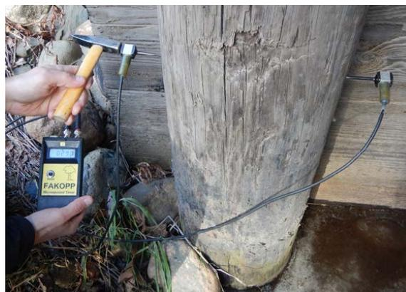
**Figure 5.21.2-2:** Stress Wave Timer using impact hammer
