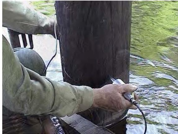
**Figure 5.21.2-3:** Stress Wave Timer using automated pulses.
