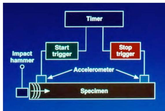
**Figure 5.21.2-1:** Schematic of a Stress Waver Timer
