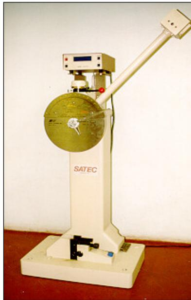
**Figure 5.23.5-1:** Charpy Impact Testing Machine.
