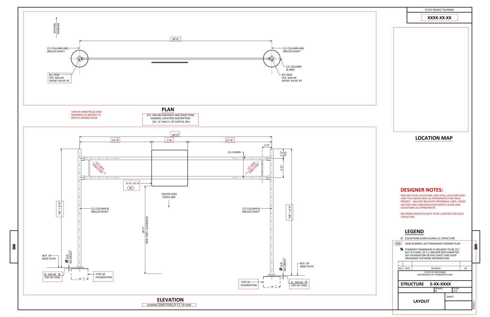
DESIGNED ACCORDING TO THE AASHTO "LRFD SPECIFICATIONS FOR STRUCTURAL SUPPORTS FOR HIGHWAY SIGNS, LUMINAIRES AND TRAFFIC SIGNALS", 1ST EDITION AND INTERIM SPECIFICATIONS, AND THE WISDOT BRIDGE MANUAL.
