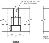
POCKET CAN BE CHAMFERED WITH SKEW
