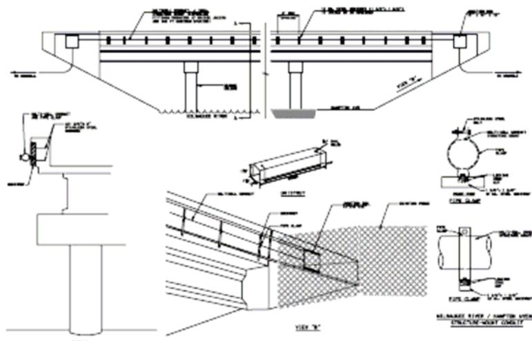
**Figure 50.3-4: Bridge-specific Structure Mount Conduit Detail Example**
